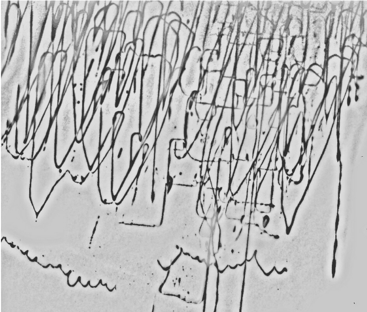
Figure 10.1. Example of dislocation structures responsible for plastic deformation in a quartz foil. The width of the transmission electron microscope image is approximately 5\ \mu\text{m} . Clear screw dislocations are seen at the bottom of the image in contrast to the dominantly edge dislocations above. [Courtesy of J. Fitz Gerald.]
