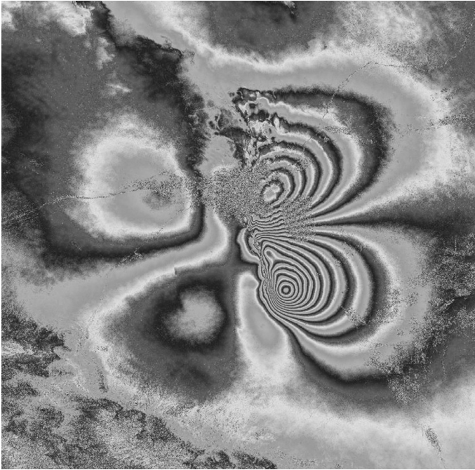
Figure 11.24. ENVISAT interferogram of the Bam earthquake in Iran, 2003 December 26, Mw 6.6; the InSAR analysis was carried out using DORIS software. Each interferometric fringe represents 28.1 mm of line-of-sight deformation. The fault is predominantly strike-slip, with a peak slip of around 2 m. The elastic deformation cannot be explained by slip on a single planar fault (Funning et al., 2005). The areas of low coherence in the centre of the image are the heavily damaged Iranian cities of Bam and Bavarat. ENVISAT SAR data were made available through the European Space Agency (ESA). [Courtesy of J. Dawson.]
