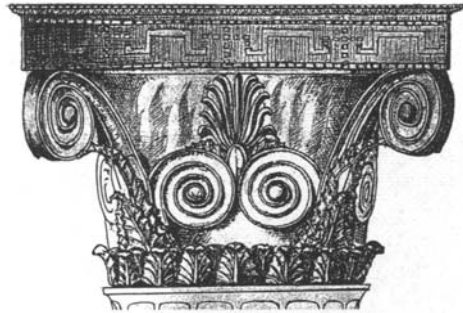
Fig. 16. Corinthian capital from the temple of Apollo Epicurius at Bassae, restored. (After D. Watschitzky, JÖAI 37 (1948) 53, fig. 5.)
