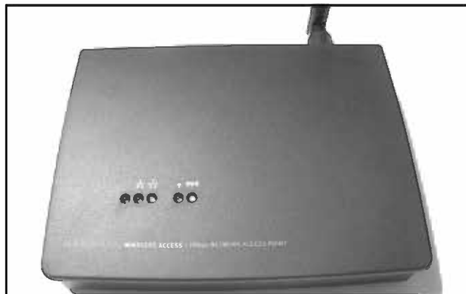
Figure 10.13 The USR 2450 Access Point before Modification
