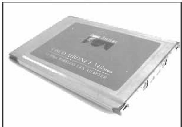
Figure 10.2 A Cisco Card with Dual MMCX Connectors
