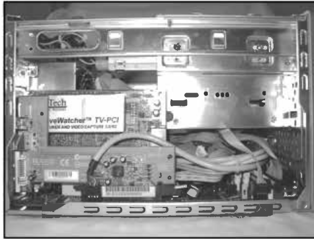
Figure 6.31 The Two Cards Installed in the Shuttle Case
