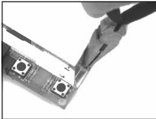
Figure 7.44 Removing the RF Shield
