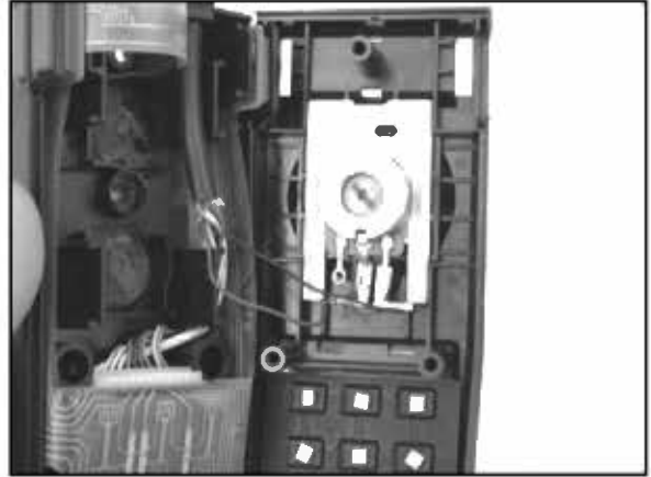
Figure 8.30 Inside the 5200 Paddle Controller
