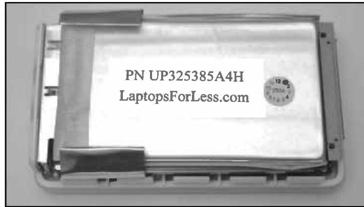
Figure 11.21 Affixing the Battery to the Hard Drive
