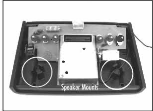
Figure 7.23 Receptacles Inside the Case for Speakers
