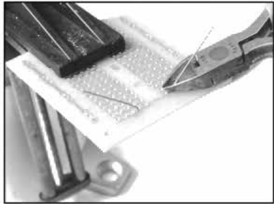
Figure 2.31 Snipping Off the Remaining Component Lead
