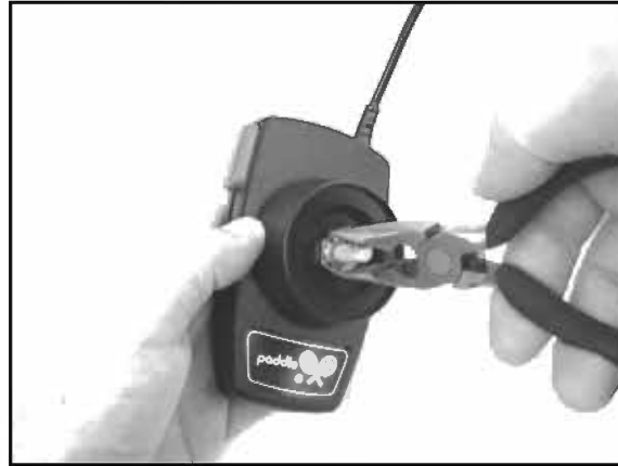
Figure 8.17 Removing the Paddle Nut
