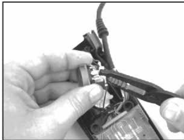
Figure 8.24 Removing Wires from the Upper 5200 Pot
