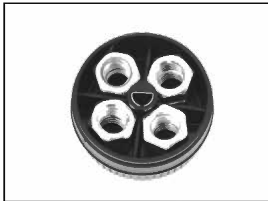
Figure 8.33 Weighing Down the Dial with Hex Nuts
