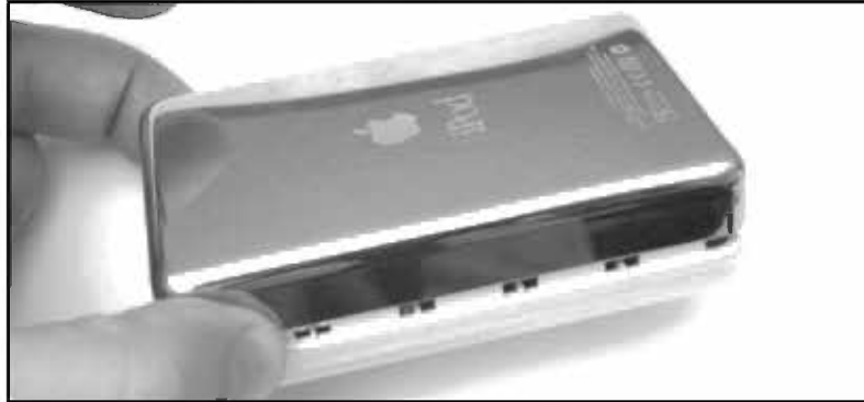
Figure 11.23 Reattaching the Metal Half of the Case
