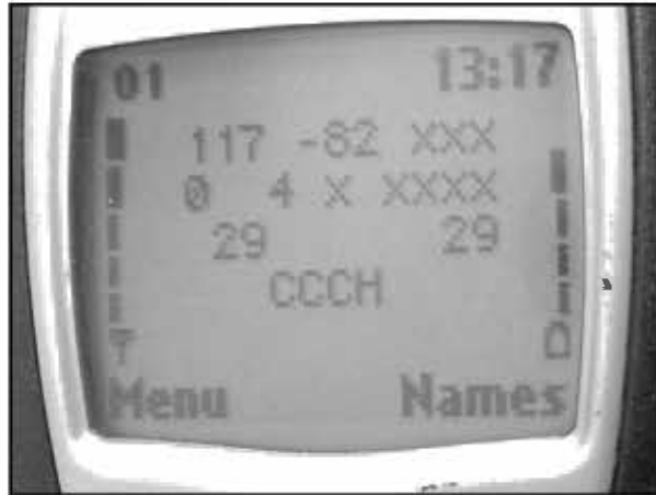
Figure 12.29 Test 01: Showing the Phone's GSM Parameters
