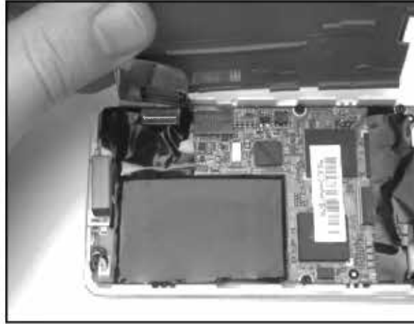
Figure 11.33 Reattaching the Hard Drive
