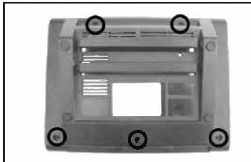
Figure 7.37 Remove Screws as Shown
