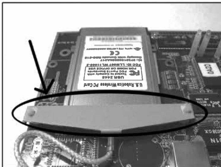
Figure 10.15 Before Removing the Card ... See the Metal Brace?
