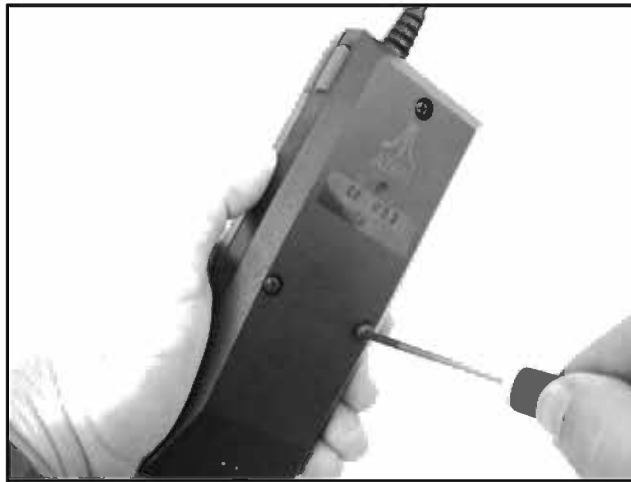
Figure 8.20 Remove the Three Screws from the Back of the 5200 Controller
