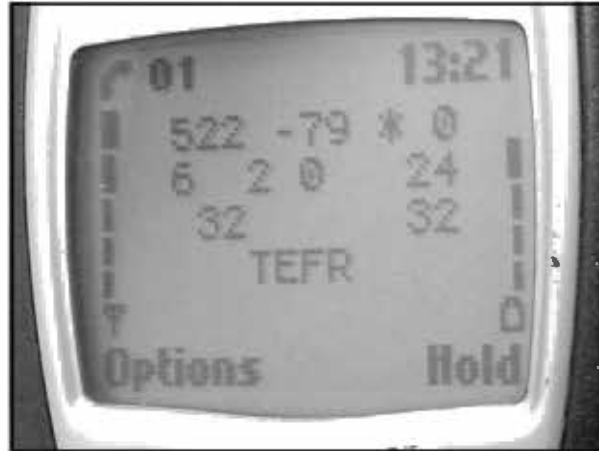
Figure 12.30 Test 01: Information Displayed When the Phone Is Engaged in a Call
