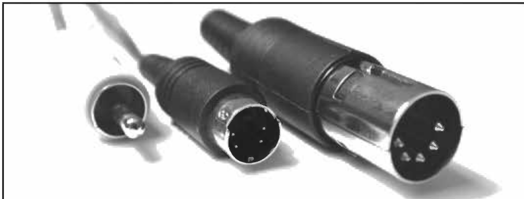
Figure 8.56 Composite, S-Video, and Atari 8-Bit Monitor Connectors (Left to Right)
