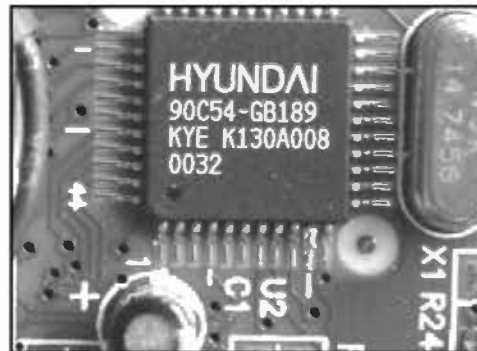
Figure 3.34 Hack Complete: Pin 10 of Microprocessor Lifted (Close-Up)
