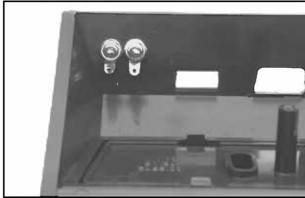
Figure 7.31 RCA Jacks Attached
