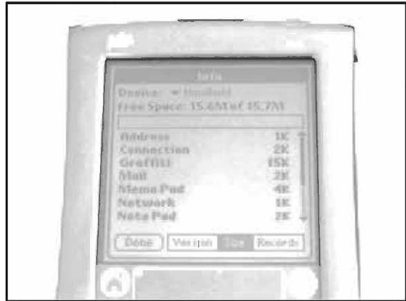
Figure 13.42 After Hack: Palm m505 With 16MB RAM
