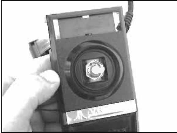
Figure 8.29 Assembling the 2600 Potentiometer
