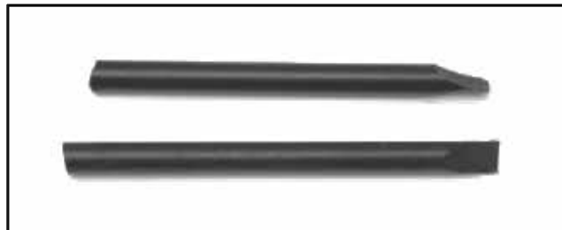
Figure 11.5 Plastic Wedges for Opening an iPod
