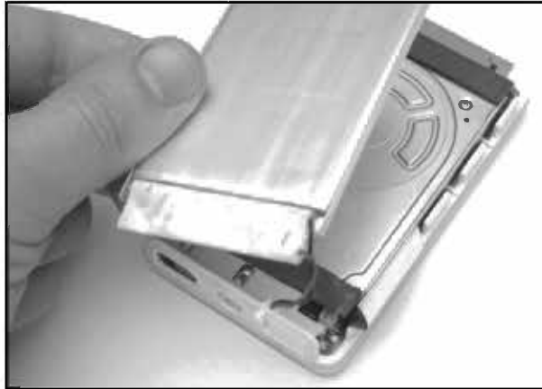
Figure 11.19 Removing the Old Battery
