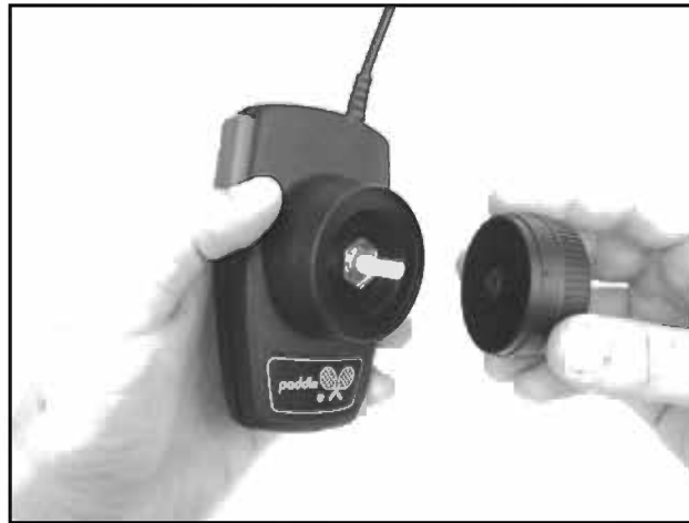
Figure 8.16 Removing the Paddle Dial
