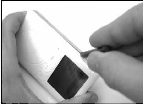
Figure 11.10 Prying into the Case
