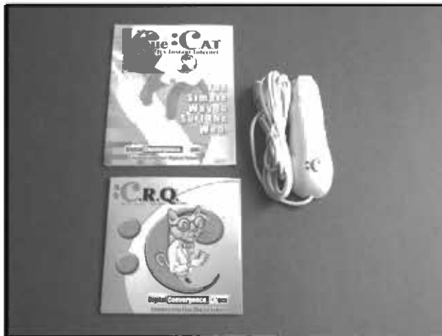
Figure 3.1 The CueCat Optical Reader, Four-Screw PS/2 Interface with Original Materials
