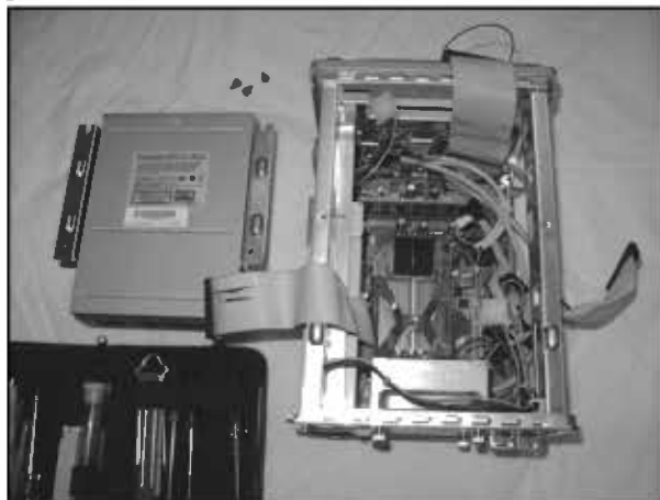
Figure 6.27 Removing Parts from the Shuttle Case
