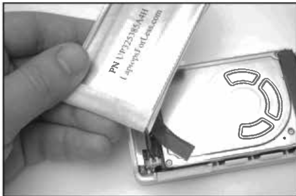
Figure 11.20 Connecting the New Battery
