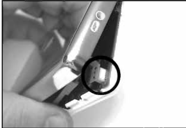
Figure 11.14 Connector Holding Two Halves Together
