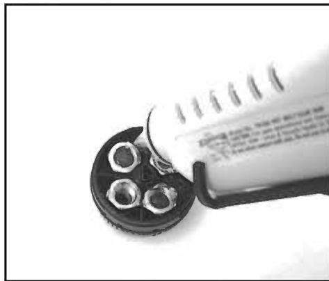
Figure 8.34 Gluing the Nuts in Place
