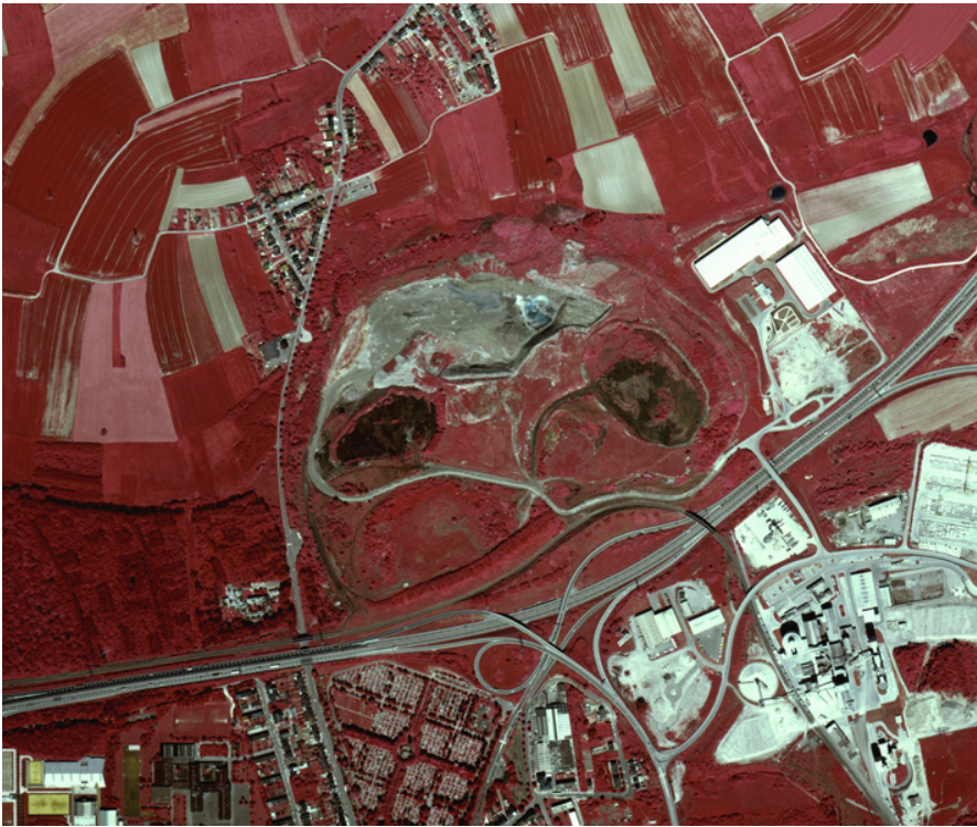
Fig. 3.1-20: CIR aerial photograph of an industrial plant (lower right corner) and its waste disposal site (in the center) near the city of Esch-sur-Alzette in Luxembourg. The photo was taken on May 27, 1999, at a scale of 1 : 15 000 by Hansa Luftbild (German Air Survey), Münster
