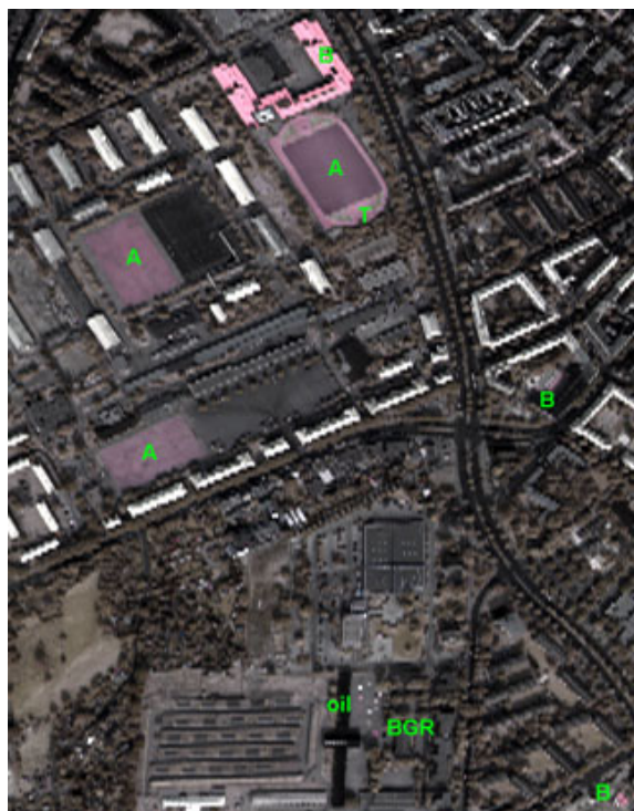
Fig. 3.3-10: Processed HyMap image showing materials containing hydrocarbon at the ground surface in Spandau, Berlin (BGR premises and oil-contaminated reference areas; A, artificial turf; T, race track; B, plastic roofs)
