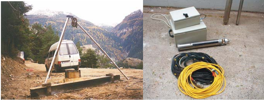
Fig. 4.6-25: VSP equipment, left: tripod with cable and registration car, right: geophone chain (black cable), 3-component borehole tool (metallic rod) and seismograph
