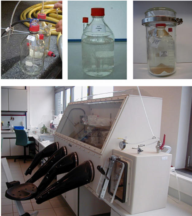
Fig. 5.3-47: Anaerobic treatment of groundwater microcosms; top left : filling of 2-L bottles with groundwater in the field; top middle : microcosm in the laboratory; top right : anaerobic incubation in an anaerobic vessel equipped with an oxygen-consuming reagent; bottom : anaerobic chamber for the anaerobic handling of microcosms
