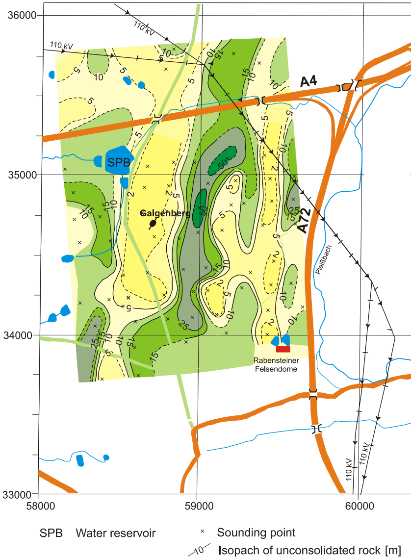
Fig. 6.2-16: Planned waste disposal site at Rabenstein near Chemnitz, Germany: Thickness of the unconsolidated cover rocks according to the results of the geoelectric depth soundings (VES) and mapping, Geophysik GGD 1993, commissioned by BGR
