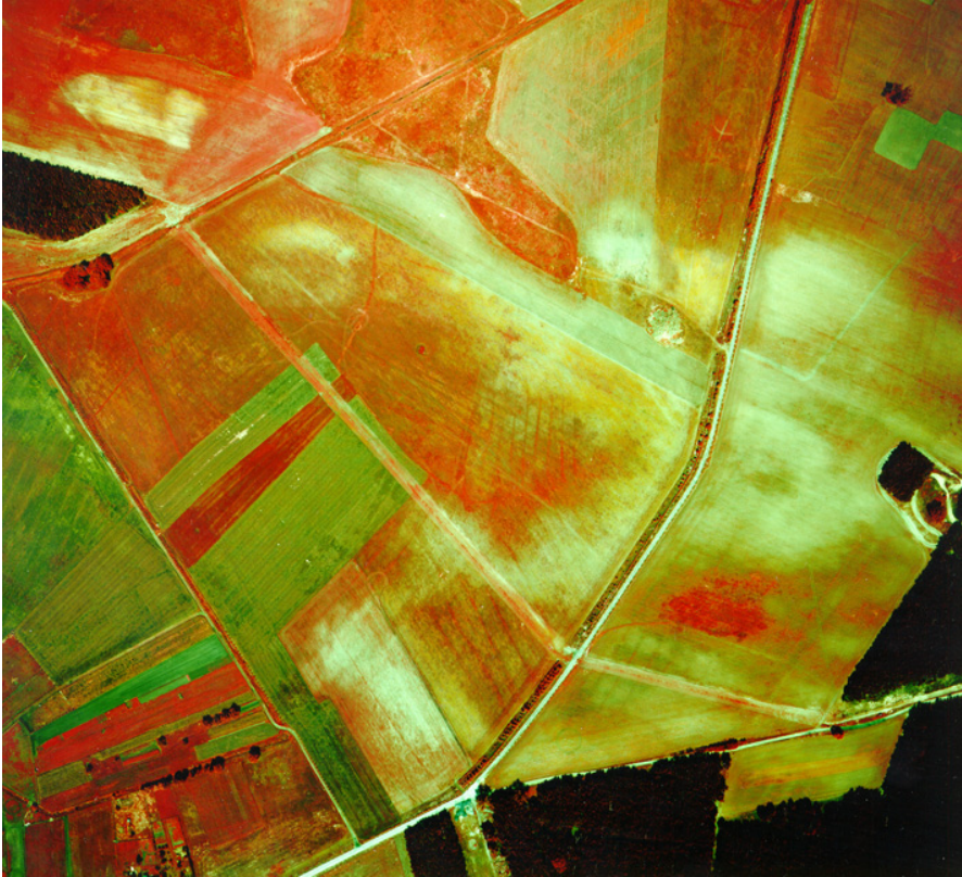
Fig. 3.1-12: CIR aerial photograph taken on July 3, 1993, of an area west of the Schöneiche waste disposal site. Extensive sandy soil substrates responsible for impaired plant growth can be recognized by the lighter colors, (Aerial photograph: WIB GmbH for BGR).
