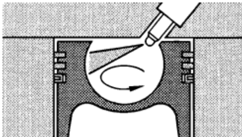
Combustion-chamber shape and nozzle location in the MAN M system
