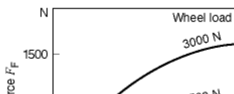
Cornering force as a function of wheel-slip angle
