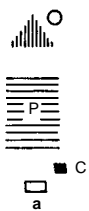
27.35 Bad organ arrangement. Key: o organ, c organ console, p people, ch choir, m, minister, a altar
