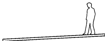
6.8 Walking along a longitudinal slope: up to 3 per cent preferred, generally 5 per cent maximum, 5-10 per cent possible depending on climate. Between 5 per cent and 8 per cent slopes are considered to be ramps
