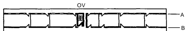
42.35 Common escape routes in balcony/deck approach single-stair buildings with an alternative exit from each dwelling. One of the external enclosures A or B must be fire resisting
