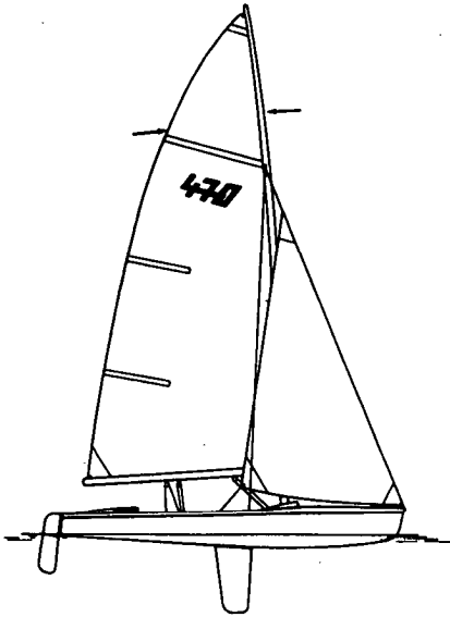
23.6 470: an Olympic boat. L/b/d/m/s = 4.7/1.68/0.97/120 \text{ min}/9 \text{ main}, 3.7 \text{ jib}, 13 \text{ spinnaker}
