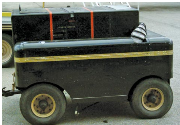
Figure 11-30. A portable compressed air cart.
