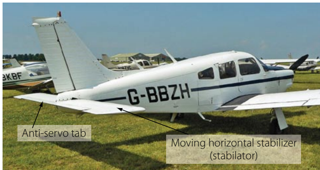
Figure 3-66. Moving horizontal stabilizer, known as a stabilator, on a Piper Cherokee Arrow provides pitch control.
