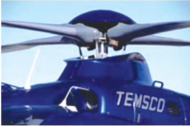
Figure 3-85. Eurocopter Model 135 rigid rotor system.
