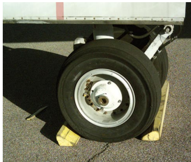
Figure 11-12. Wheels chocked fore and aft.
