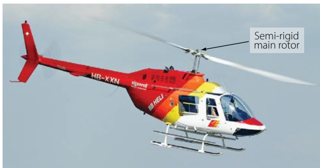
Figure 3-84. Bell Jet Ranger with semi-rigid main rotor.
