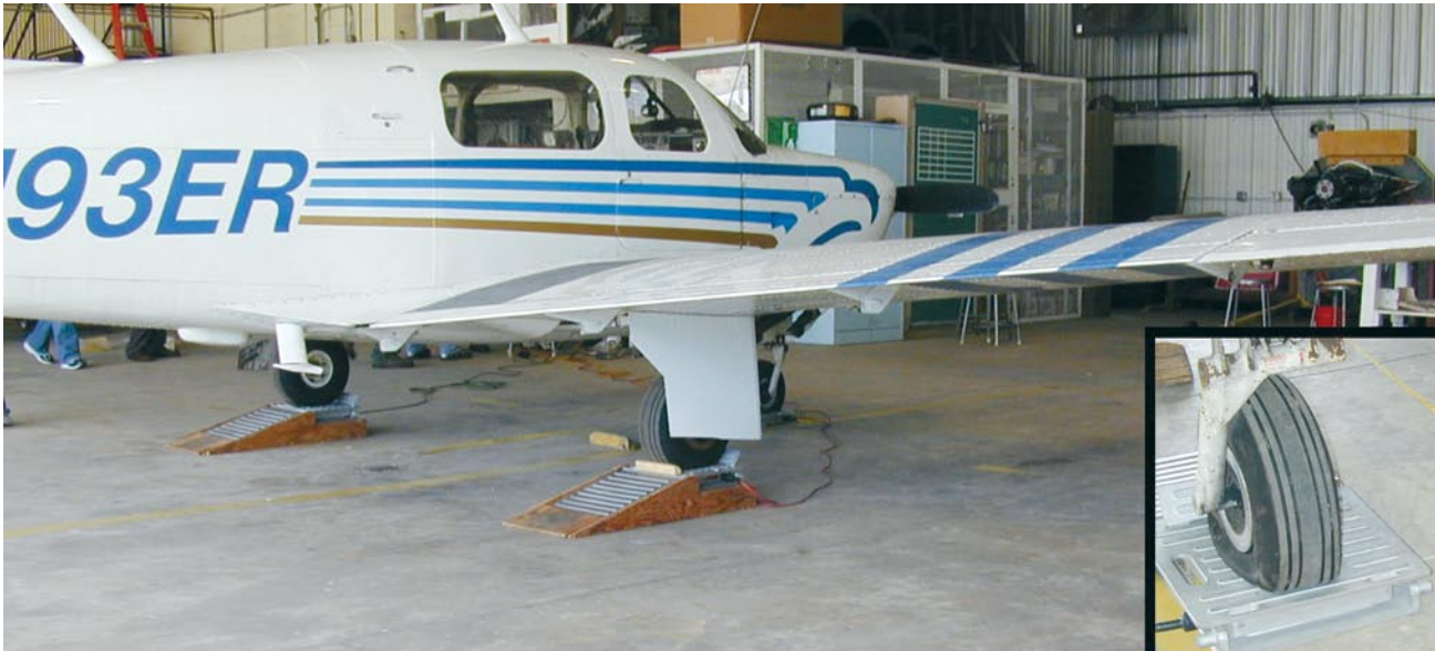
Figure 4-13. Mooney M20 being weighed with portable electronic platform scales.
