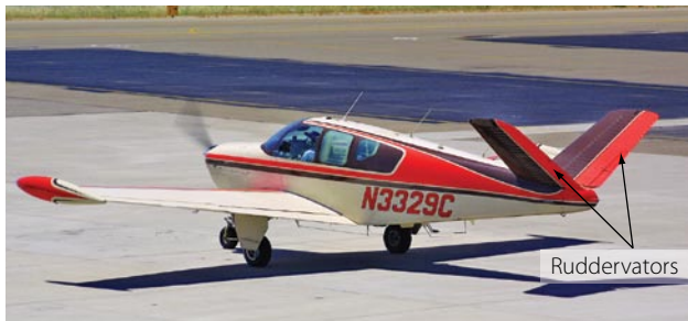
Figure 3-67. Ruddervators on a Beechcraft Bonanza provide pitch control.
