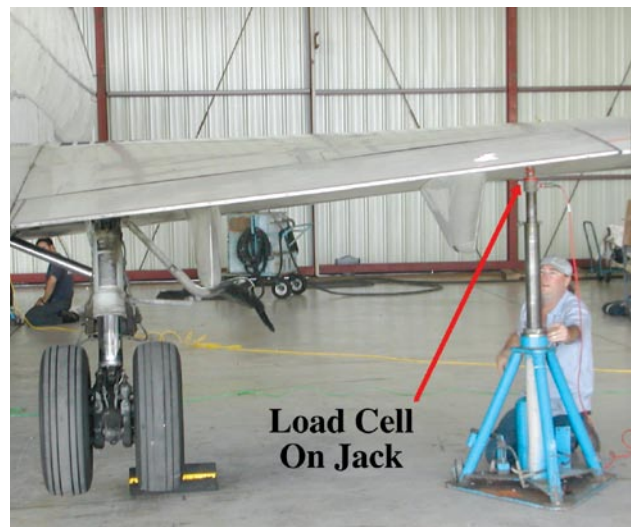
Figure 4-15. Airplane on jacks with load cells in use.
