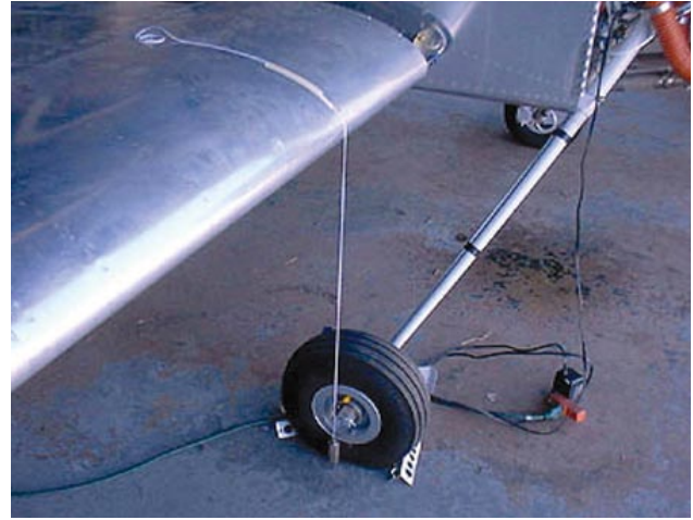
Figure 4-17. Plumb bob dropped from a wing leading edge.
