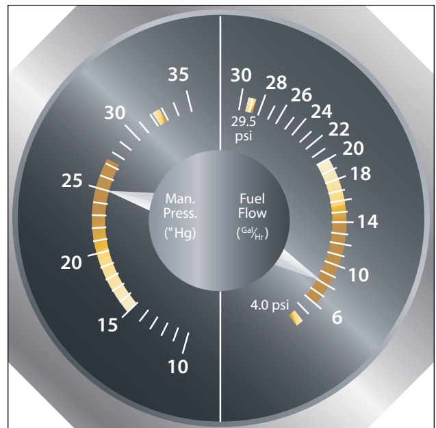
Figure 3-35. Manifold pressure gauge indicating absolute pressure.
