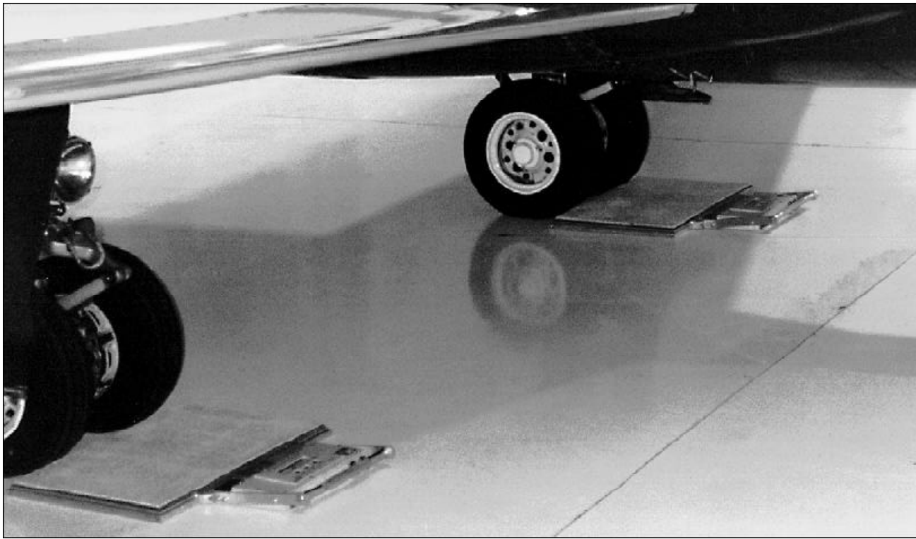
Figure 3-1. Low profile platform scales are used to weigh some aircraft. One scale is placed under each wheel. (Photo courtesy General Electrodynamics Corp.)
