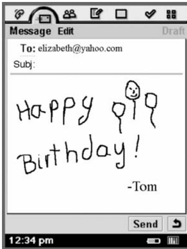
FIGURE 26.43 Example of ink messaging application for mobile devices. Users can draw or write with a stylus on the device screen to compose an e-mail in their own handwriting; no automatic recognition is necessarily involved.
