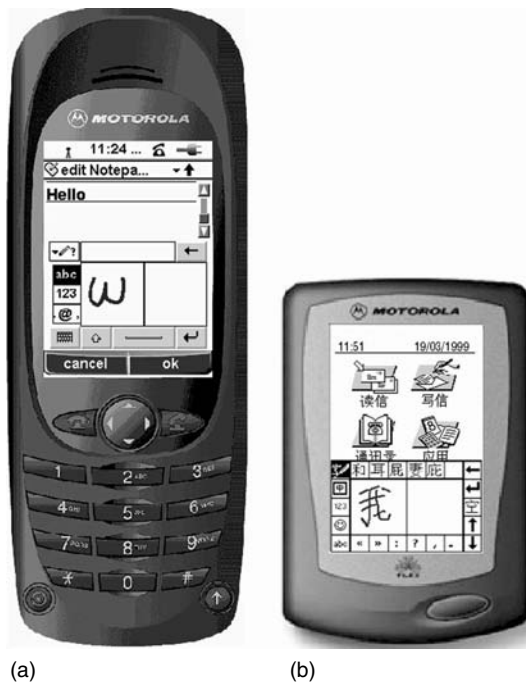
FIGURE 26.37 Character-based text input method on today's mobile devices. In (a), user interface for English character input on a cellular phone. In (b), user interface for Chinese character input on a two-way pager.
