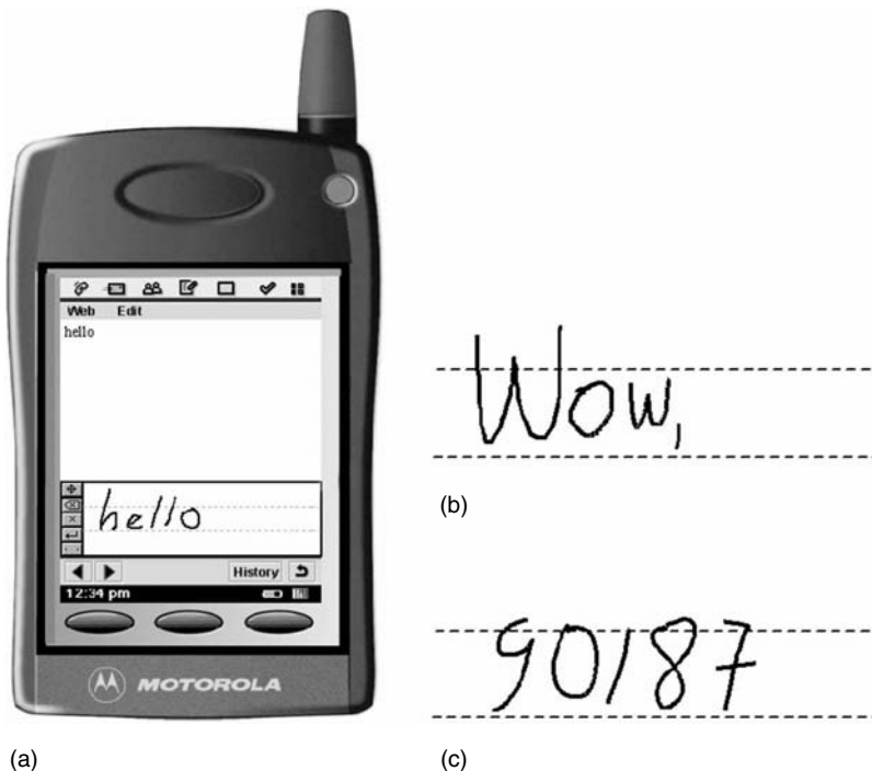
FIGURE 26.38 Word-based text input method for mobile devices. In (a), a user interface prototype. In (b), an image of the mixed-case word Wow, where relative size information can be used for distinguishing among the letters in the Ww pair. In (c), an image of the digit string 90187 where ambiguity in the identity of the first three letters can be resolved after identifying the last two characters as digits.
