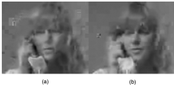
FIGURE 42.34 One frame of Suzie sequence encoded with MPEG-4 at 18 kbit/s and transmitted over a GPRS channel with C/I = 15 dB, with CS-1 and 4 time-slots used: (a) no error resilience and (b) AIR.
