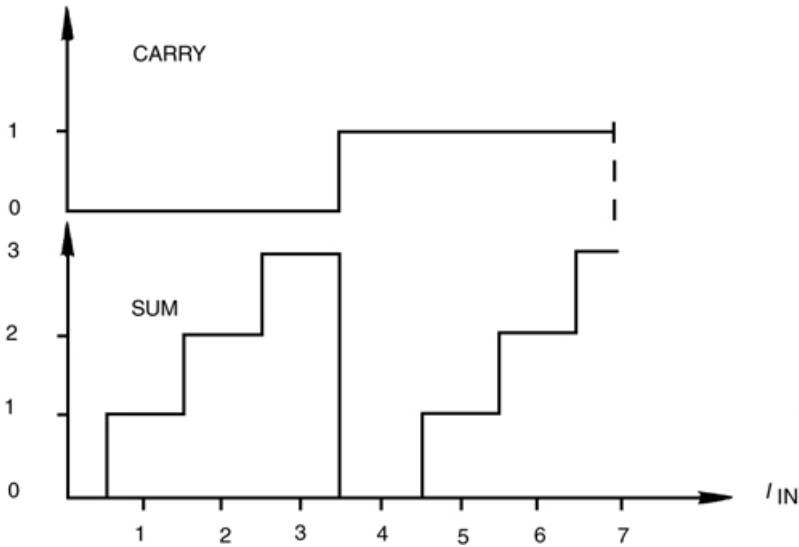
FIGURE 11.6 Current-mode CMOS quaternary threshold logic full adder I/O transfer characteristic.
