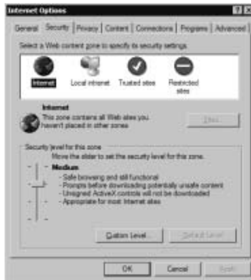
Figure 8.1 Settings on the Security tab in IE's Internet Options define security zones.
