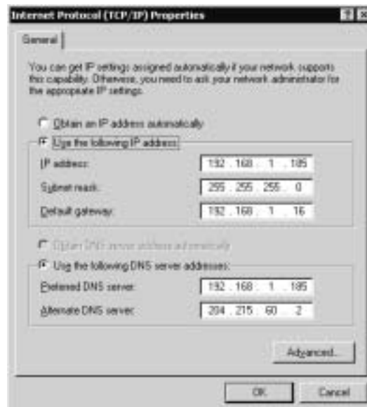
Figure 5.11 Network administrators can manually assign IP addresses (called “static addresses”) to computers.
