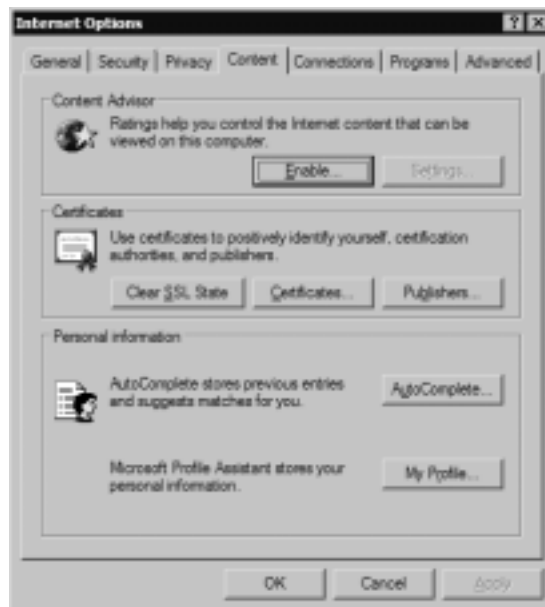
Figure 8.3 You can configure certificate options in IE using the Content tab in Internet Options.
