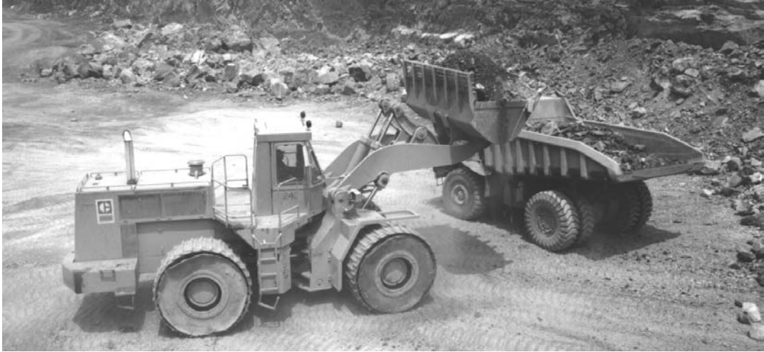
Fig. 13.7 Wheel loader loads off-highway dump truck. (Caterpillar Tractor Co.)
