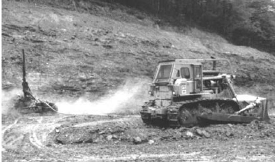
Fig. 13.16 Percussion drill powered by an air compressor and mounted on a tractor. ( Caterpillar Tractor Co. )
