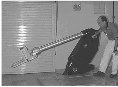
FIGURE 21.13 Force controlled hydraulic manipulator (courtesy Oak Ridge National Laboratory).
