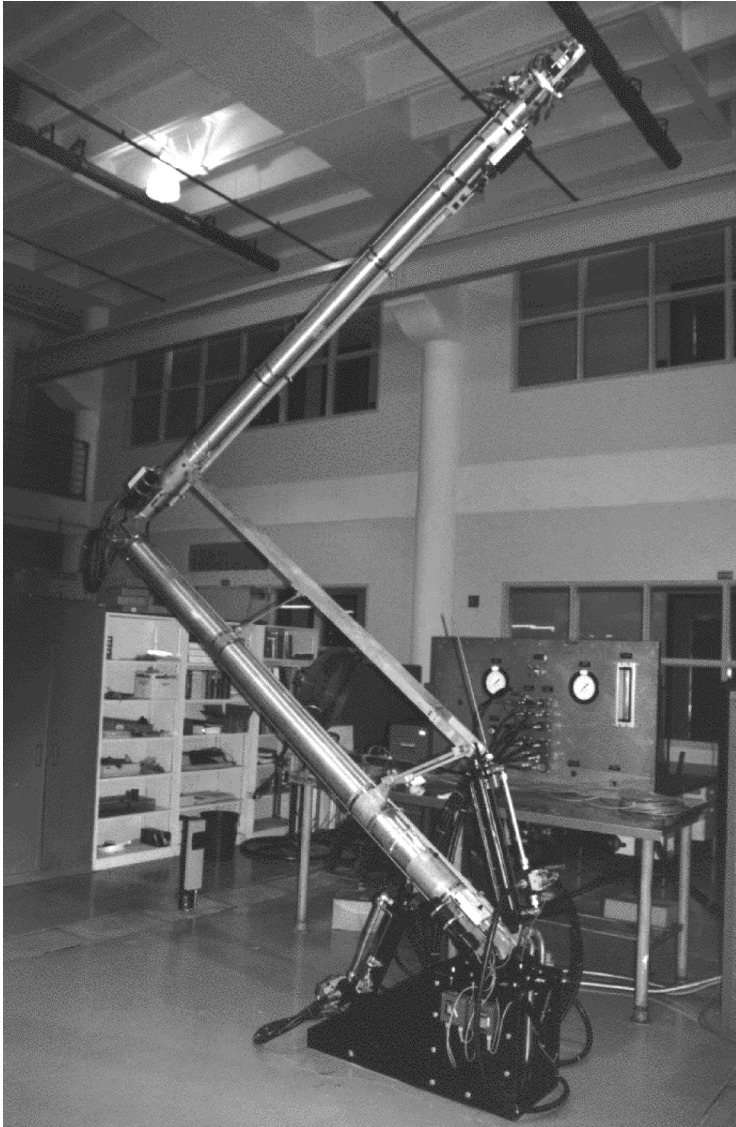
FIGURE 24.6 The experimental arm RALF (Robotic Arm Large and Flexible). (Total length about 6 m, lowest natural frequency about 3 Hz.)
