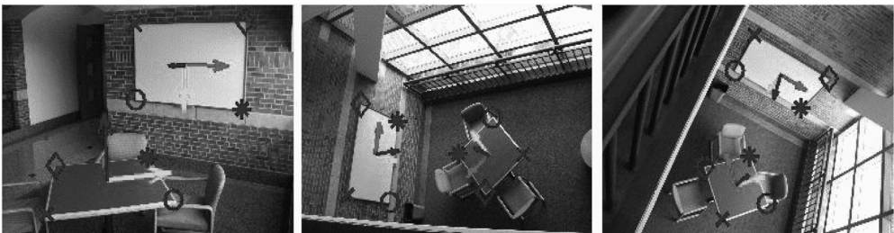
FIGURE 22.12 Two symmetry cells are matched in three images. From the raw images, symmetry cell extraction, to cell matching, the process needs no manual intervention.
