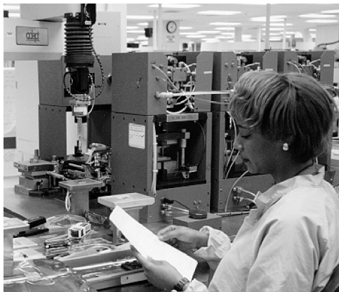
FIGURE 10.10 An automated system for forming the leads on electronic packages.
