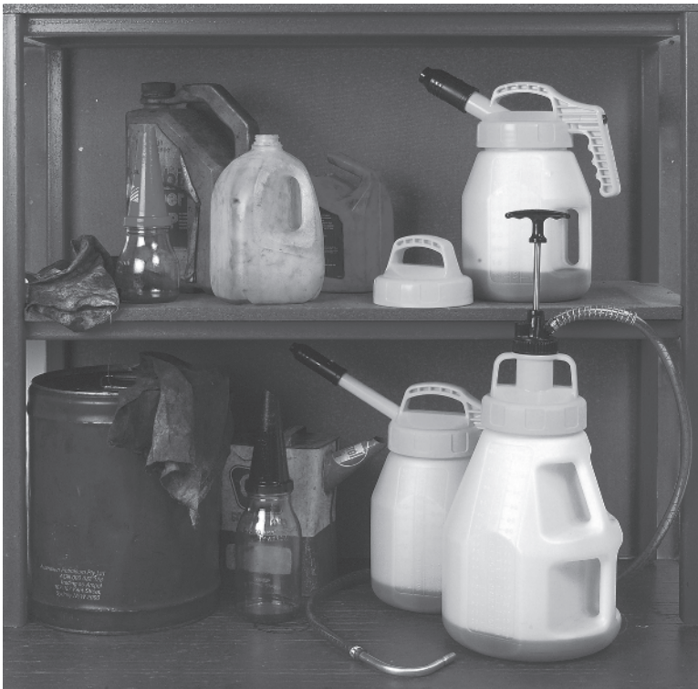
Figure 10-27: Variations of high-grade lube oil transfer containers suit every reasonable requirement (Source: Oil Safe® Systems Pty. Ltd., also Trico Mfg. Company and PdM USA)
