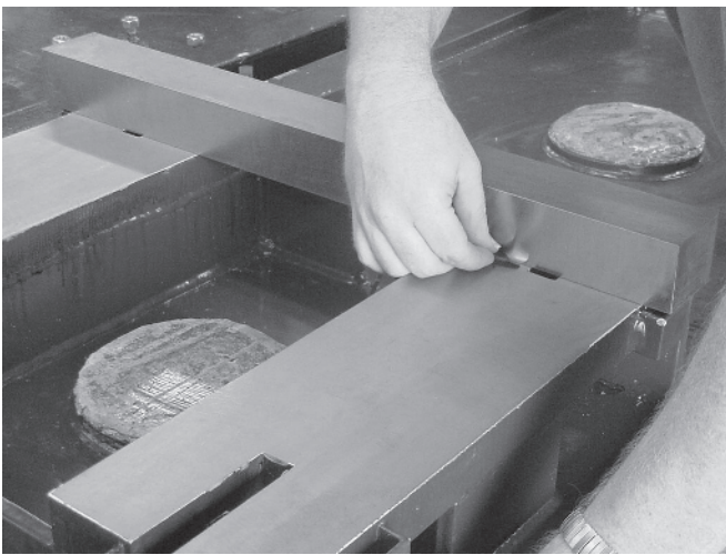
Figure 3-22: Flatness being measured with ground bar stock and feeler gauges
