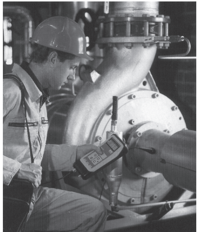
Figure 12-5: SPM data collection on a process pump (Source: SPM Instruments, Inc., Marlborough, Connecticut)
