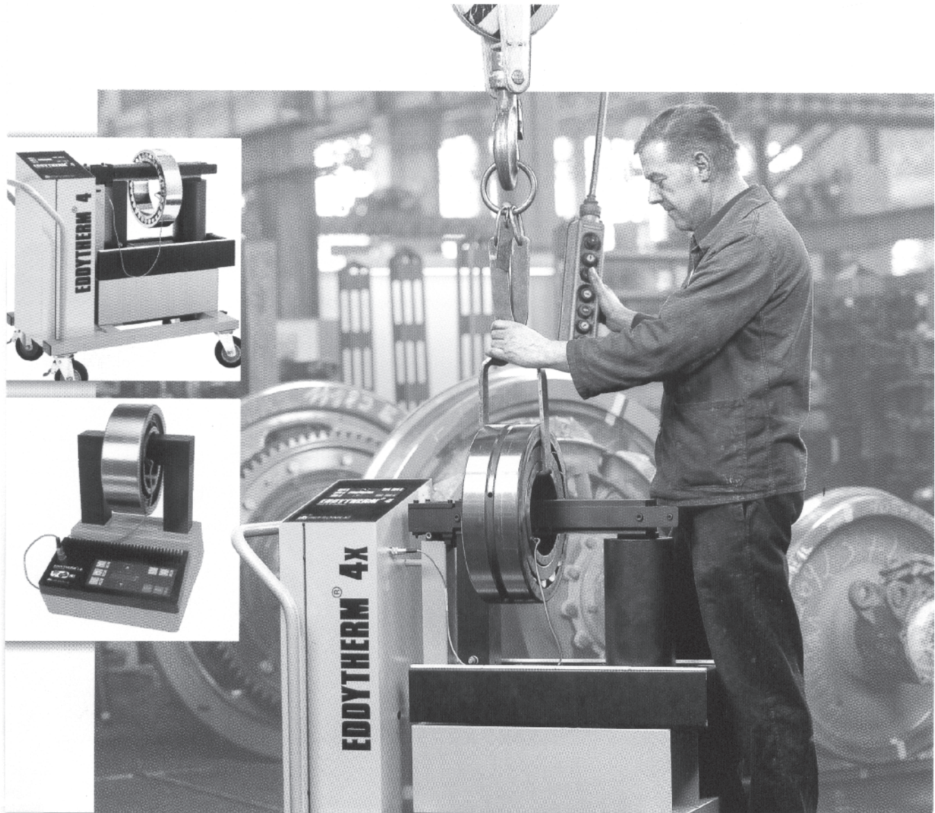
Figure 15-20: Eddy current (induction) heater (Source: Prueftechnik A.G., D-85737 Ismaning, Germany)
