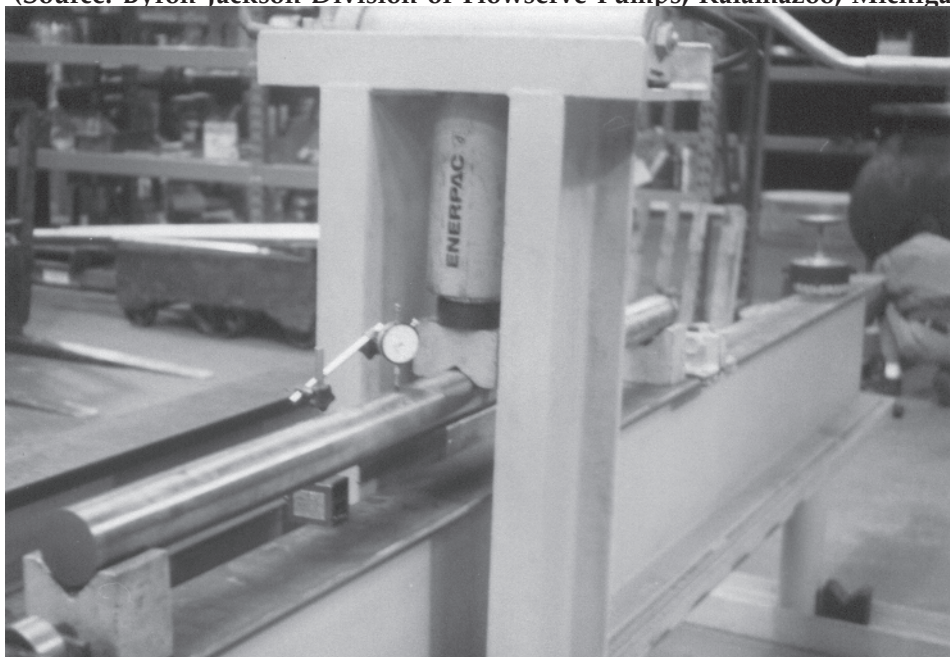
Figure 15-18: Mechanical shaft straightening method (Source: Byron Jackson Division of Flowserve Pumps, Kalamazoo, Michigan)
