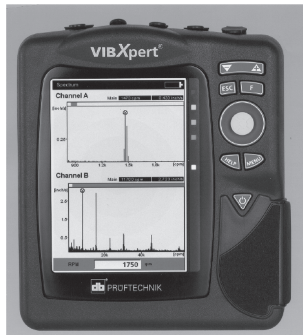
Figure. 12-17: Modern light-weight data collector and vibration analyzer (Source: Prueftechnik, Germany, and Ludeca, Inc., www.ludeca.com )
