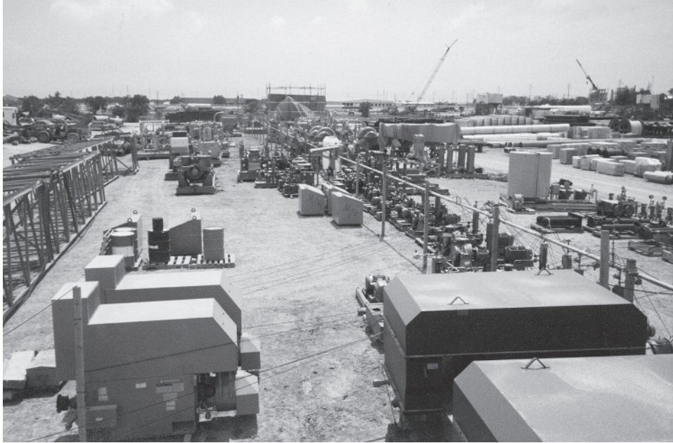
Figure 10-19: Oil mist protected outdoor equipment storage in a hot and humid U.S. Gulf Coast environment.
