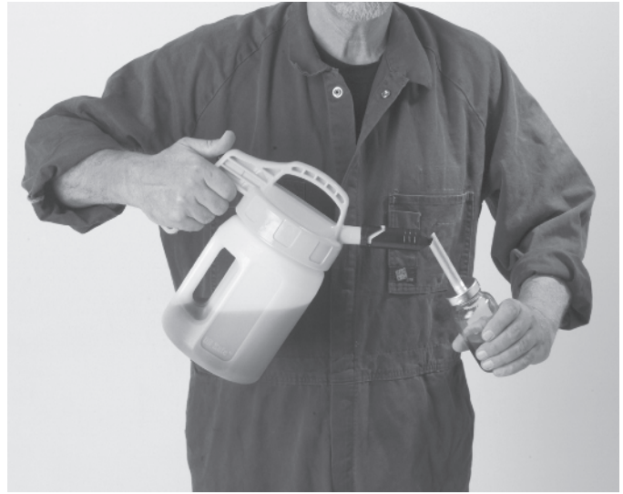
Figure 10-28: Using a high-grade lube oil transfer container to refill a pump constant level lubricator bottle (Source: Oil Safe® Systems Pty. Ltd.)
