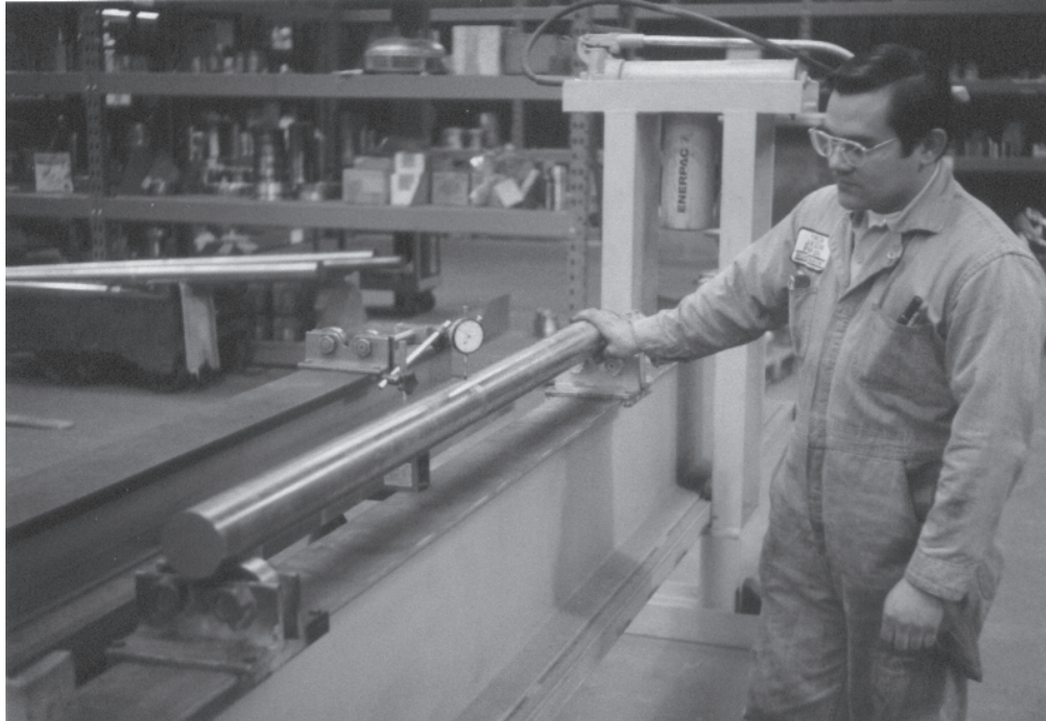
Figure 15-17: Checking shaft straightness (Source: Byron Jackson Division of Flowserve Pumps, Kalamazoo, Michigan)
