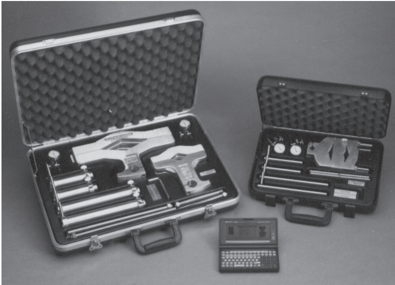
Figure 3-48: Reverse indicator devices and components in carrying case (Source: A-Line Mfg. Co., Liberty Hill, Texas 78642)
