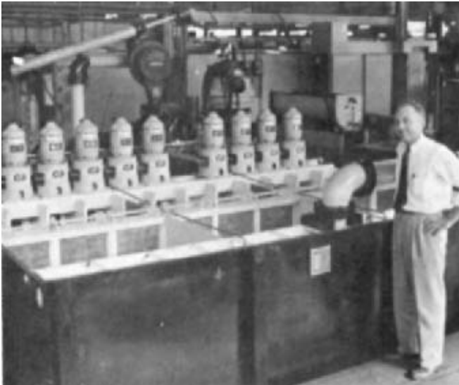
FIGURE 17 Model pit test setup with fixed screens and pumps and valves for variable flow, to scale (Flowsolve Corporation)
