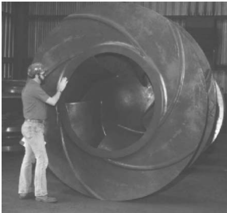
FIGURE 2 Dredge pump impeller, 105 in (2.67 m) diameter
