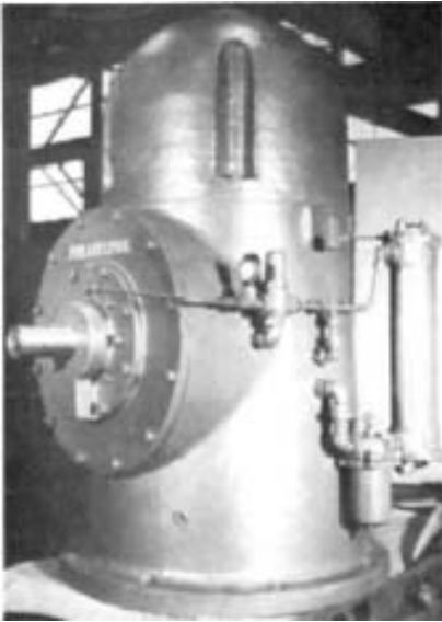
FIGURE 1 Spiral-bevel gear, right-angle vertical pump drive
