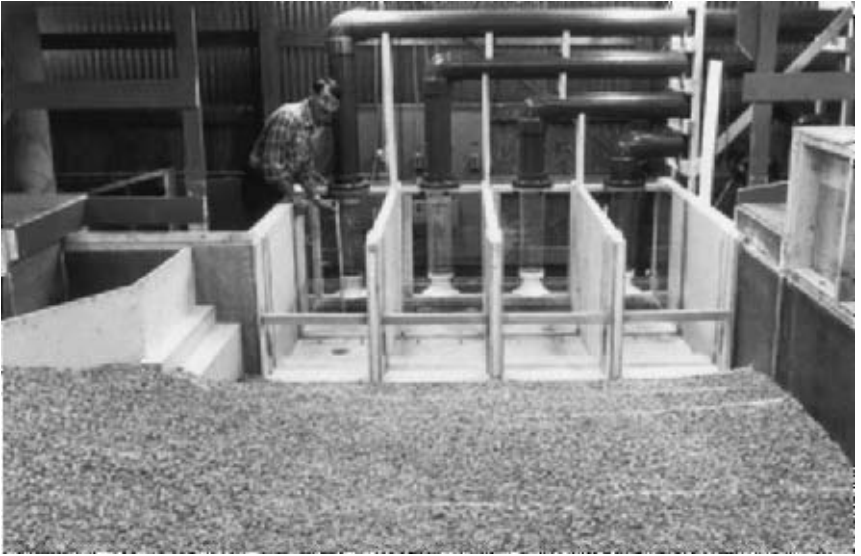
FIGURE 4A A 1:10 geometric scale model of a four pump-bay pump intake (Courtesy of Alden Research Laboratory, Inc.)
