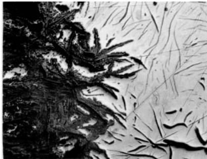
FIGURE 2 The interface between the advancing graphitized front and the sound base metal. Graphitic corrosion propagates along the path of the graphite flakes (50 \times ).
