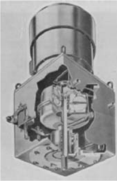
FIGURE 13 Cutaway view of vertical fluid drive suitable for operation with vertical pumps. Note the NEMA P pump flange and output shaft (American Davidson)
