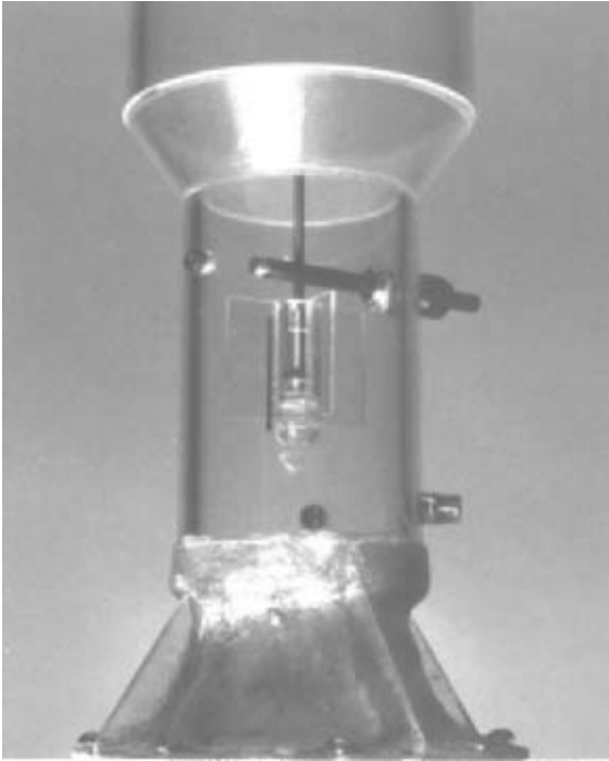
FIGURE 6 Swirl meter in a model pump column (Courtesy of Alden Research Laboratory, Inc.)
