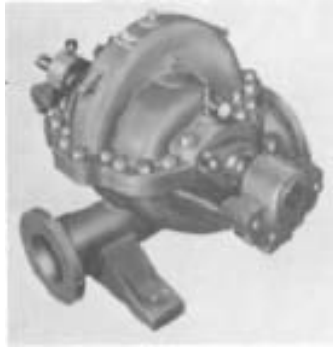
FIGURE 10 An axially split casing, horizontal-shaft, double-suction volute pump (Flowsolve Corporation)
