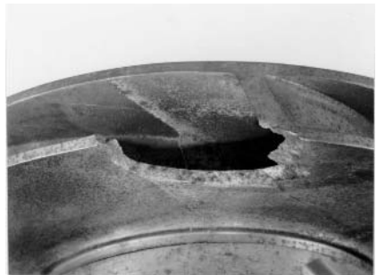
FIGURE 20 A higher magnification of one of the fatigue fractures that originated at a corrosion pit at the exit vane tip and shroud intersection. Additional corrosion pitting can be seen on the impeller in this figure.
