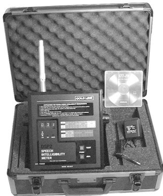
EXHIBIT 14.12 Speech Intelligibility Meter. (Source: Gold Line, West Reading, CT)
