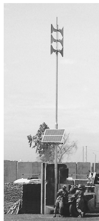
EXHIBIT 24.10 High Power Speaker Array. (Source: Cooper Notification, Long Branch, NJ)
