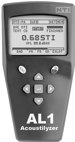
EXHIBIT S3.9 NTI AL1 Displaying Basic STIPA Result. (Source: NTI Americas, Tigard, OR)
