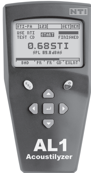
EXHIBIT 18.8 Combination Sound Pressure Level Meter/Analyzer and Speech Intelligibility Meter (left) and AL1 Meter Displaying Basic STI-PA Result (right). [Sources: (left) Gold Line, West Redding, CT; (right) NTI Americas, Tigard, OR]
