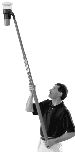
EXHIBIT 14.9 Functional Test of a Smoke Detector. (Source: No Climb Products Ltd., Hertfordshire, UK)
