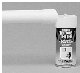
EXHIBIT 14.10 Aerosol Smoke Product for Functional Test of a Smoke Detector. (Source: Home Safeguard Industries, Inc., Rolling Meadows, IL; photo courtesy of R. P. Schifiliti & Associates)
