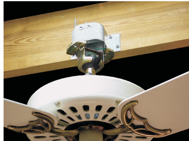
Exhibit 422.2 Supporting a ceiling-suspended (paddle) fan (35 lb or less) with a box identified for such use. (Courtesy of Hubbell RACO)
