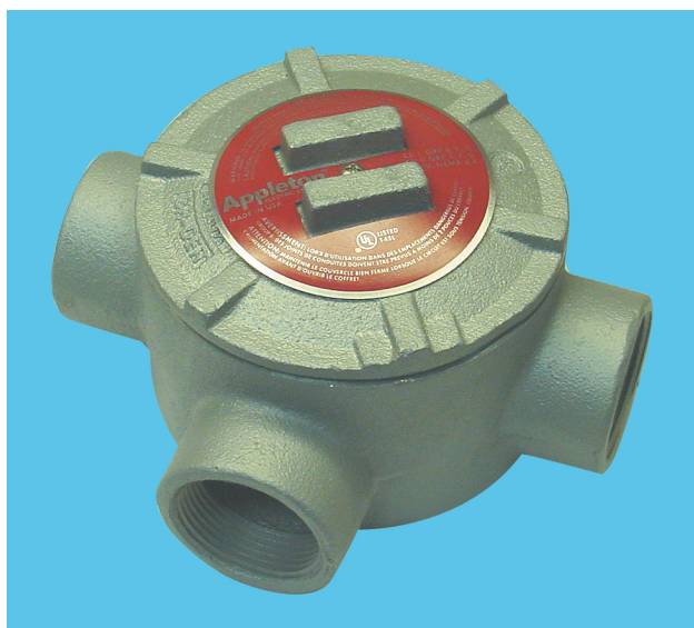
Exhibit 502.1 Junction box with threaded hubs, suitable for use in Class II, Group E hazardous atmospheres. (Courtesy of Appleton Electric Co., EGS Electrical Group)
