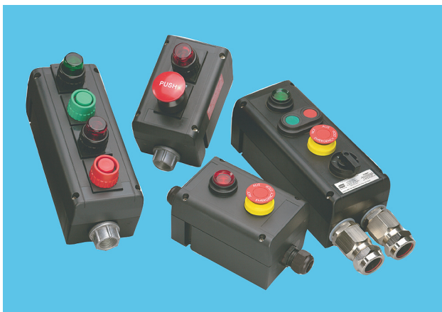
Exhibit 505.1 Typical control stations with the combination of flameproof and increased safety types of protection suitable for use in Class I, Zone 1 areas. (Courtesy of Cooper Crouse-Hinds)
