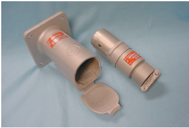
Exhibit 501.23 A 4-pole (delayed action) explosionproof receptacle and attachment plug suitable for use without a switch. (Courtesy of Appleton Electric Co., EGS Electrical Group)
