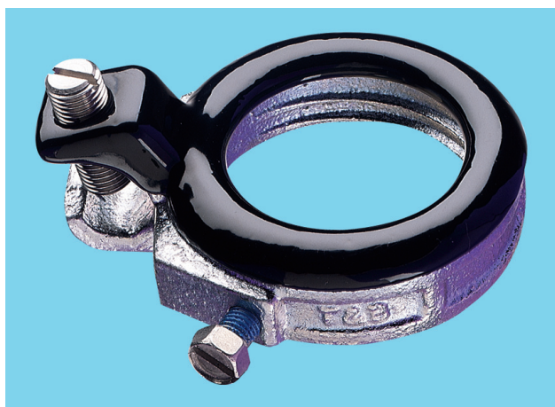
Exhibit 250.36 A threaded grounding bushing with set screws used to ensure electrical and mechanical connection and a terminal for connection of a grounding conductor or bonding jumper. (Courtesy of Thomas & Betts Corp.)
