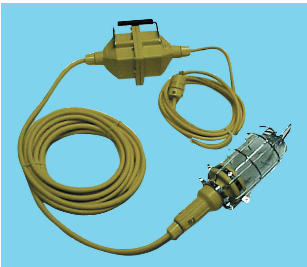
Exhibit 250.45 Lighting equipment supplied through an isolating transformer operating at 6 or 12 volts and therefore not required to be grounded. (Courtesy of Daniel Woodhead Co.)
