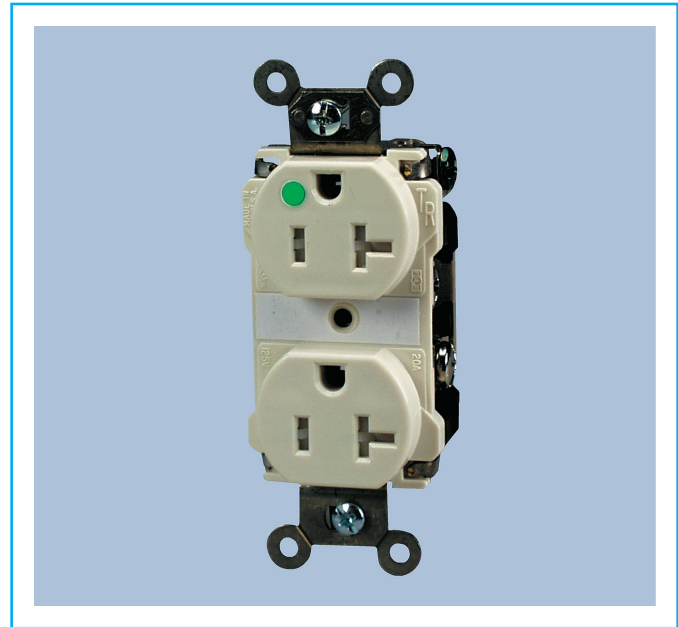
Exhibit 517.1 A tamper-resistant hospital-grade receptacle, identified by a green dot on its face, that fulfills the requirements of 517.18(B) and 517.18(C). (Courtesy of Pass & Seymour/LeGrand®)
