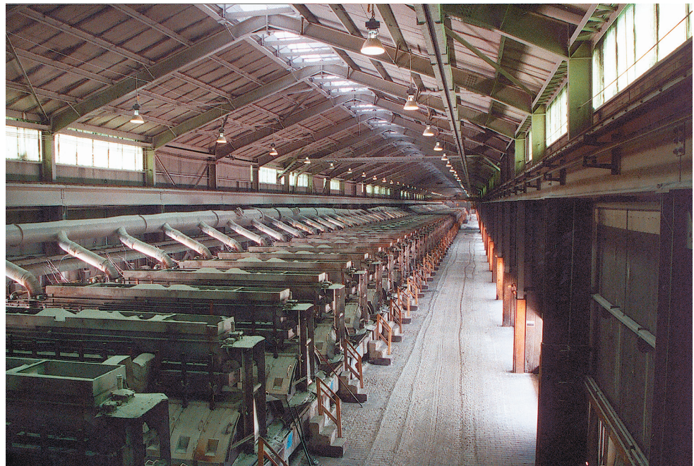
Exhibit 668.1 A typical pot room in an aluminum reduction plant. (Courtesy of Alcoa Inc.)
