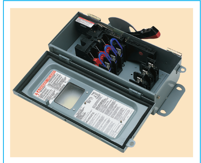
Exhibit 430.22 Heavy-duty safety switches, UL-listed for use on systems up to 200,000 amperes, fault current rms symmetrical with Class J or Class R fuses installed. (Courtesy of Square D Co.)
