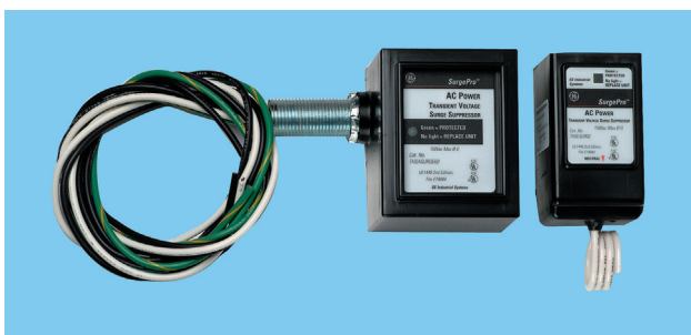
Exhibit 285.1 Two TVSS devices suitable for service-entrance installation, one for direct connection to panelboard busbars and one for mounting in an cabinet or enclosure knockout. (Courtesy of General Electric Co.)
