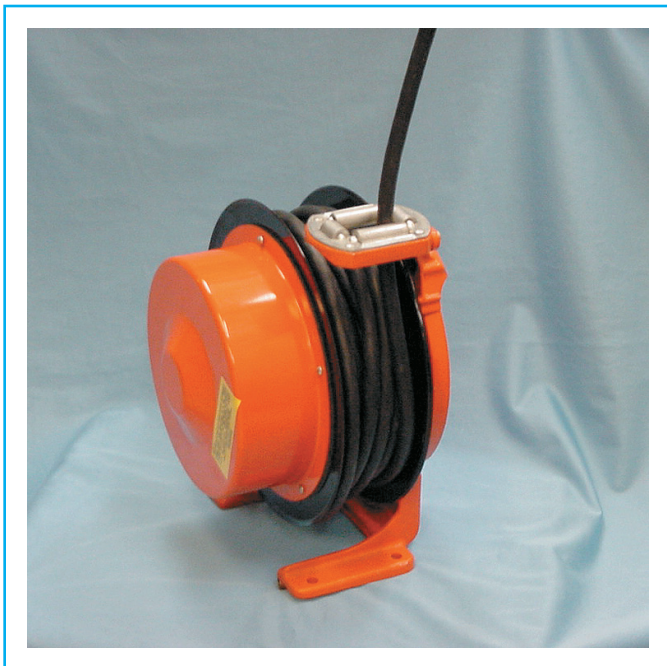
Exhibit 511.2 Cord reel. This cord, which is part of a portable lamp assembly, must be arranged so that the lamp cannot be used in a Class I location. Otherwise, the lamp must be an explosionproof type approved for Class I, Division 1 hazardous locations. (Courtesy of Appleton Electric Co., EGS Electrical Group)
