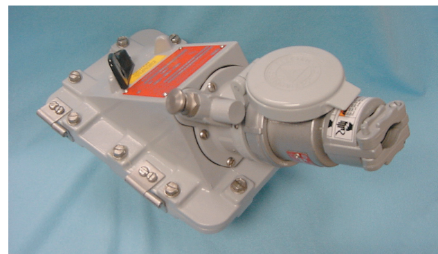
Exhibit 501.22 A receptacle and attachment plug of the explosionproof type with an interlocking switch. The switch must be in the off position before the attachment plug can be removed. (Courtesy of Appleton Electric Co., EGS Electrical Group)
