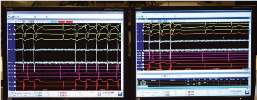
Figure 3.3 The page displayed during studies typically shows several intracardiac electrograms with 3 to 4 surface ECG leads which allows for axis determination, activation timing, and P/QRS morphology.
