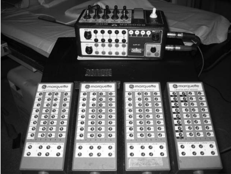
Figure 3.2 The junction boxes receive the intracardiac signals from the catheters and provide an interface into the physiologic recorder.
