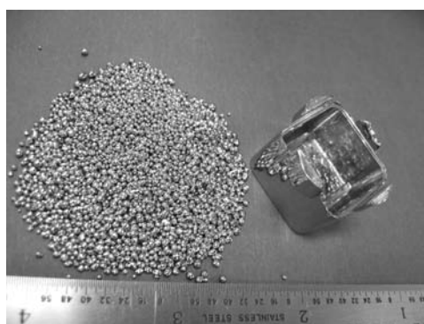
FIGURE 17.20 Feedstock material and superplastically formed part made of the metallic glass Pt_{57.5}Cu_{14.7}Ni_{5.3}P_{22.5} . (Reproduced from Schroers, J., J. Mater. JOM 57, 35, 2005. With permission.)
