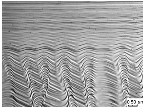
FIGURE 15.3 Interface instability caused by constitutional supercooling during the Czochralski growth of a GeSi single crystal with 2% at Si. The crystal was pulled in the \langle 112 \rangle direction (Courtesy of IKZ — SiGe group).
