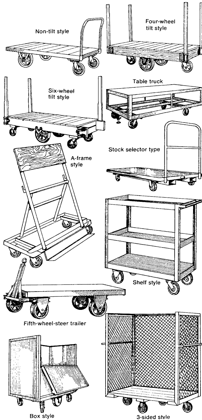
FIGURE 4.40 Factory trucks and wheel arrangement patterns. (Reproduced with permission from Material Handling Engineering Handbook and Directory, 1979–1980, published by Material Handling Engineering magazine, Cleveland, Ohio.)
