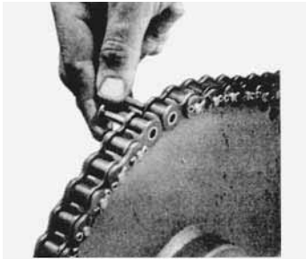
FIGURE 5.100 Inserting connecting link.
