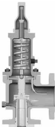
FIGURE 5.191 Conventional safety relief valve.
