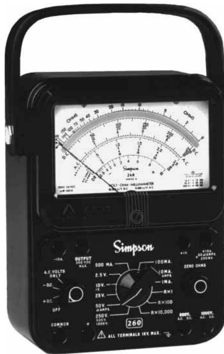
FIGURE 5.1 Analog volt-ohm-milliammeter (VOM).
