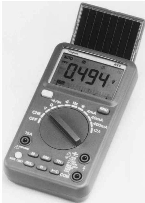
FIGURE 5.2 Digital multimeter (DMM).
