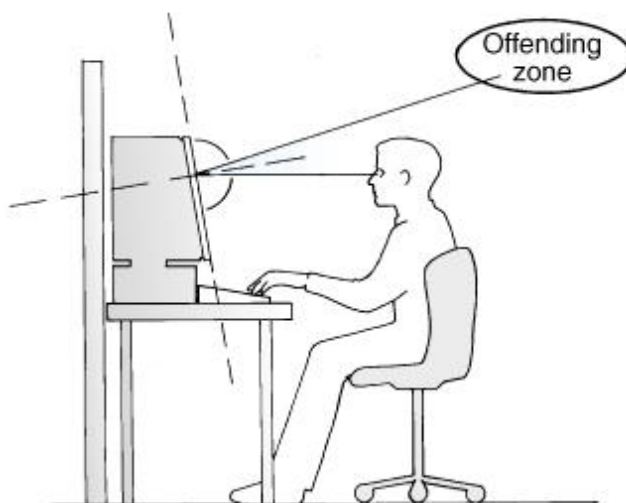
Figure 11-18. Depending on the eye-screen geometry, the offending zone may be located on the ceiling plane, a wall, or a partition. Screen curvature may enlarge or change the location of the offending zone.
