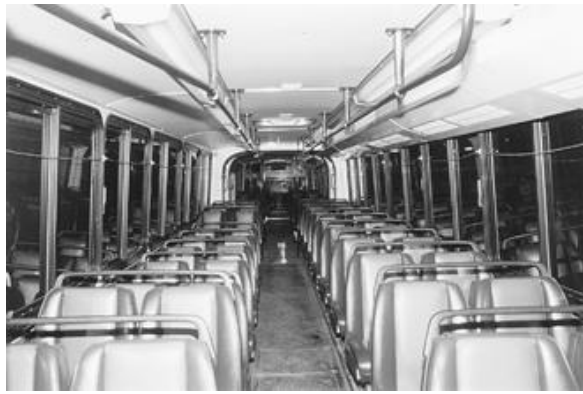
Figure 23-8. Articulated city bus. Fluorescent luminaires mounted end to end over the passenger seats provide diffuse semidirect illumination. Dome lights are incandescent.
