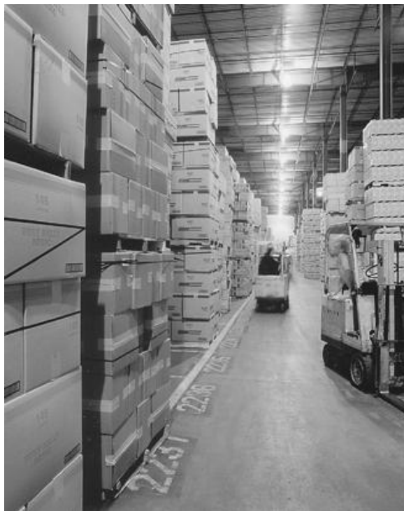
Figure 19-32. Storage areas must provide good vertical illuminance to facilitate reading labels and adequate horizontal illuminance to allow safe movement and proper location identification.
