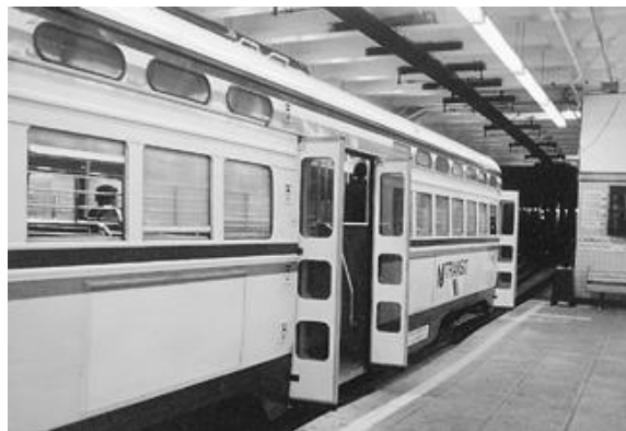
Figure 23-13. Well-lighted underground rail station platforms add to passenger comfort and safety. It is important that the car entrance and exit areas have good lighting.
