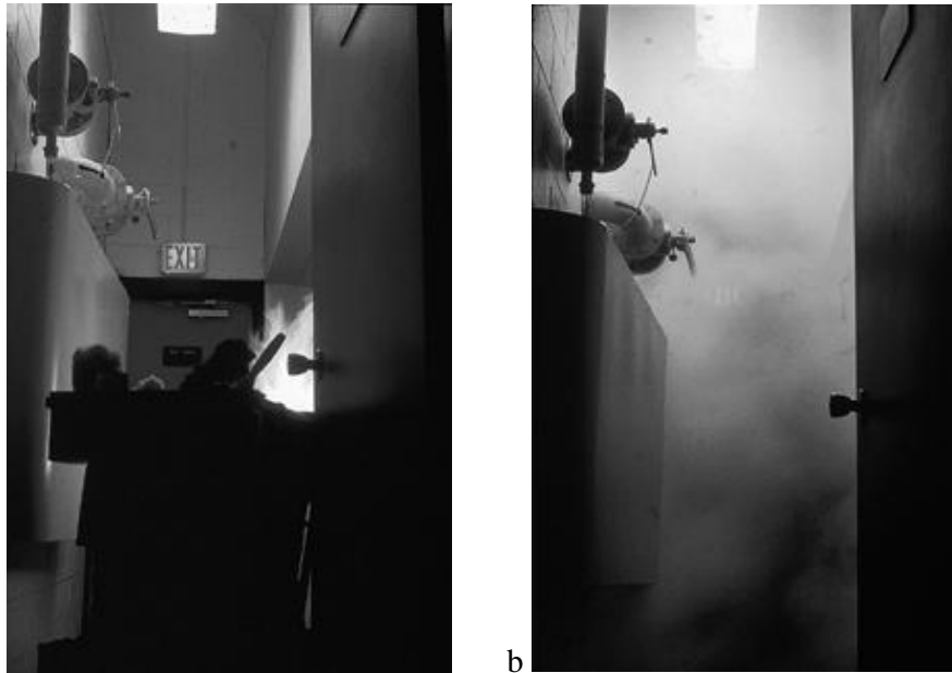
Figure 29-8. a. Exit sign visible in smoke-free fire. b. Exit sign nearly obscured in smoke. Visibility is greatly reduced by the glare from the overhead luminaire.
