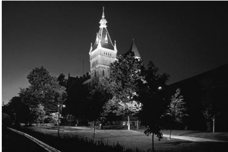
Figure 21-2. The lighting for this church uses varied surface brightness to add interest and depth.
