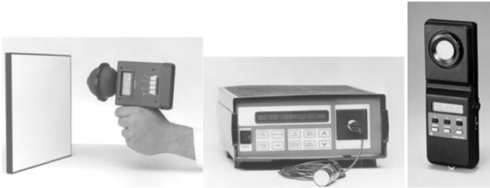
Figure 2-7. Various commercial illuminance meters. (a) Portable illuminance meter with small integrating sphere; (b) laboratory grade system that includes a photometer, a radiometer, and a fiber-optic power meter; (c) multifunction portable illuminance meter with detachable receptor head.
