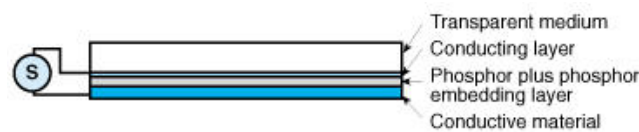
Figure 1-19. Diagrammatic cross section of an electroluminescent lamp.
