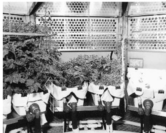
Figure 5-28. The Biomass Production Chamber at Kennedy Space Center, where they are developing systems to raise food in the space colonies of the future. The lighting is high pressure sodium at a very high intensity. The plants in this picture are potatoes.
