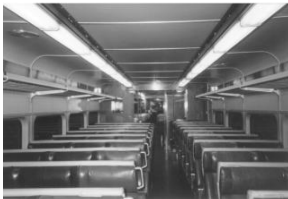
Figure 23-18. Linear luminaires with well-designed diffusers distribute light uniformly throughout the car and control glare from the luminaires. Light-colored, matte interior finishes would have been effective in glare control in the car pictured.
