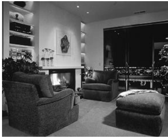
Figure 18-4. Lighting contributes to a room's aesthetics and atmosphere. This inviting living room, with its extraordinary view of the city, features downlighting in the seating area, accent lighting on the painting and sculpture over the fireplace, and shelf lighting to illuminate the stereo and highlight decorative items.
