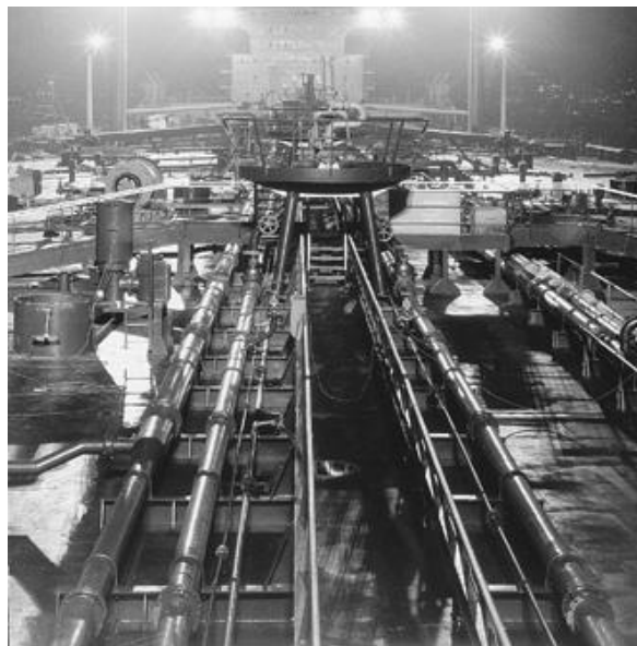
Figure 23-36. Deck illuminance on a tanker is provided by high-tower floodlights using HID lamps.
