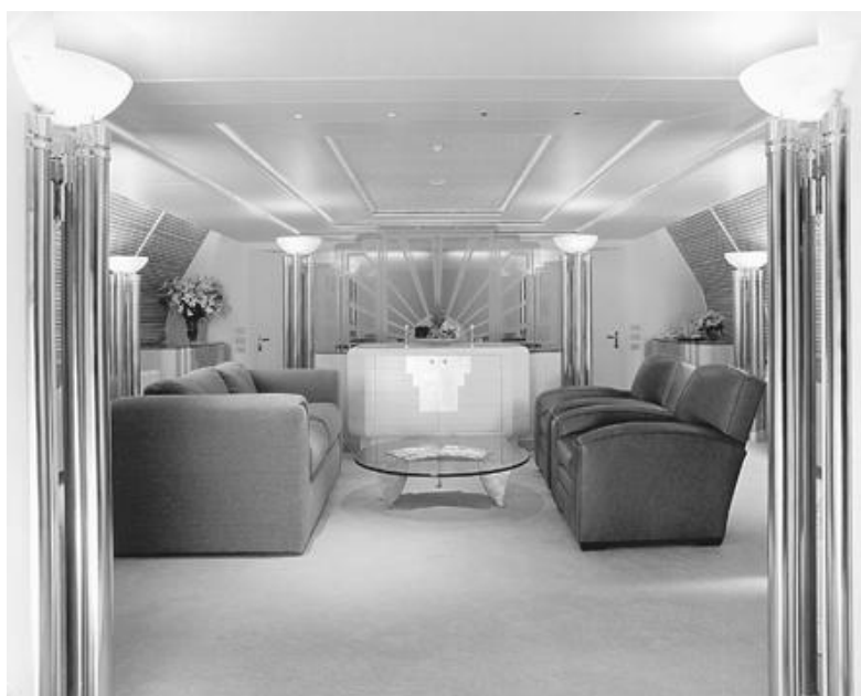
Figure 23-33. Lounge space aboard the M/Y Lady Tiffany showing a combination of recessed, cove, wall mounted, and torchiere luminaires.
