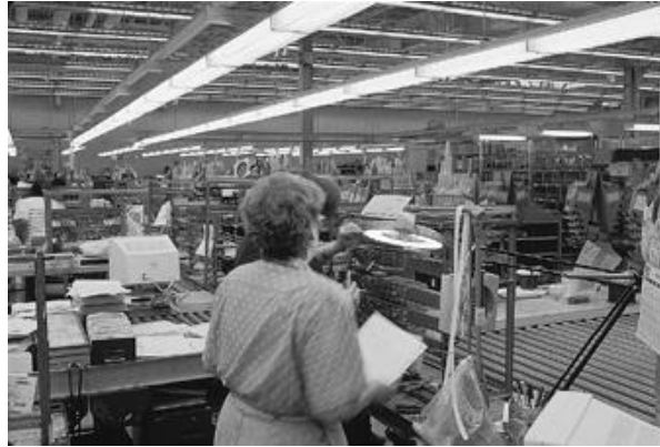
Figure 19-14. Supplementary general lighting with diffusers, permanently installed at a lower level to improve visibility where more demanding visual tasks occur. Note the circular fluorescent magnifying luminaire to aid critical inspection tasks.
