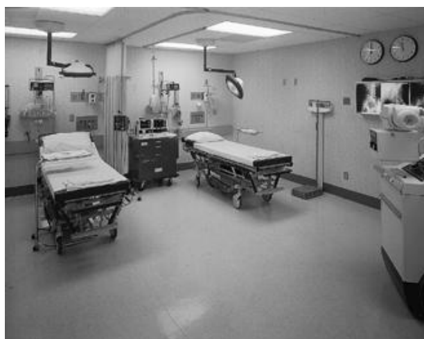
Figure 16-3. Critical care room. Dimmable fluorescent lighting provides general illumination. Surgical
