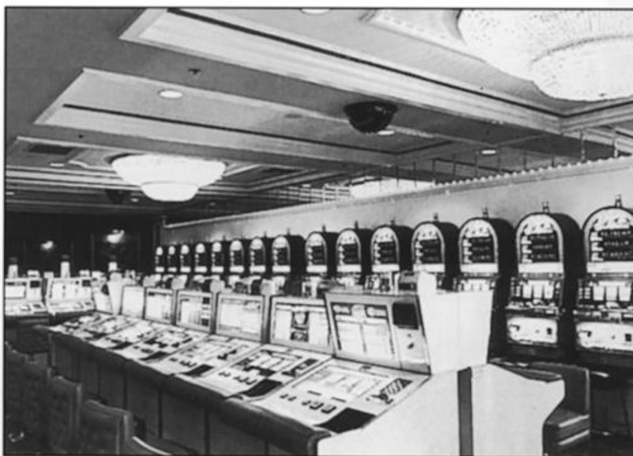
Figure 13-17. Lighting has been integrated with the ceiling design to focus interest on the video machines.
