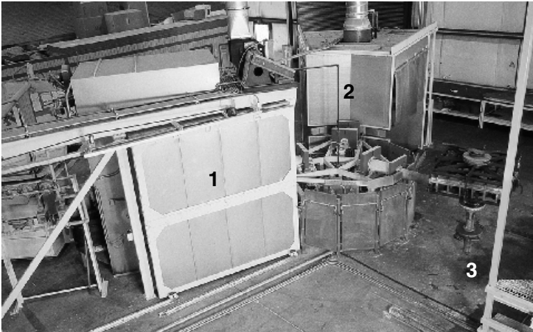
FIGURE 6.27 Three-arm turret machine showing the oven (1), cooler (2), and servicing (3) stations. (Courtesy of Ferry Industries, Inc.)
