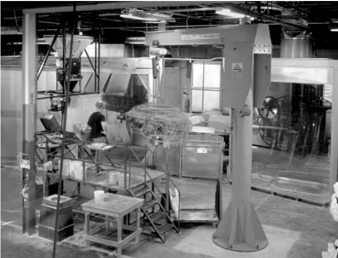
FIGURE 6.22 Platform used to raise an operator to the level of a mold. (Courtesy of Ferry Industries, Inc.)
