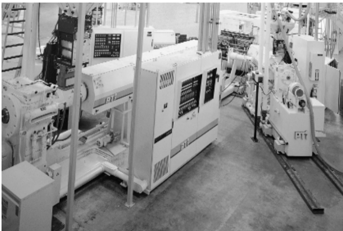
FIGURE 3.58 Extruded arrangement for a four-layer structure. (Courtesy of PTi, Aurora, IL.)
