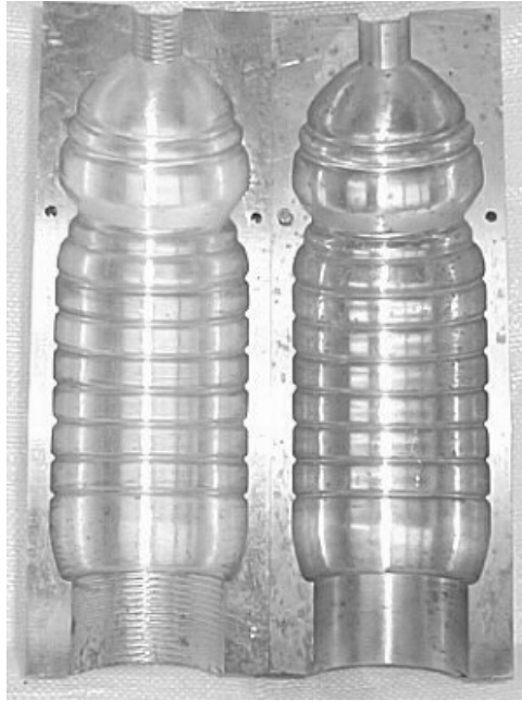
FIGURE 5.56 Mold cavities for a 1-liter water bottle. (Courtesy of Roa Designs International, Schiller Park, IL.)
