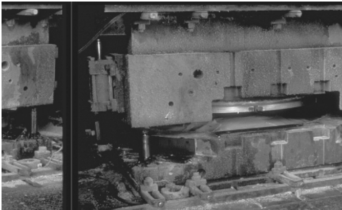
FIGURE 8.14 Compression molding operation. (Courtesy of Owens Corning. Used with permission.)
