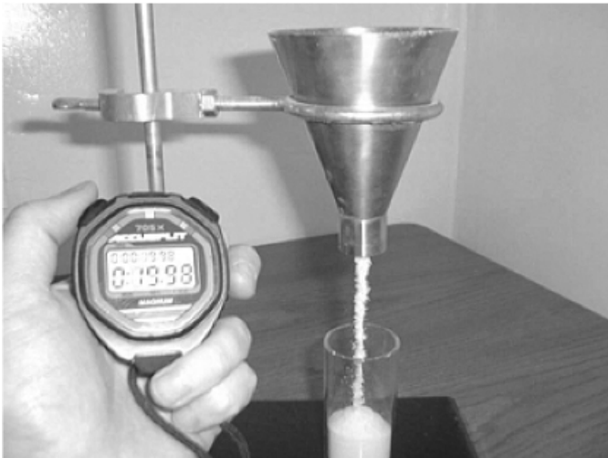
FIGURE 6.11 Free-flowing powder during a flow rate test.
