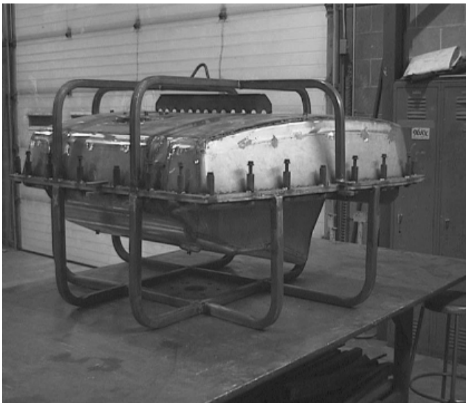
FIGURE 6.16 Stainless steel mold supported in a steel frame at parting lines. (Courtesy of Rivers Metal Molds, Inc.)
