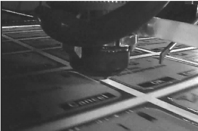
FIGURE 9.23 Jet dispensing of a UV gasket material on a cell phone display.
