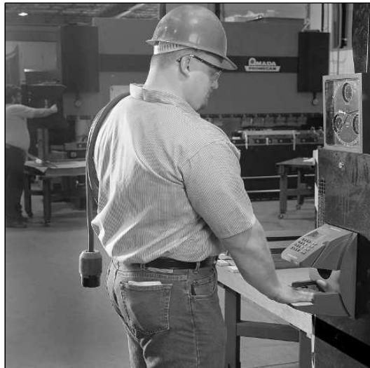
Fig. 23.5. A hand-geometry biometric time and attendance system being used in a factory environment. Picture courtesy of Ingersoll Rand.
