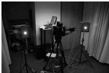
Fig. 15.7. Camera and lighting setup for image collection
