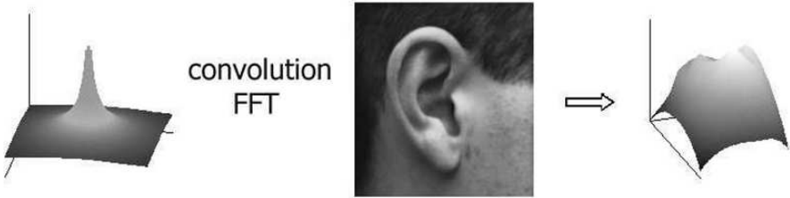
Fig. 7.8. Generating an ear energy surface by convolution. The energy field for an ear (right) is obtained by locating a unit value potential function (left) at each pixel location and scaling it by the value of the pixel and then finding the sum of all the resulting functions. For efficiency this is actually calculated in the frequency domain.
