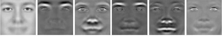
Fig. 3.1. The first six basis vectors of Eigenfaces.
