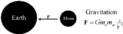
Fig. 7.7. Newton’s Universal Law of Gravitation. The earth and moon are mutually attracted according to the product of their masses m_e and m_m respectively, and inversely proportional to the square of the distance between them. G is the gravitational constant of proportionality.
