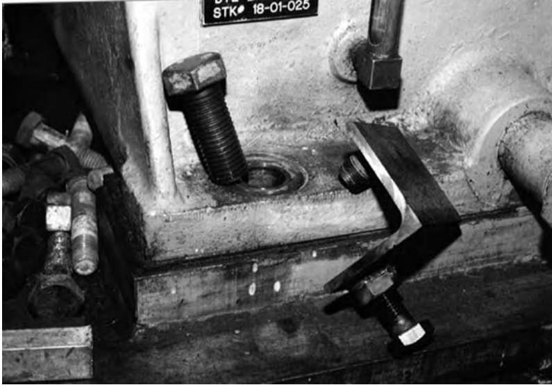
FIGURE 7.21 Drop-in puller device ready to be inserted into bolt hole on machine case.
