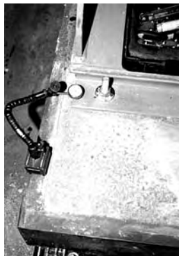
FIGURE 5.53 Checking for lift with a magnetic base and dial indicator on a fan frame.
