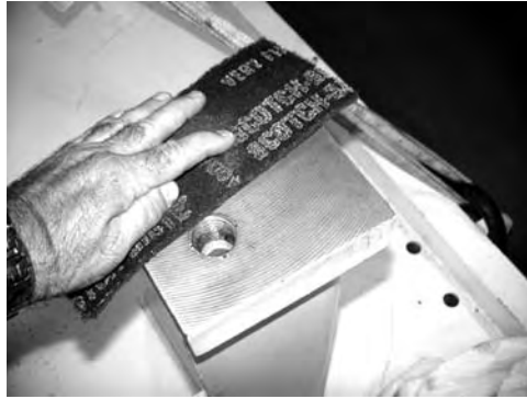
FIGURE 3.34 Cleaning the top surfaces of each mounting point.
