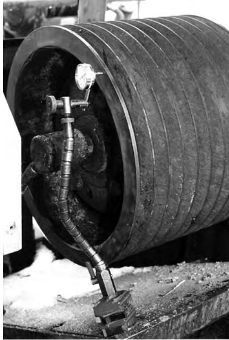
FIGURE 5.32 Measuring face runout on a multi-V sheave.
