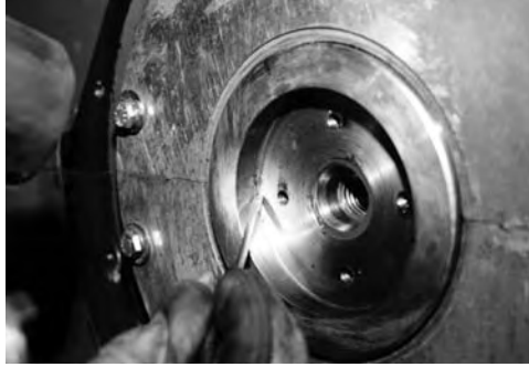
FIGURE 5.30 Metal shaving found on mating face of stub shaft causing the runout in Figure 5.29.
