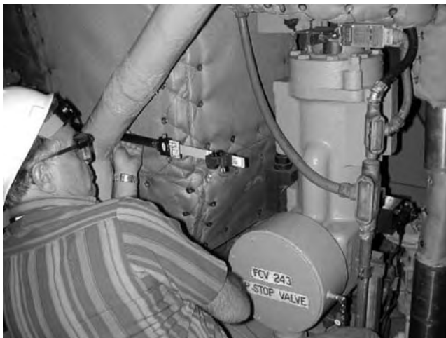
FIGURE 16.49 Jig transit and scale target on outboard pump bearing for lateral measurement.
