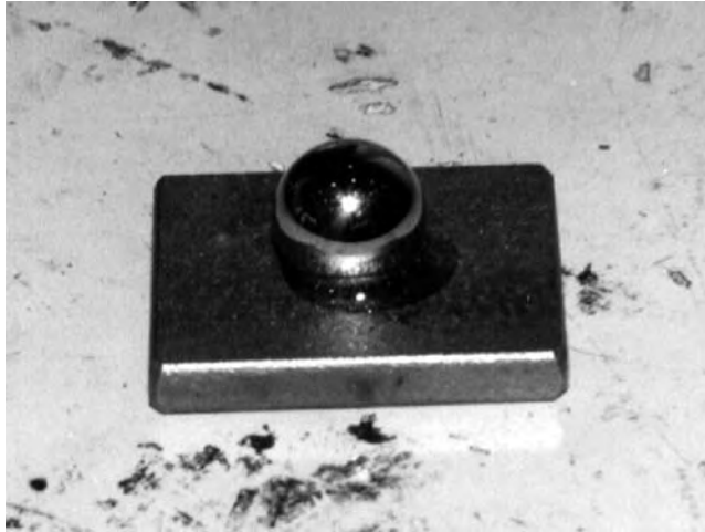
FIGURE 16.9 Tooling ball fabricated from 0.5 in. steel ball and 1.5 in. × 1.5 in. × 0.25 in. steel plate with the ball welded to the plate.
