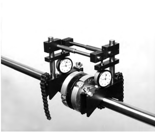
FIGURE 6.75 PAS-1 system set up for reverse indicator method. (Courtesy of Benchmark Maintenance Services Inc., Toronto, Ontario, Canada. With permission.)
