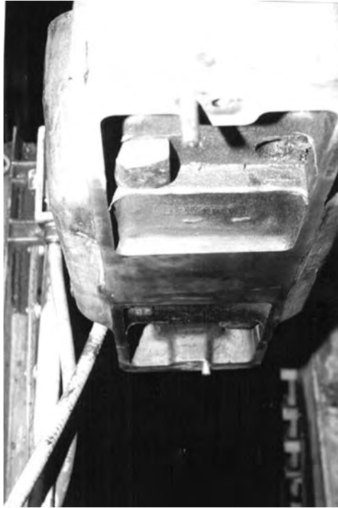
FIGURE 5.55 Underside of pillow block bearing lower casting.
