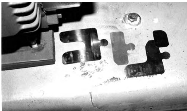
FIGURE 5.50 Soft foot correction shims stack.
