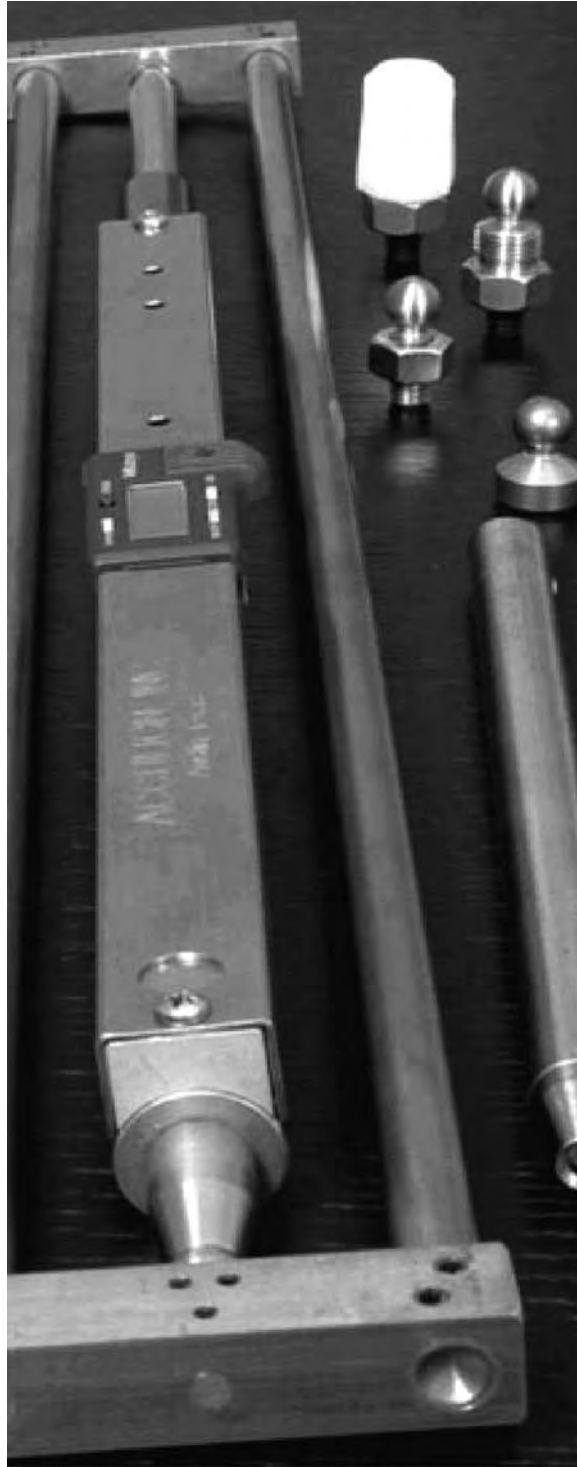
FIGURE 16.16 Acculign micrometer in calibration fixture. (Courtesy of Acculign, Austin, TX, www.acculign.com . With permission.)
