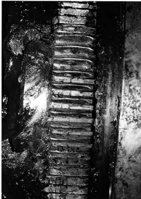
FIGURE 5.20 Excessively worn gear coupling.
