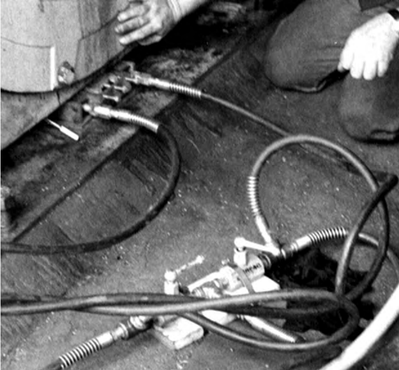
FIGURE 7.17 Hydraulic machinery lifting and lateral positioning device. (Courtesy of Murray & Garig Tool Works, Baytown, TX. With permission.)
