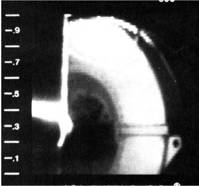
FIGURE 16.7 Thermal image of compressor end casing.
