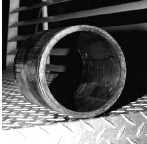
FIGURE 21.32 Excessively worn upper pump bushing due to excessive lateral misalignment.
