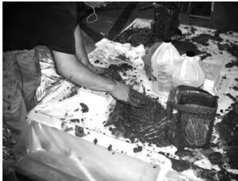
FIGURE 3.54 Hand packing the grout.
