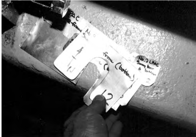
FIGURE 5.48 Soft foot correction shim stack.
