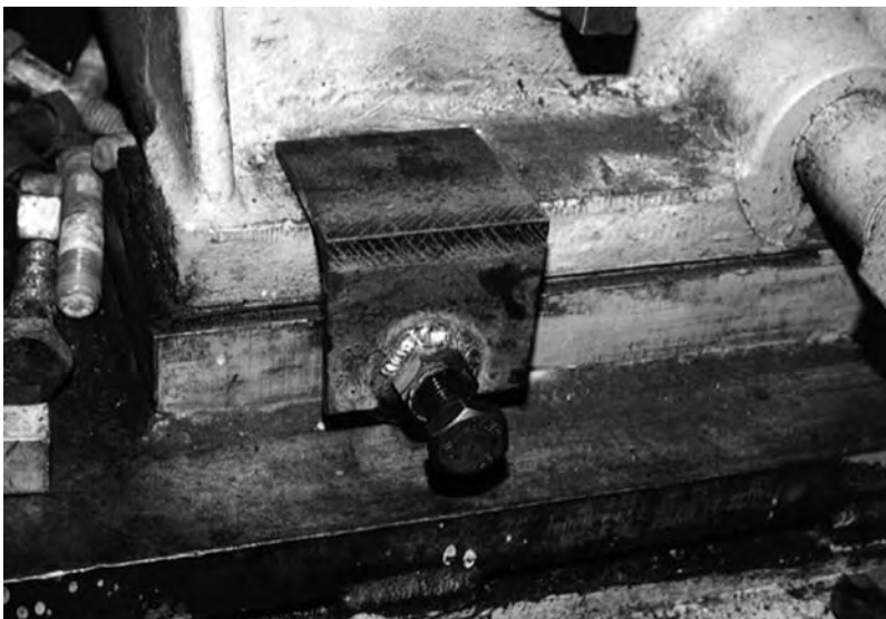
FIGURE 7.22 Drop-in puller device inserted into hole and ready to pull machine sideways.
