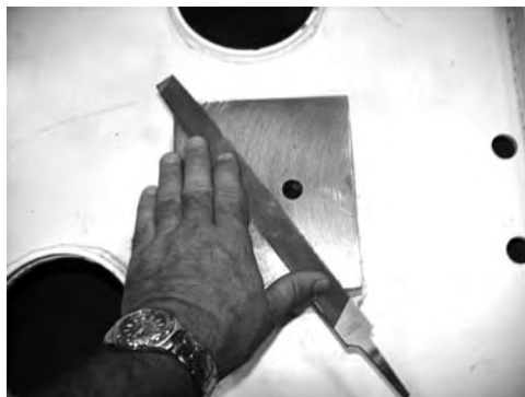
FIGURE 3.35 Removing burrs with a flat file.
