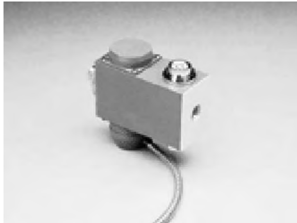
FIGURE 20.27 Hamar Model T-261A 4 axis target. (Courtesy of Hamar Laser Instrument Co., Danbury, CT. With permission.)
