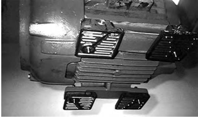
FIGURE 5.59 Foot plane compensator. Underside view showing epoxy channels. (Courtesy of Max Roeder Consulting, Inc., Danville, IN.)
