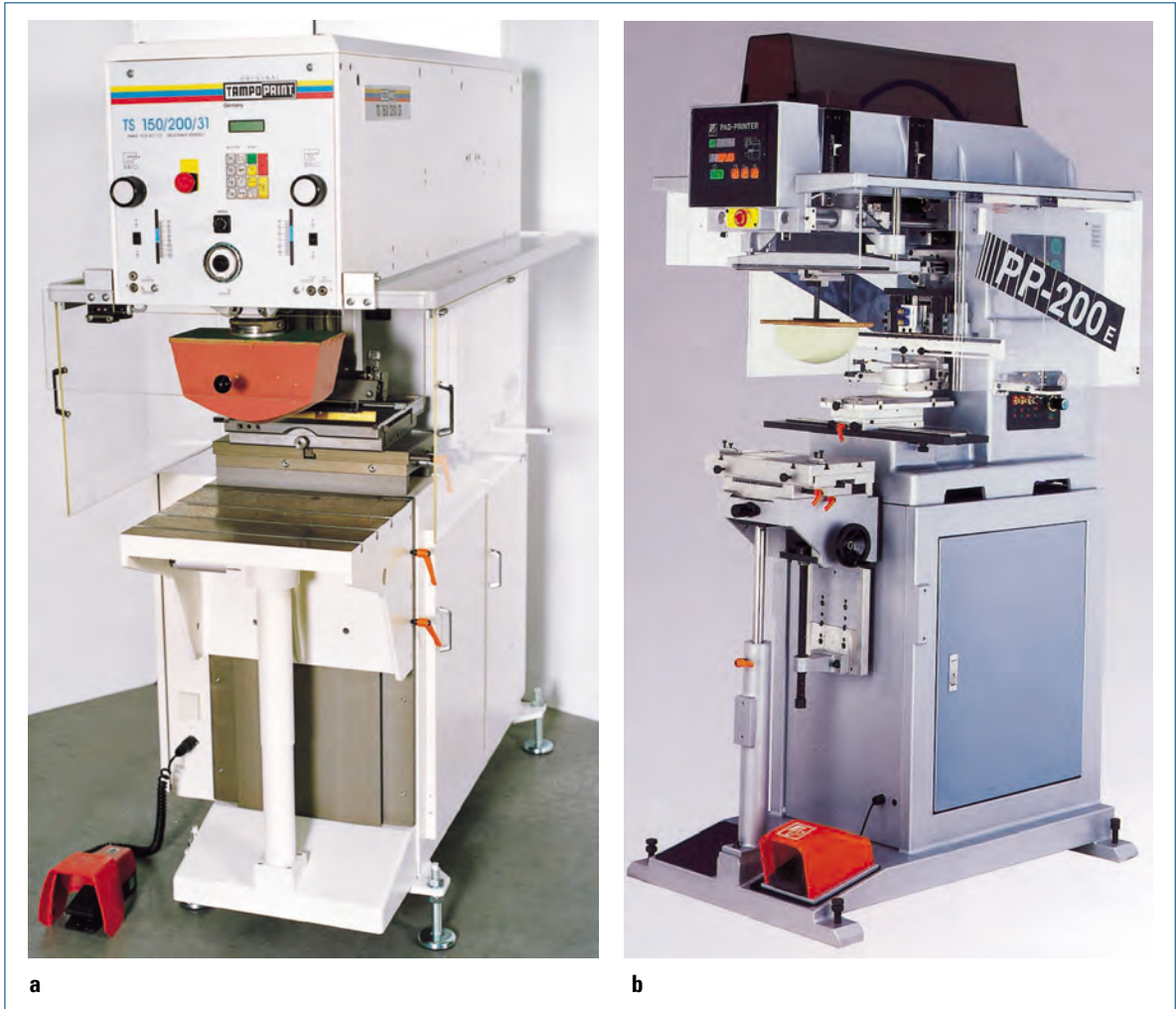
Fig. 2.5-34 Single-color pad transfer printers. a Press with open inking system (TS 150/200/31, Tampoprint); b Press with closed inking system (Pad Printer PP 200, Mino Group)
