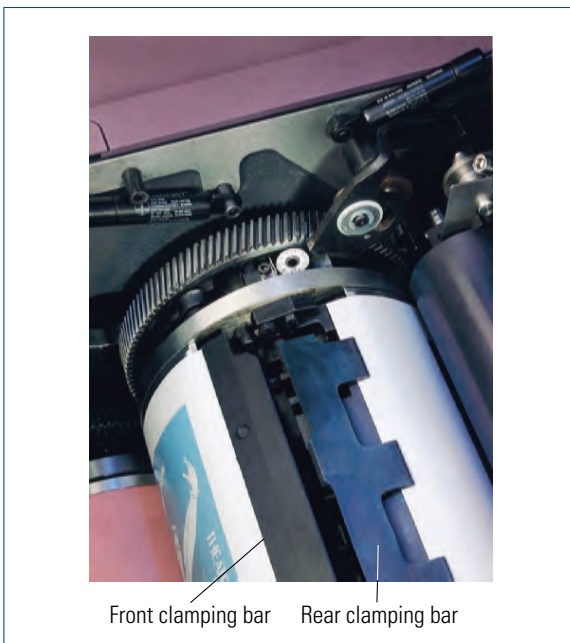
Fig. 2.1-42 Plate clamping (Printmaster QM 46, Heidelberg)
