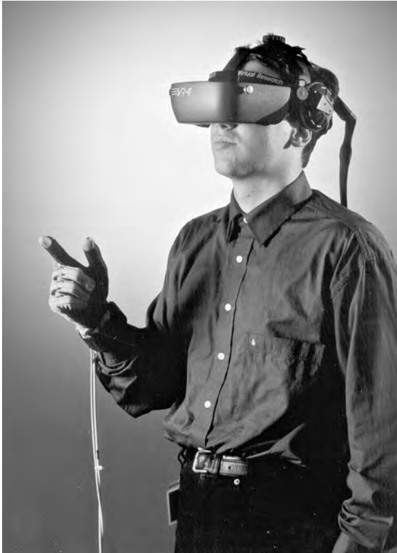
Fig. 11.2-7 Components for interaction (man and machine) in virtual reality: data glove and data helmet including head mounted display
