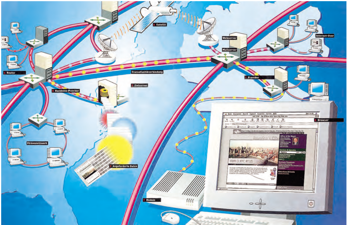
Fig. 3.2-59 Structure and components of a global network (Internet) for data transmission and communication (EnBW/Zbigniew Sroga)
