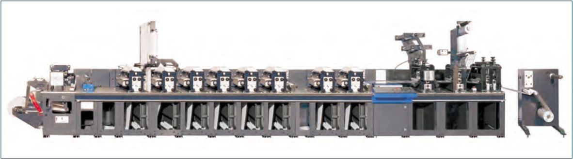
Fig. 2.3-21 Flexographic label printing press with UV drying and rotary die-cutter, speed 2.5 m/s (Arsoma EM 510, Heidelberg/Gallus)
