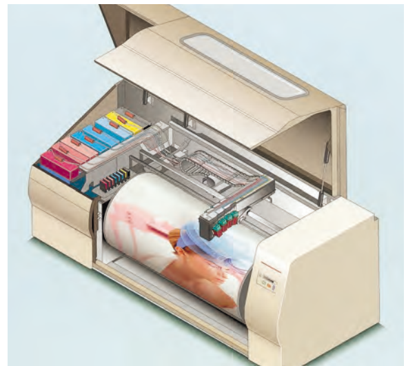
Fig. 4.1-9 Ink jet printing system for digital multicolor proofing (AGFA Jet)
