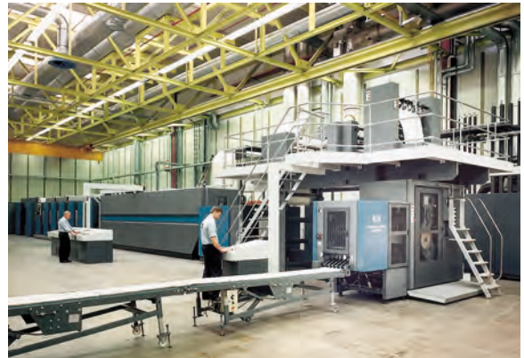
Fig. 1.2-36 Web-fed offset printing system (M-600, Heidelberg)
