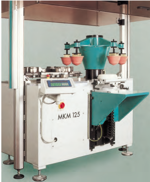
Fig. 2.5-40 Multicolor carousel pad transfer printer (MKM 125, Morlock)
