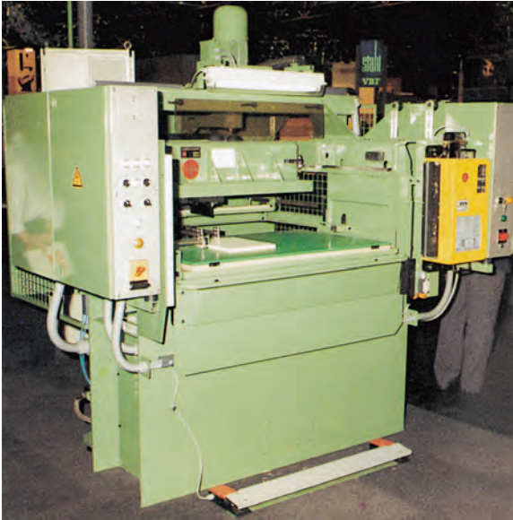
Fig. 7.2-15 Hydraulic flat-bed/bridge die-cutter with reversible bridge (Model 6100B, Schön & Sandt)
