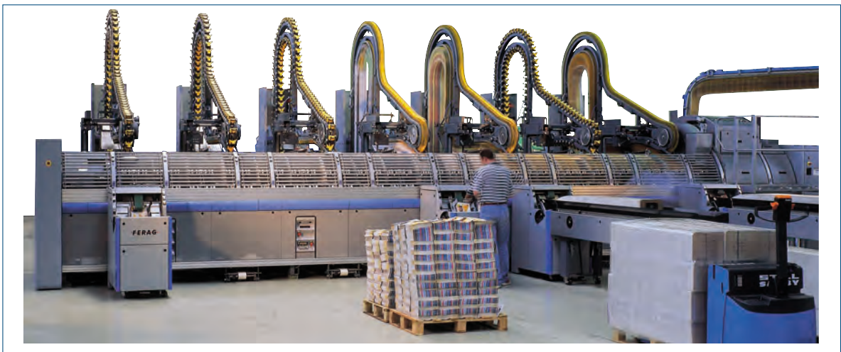
Fig. 7.2-60 Saddle-stitcher drum for the production of magazines (Ferag)
