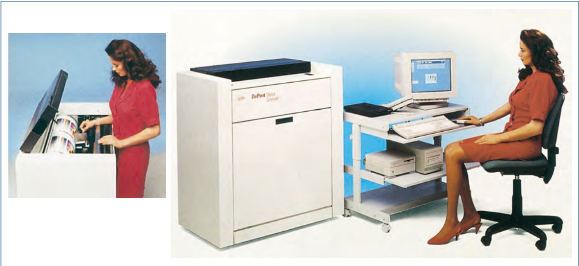
Fig. 1.3-31 Multicolor ink jet printing system (continuous ink jet) for proof production (Digital Cromalin, DuPont)
