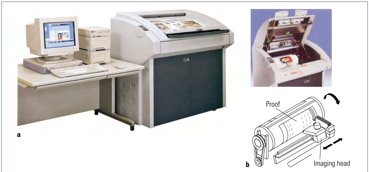
Fig. 5.5-8 Digital proof system with continuous ink jet NIP technology.
