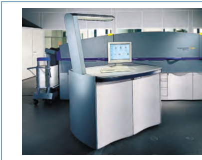
Fig. 9.2-11 Digital production multicolor sheet-fed printing system (electrophotography, 600 dpi, multiple gray values per pixel, LED imaging system, unit construction/singlepass design, intermediate blanket cylinder, format A3+/portrait, 70 A4 pages/min, 2100 A3 pages/h) with perfecter for in-line printing on both sides of the sheet (NexPress 2100, Heidelberg/ Kodak)
