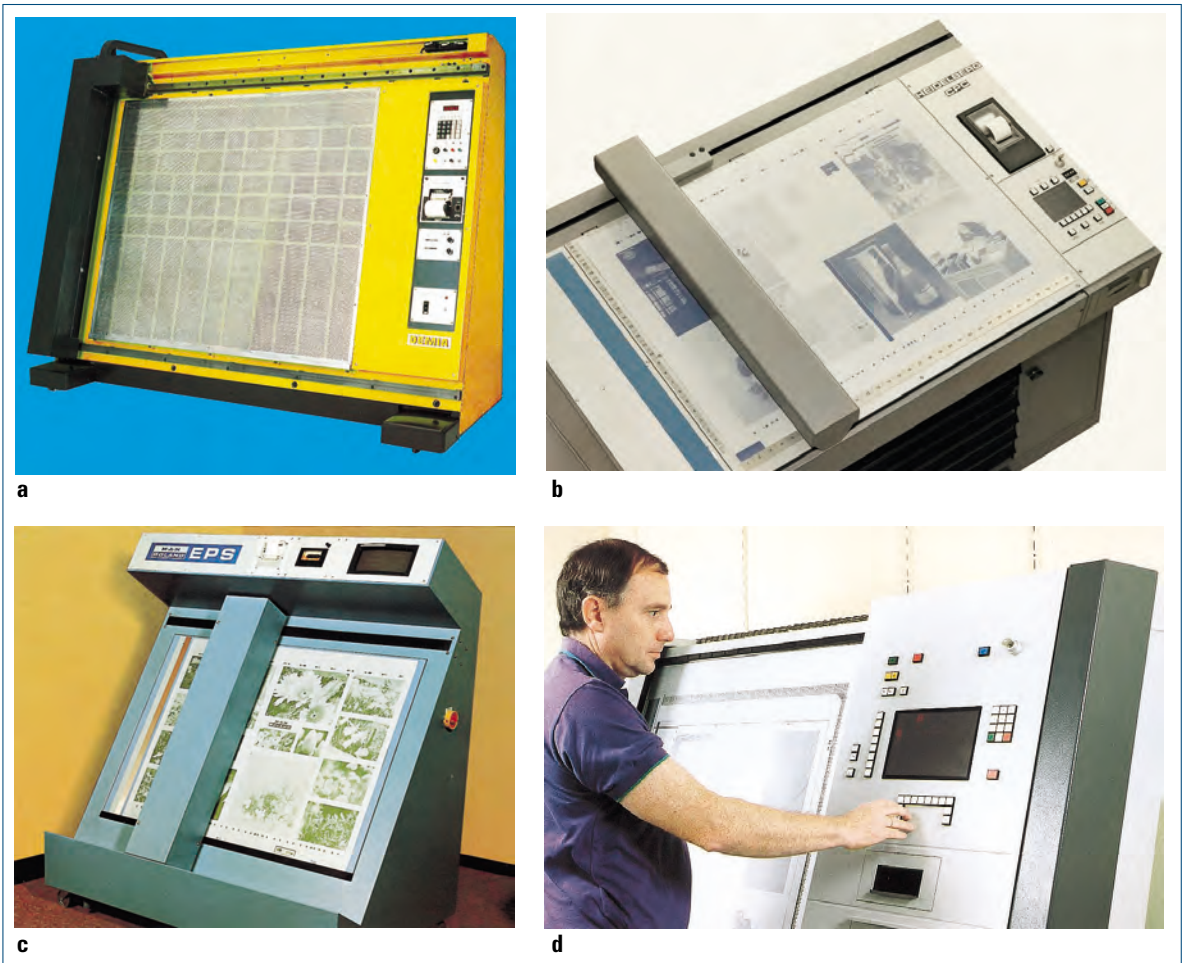
Fig. 2.1-127 Plate image reader designs for ink presetting operations. a DEMIA plate image reader (Device for Measuring an Image Area, Dai Nippon Printing); b CPC3 plate image reader (Computer Print Control, Heidelberg); c EPS plate image reader (Electronic Plate Scanner, MAN Roland); d CPC31 plate image reader (Heidelberg)
