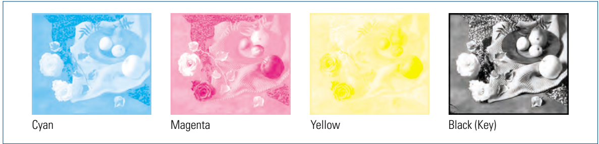
Fig. 11.2-4 Four channels of a CMYK image for four-color printing (in accordance with fig. 11.2-2c)
