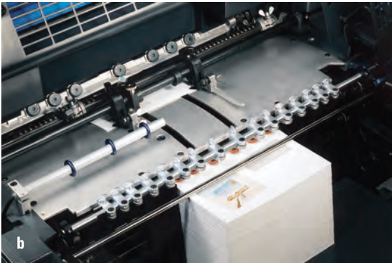
Fig. 2.1-23 Single-sheet feeder. a Diagram of the sheet transportation; b Example of a single-sheet feeder (Heidelberg)
