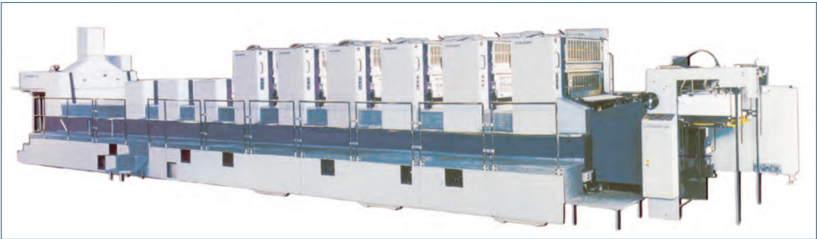
Fig. 2.1-174 Lithrone 40, 6-color press, two coating units, unit for intermediate drying, hot-air extraction in the delivery; sheet size 720 mm × 1030 mm, printing speed 15000 impressions/hour (Komori)
