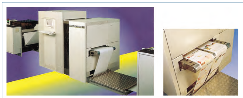
Fig. 5.4-7 Printing system for magnetography-based digital printing for printing paper webs. Resolution: 480 dpi, printing speed 1 m/s (Nipson 7000, Nipson; status: 1998)
