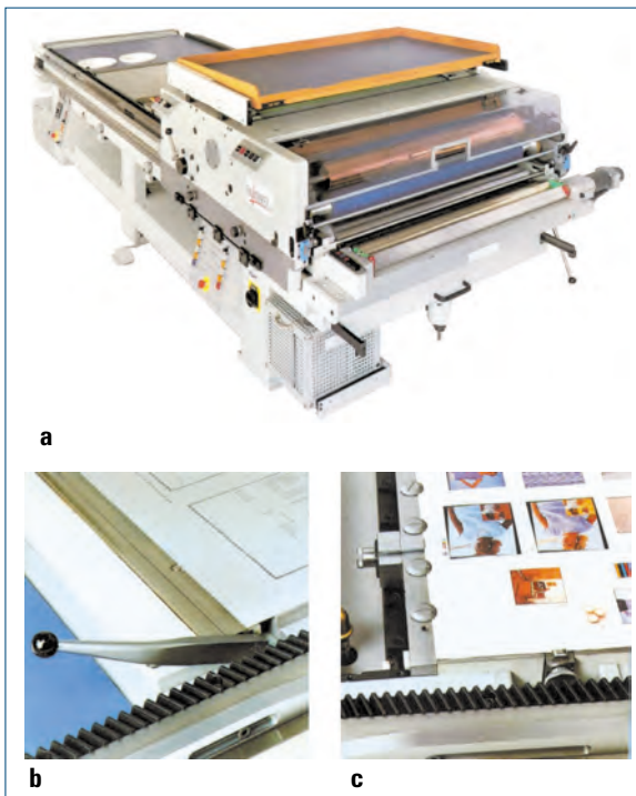
Fig. 3.1-45 Flat-bed offset proofing press (Korrex 2000, FAG). a Proofing press; b Plate fixture on the table; c Printed sheet on the flat-bed table
