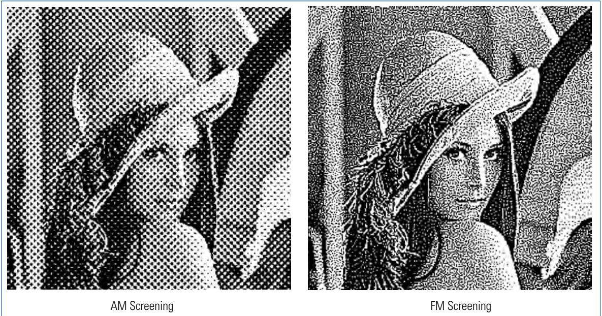
Fig. 1.4-38 Comparison of amplitude-modulated (AM) screening with frequency-modulated (FM) screening (AccuTone, R. R. Donnelley)
