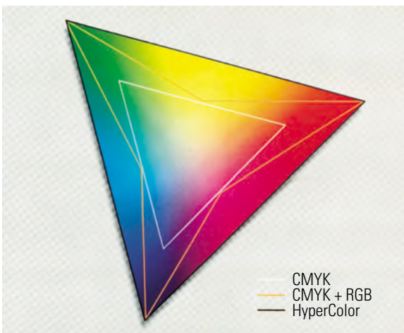
Fig. 2.1-215 High-fidelity multicolor printing (HiFi color) to expand color gamut in offset printing; diagrammatic (HiFi color system: HyperColor, DuPont)
