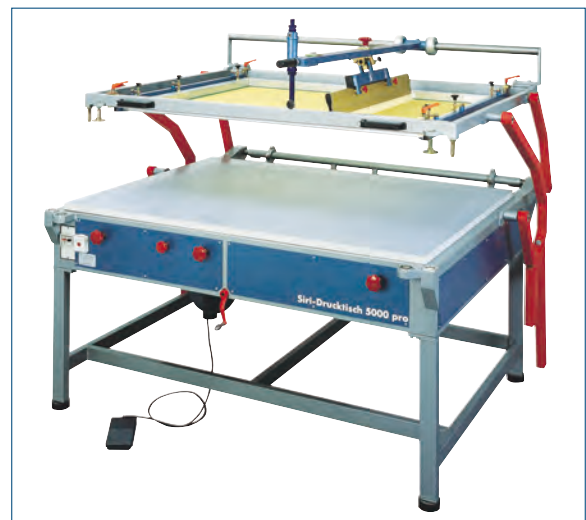
Fig. 2.4-12 Flat-bed screen printing equipment (Siri/Steinmann)
