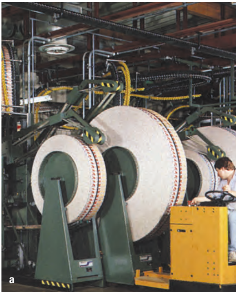
Fig. 7.3-7 Temporary storage for folded sheets on reel storage units (disk).
