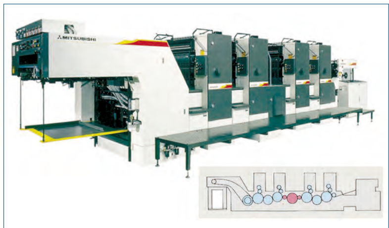
Fig. 2.1-175 Model 3FR-4, 4-color press with sheet reversal for 2/2 printing; sheet size 720 mm × 1020 mm, printing speed 13000/11000 impressions/hour, reduced speed for perfecting (Mitsubishi)
