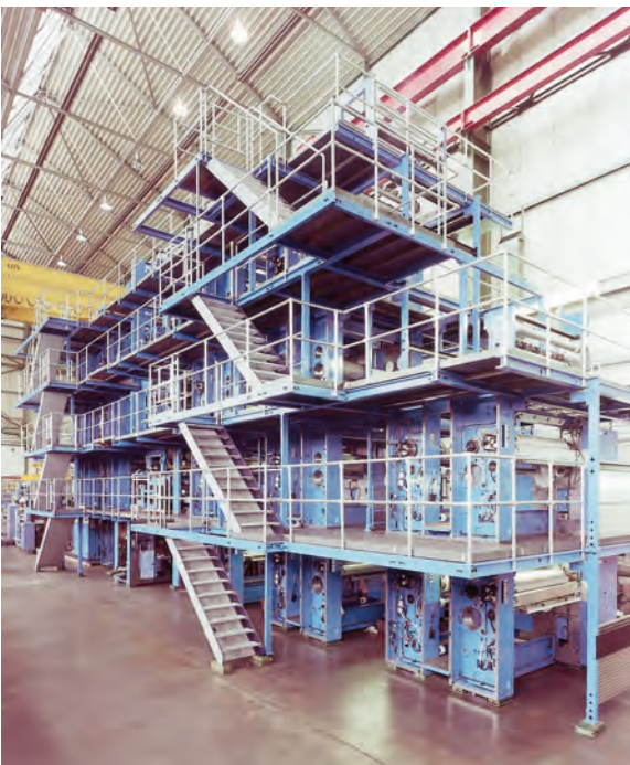
Fig. 2.3-22 Newspaper press for multicolor printing with 144 printing units (Flexocourier, KBA)
