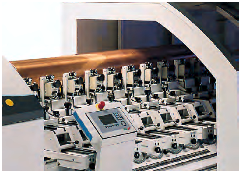
Fig. 2.2-7 Engraving machine for electromechanical stylus engraving with up to 16 engraving heads (HelioKlischograph K 406-Sprint, HELL Gravure Systems)
