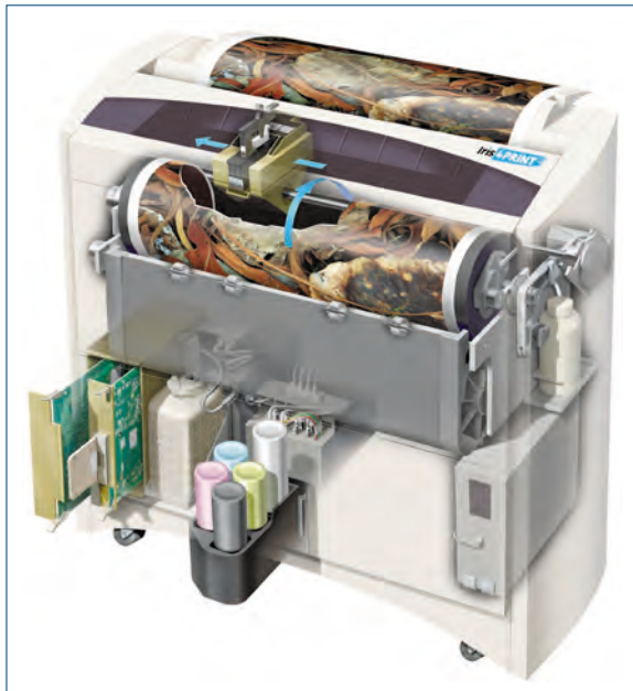
Fig. 3.2-75 Ink jet system for color proofs (Iris 4 Print, Scitex)
