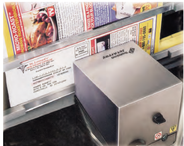
Fig. 5.5-10 Multi-deflection ink jet system for addressing. a Ink jet head for addressing newspapers consisting of four individual systems for writing four lines (Imaje); b Ink jet system for addressing periodicals with six lines during in-line production in web offset printing (Jet Array, Domino)
