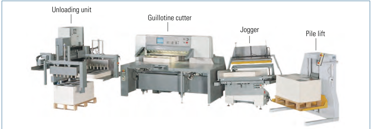
Fig. 7.2-7 Cutting line for cutting printed sheets for medium-sized bookbinding companies (Polar Mohr)
