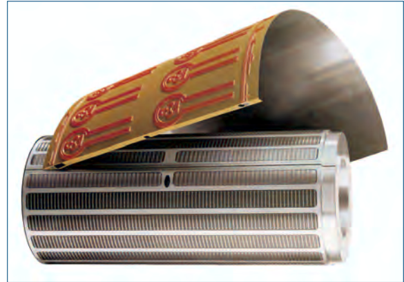
Fig. 2.3-5 Magnetic cylinder with letterpress plate (NELA)
