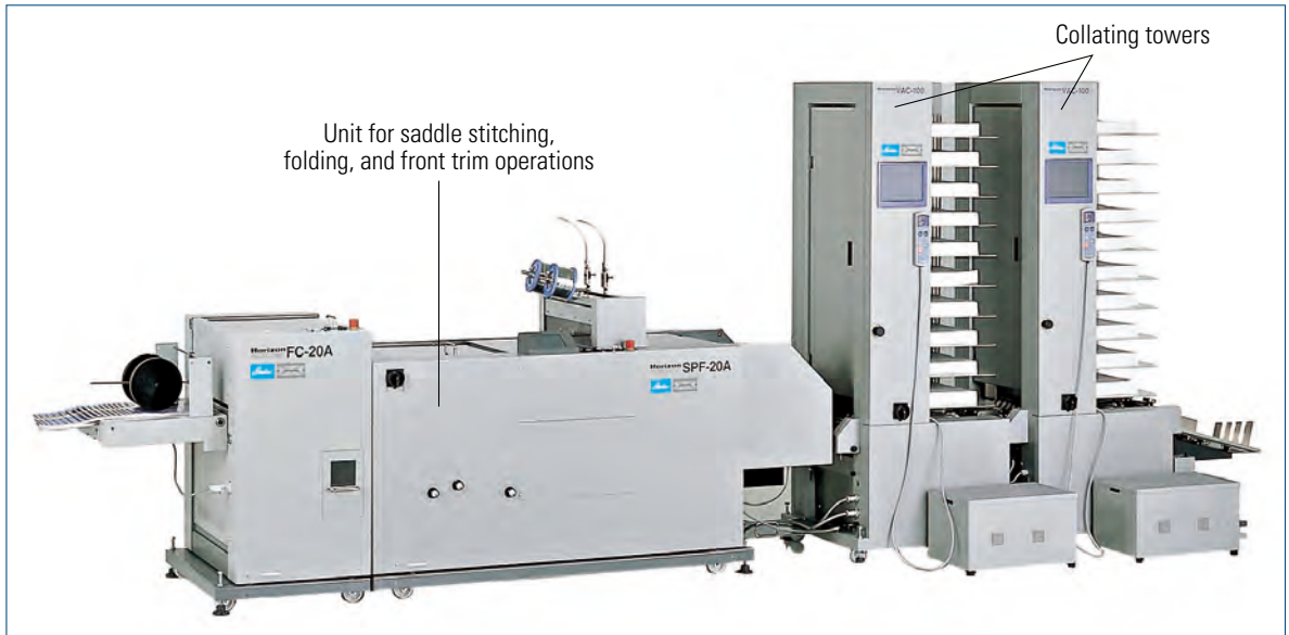
Fig. 7.2-53 Tower collator (vertical feeder arrangement) with further sheet processing (Horizon)
