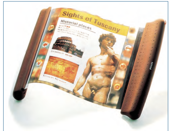
Fig. 12.3-4 Concept study for an Electronic Book with roll-out screen; in this example used as an interactive travel guide (Philips; status: around 1996)
