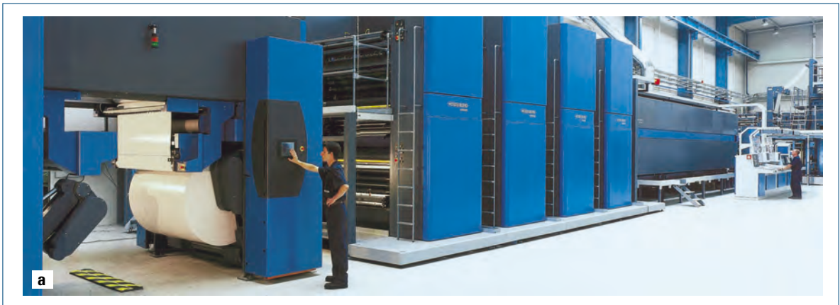
Fig. 2.1-203 a Commercial web offset printing system (48 pages, double-sized cylinders, 50000 revs./hour, max. 100000 copies/hour, web speed 15 m/s) with zero-speed web splicer in horizontal design (M-4000, Heidelberg); b Folder with double stream delivery, copy stream diverters and gathering (PFF-3, Heidelberg)
