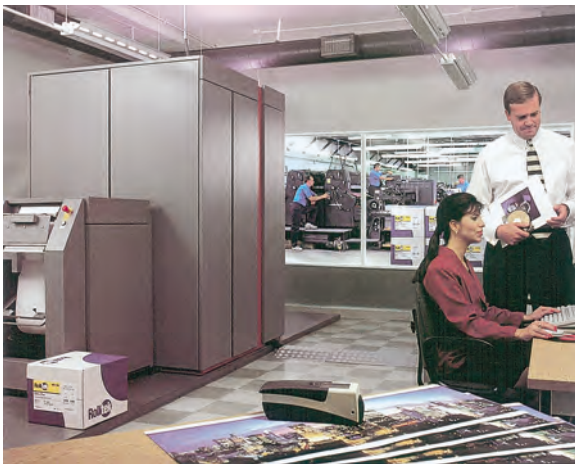
Fig. 9.2-13 Printing company with conventional (offset) and digital (electrophotographic) printing systems (Speedmaster and DCP/32D, Heidelberg/Xeikon)
