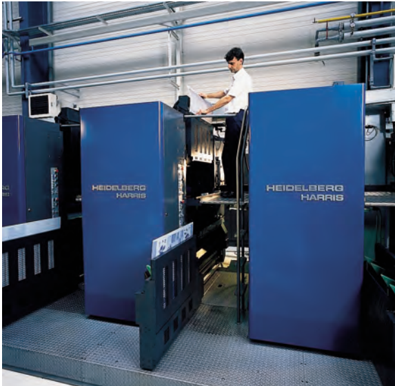
Fig. 2.1-159 Automated printing plate change on a web offset printing system (M-600, Heidelberg)
