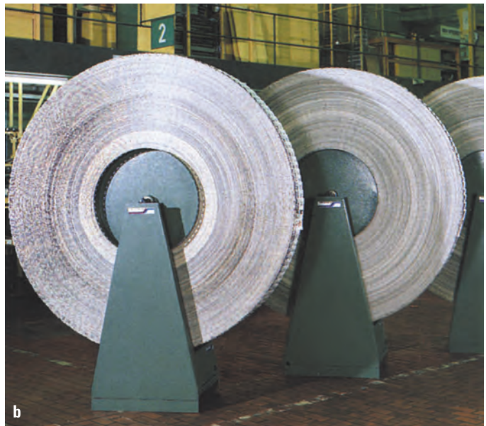
Fig. 7.3-6 Logistics system for folded sheet bundles for producing magazines (Müller Martini)
