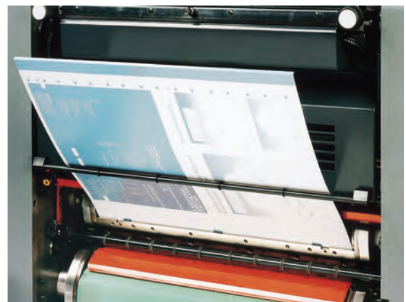
Fig. 2.1-43 Automatic plate loading (Speedmaster SM 52, Heidelberg)
