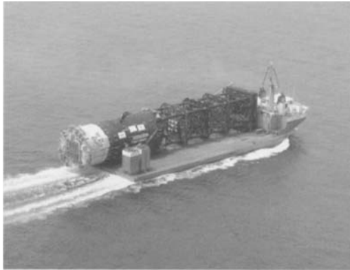
Figure 7.82 Transportation of the spar (Technip Offshore)
