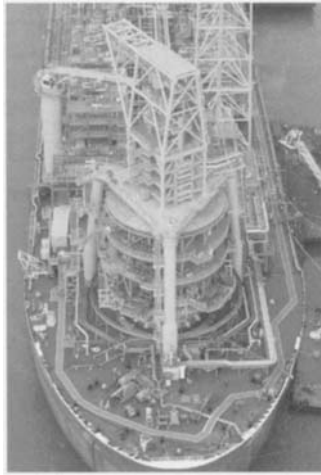
Figure 7.29 Internal bow turret (SBM–Imodco)
