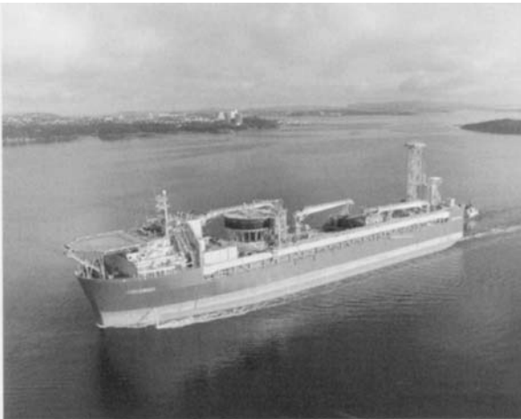
Figure 7.25 Balder FPSO with Turret Midships (ExxonMobil)
