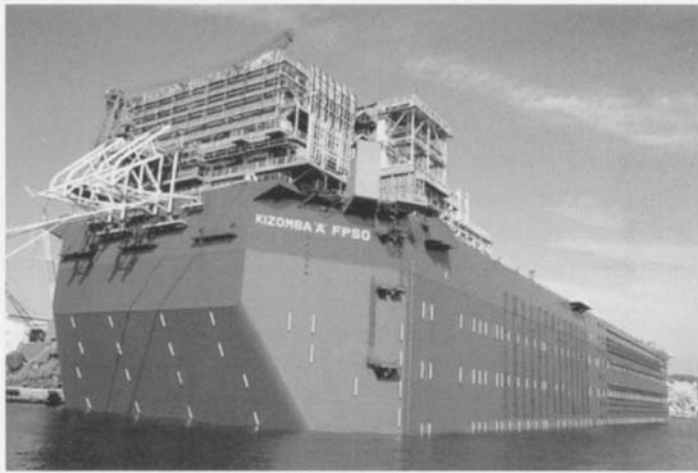
Figure 7.26 Kizomba A, Spread Morred FPSO in West Africa (ExxonMobil)
