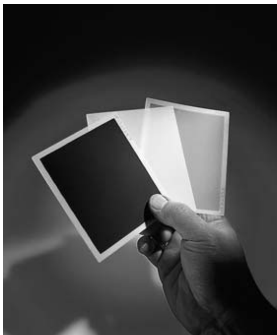
Fig. 20.7 Photograph of planar zirconia electrolyte plates: black cathode, white electrolyte, green anode (grey in picture). (Courtesy of Ceramic Fuel Cells Inc.)
