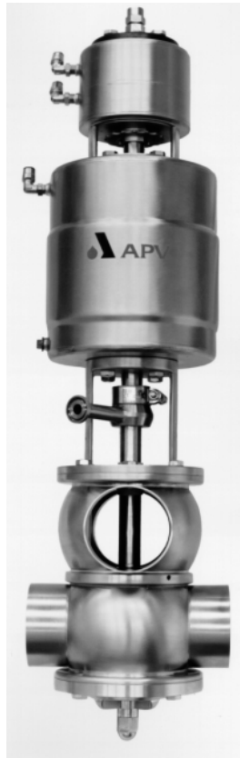
FIGURE 15.11 This mix-proof valve is equipped with a seat lifter module (top) and a vent cavity CIP supply (center). Any leakage due to failure of either of the valve sealing rings will be to atmosphere through the full size leak port, rather than from one fluid to the other. (Courtesy APV.)
