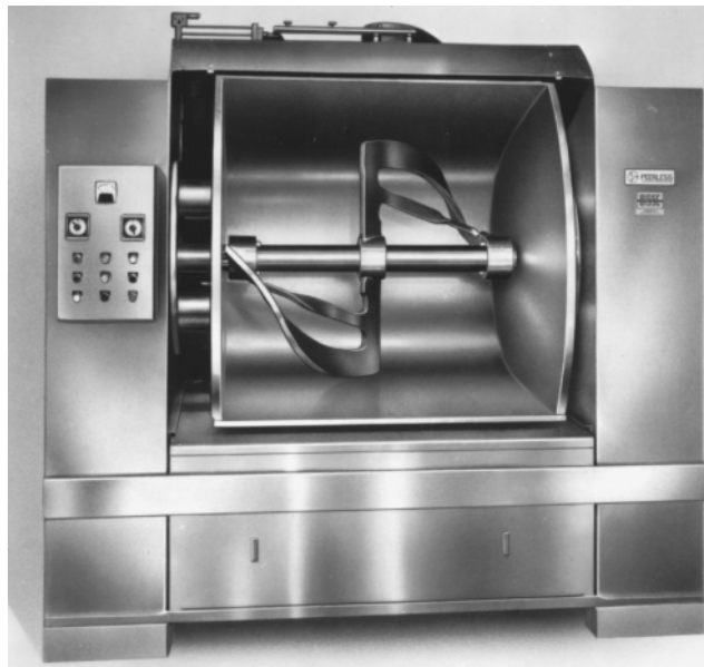
FIGURE 12.9 A single spiral mixer. (Courtesy of Peerless Manufacturing Corp., Sydney, OH.)
