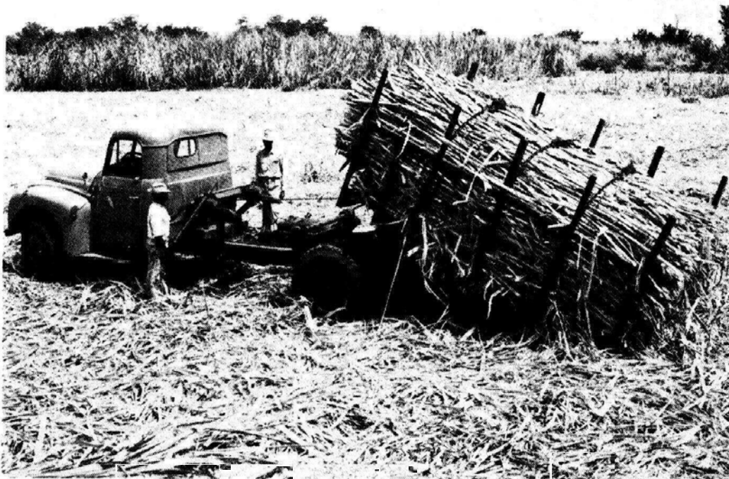
Fig. 1.4. Cane transport by detachable container (loading in field)
