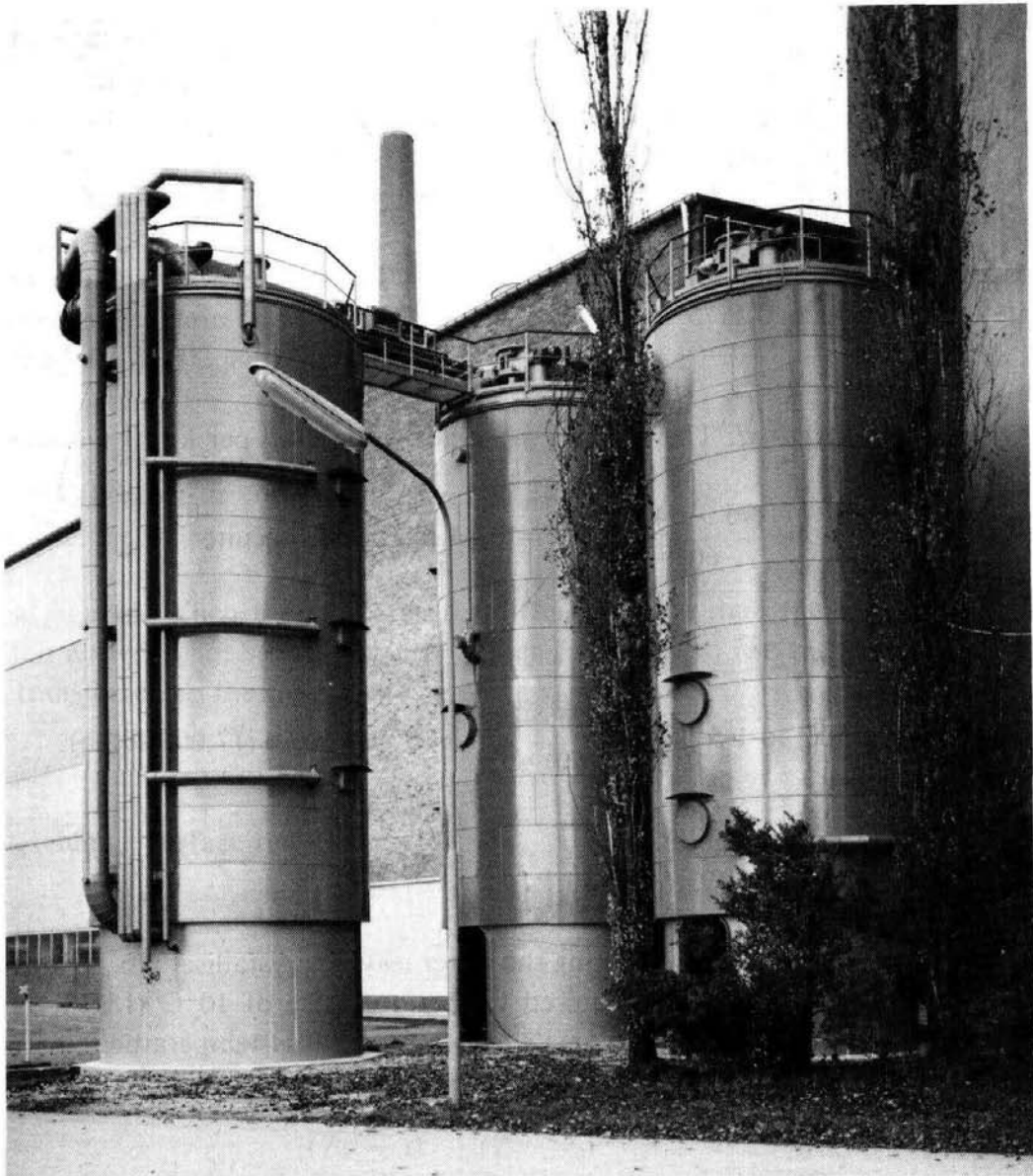
Fig. 34.12 Series of three vertical crystallisers (B.M.A.).
