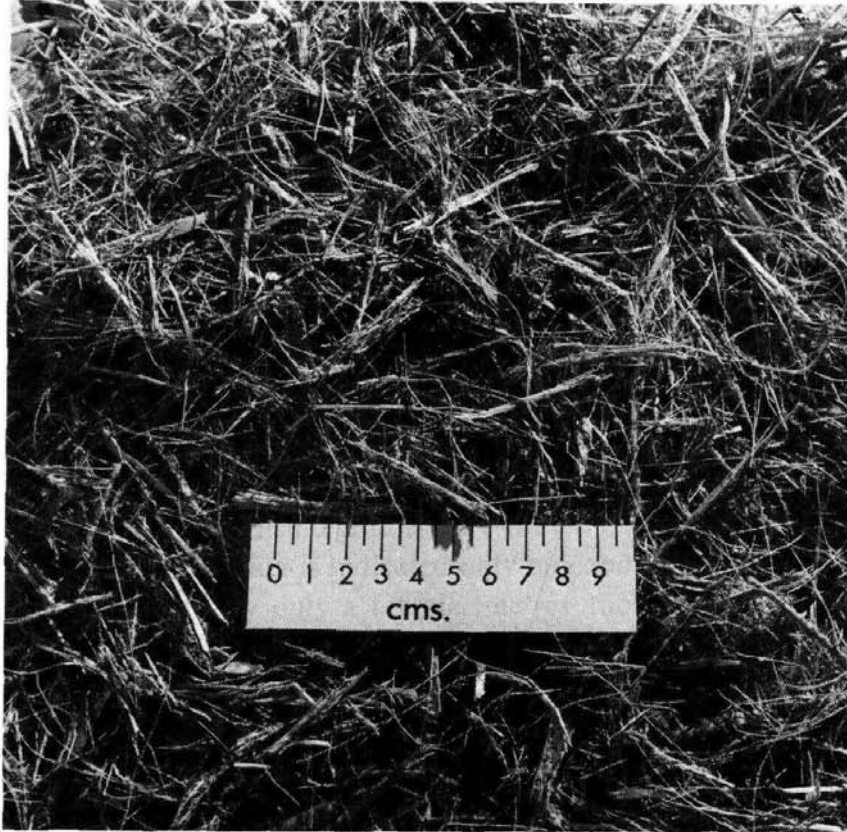
Fig. 6.9. Shredded cane (photo Gruendler).
