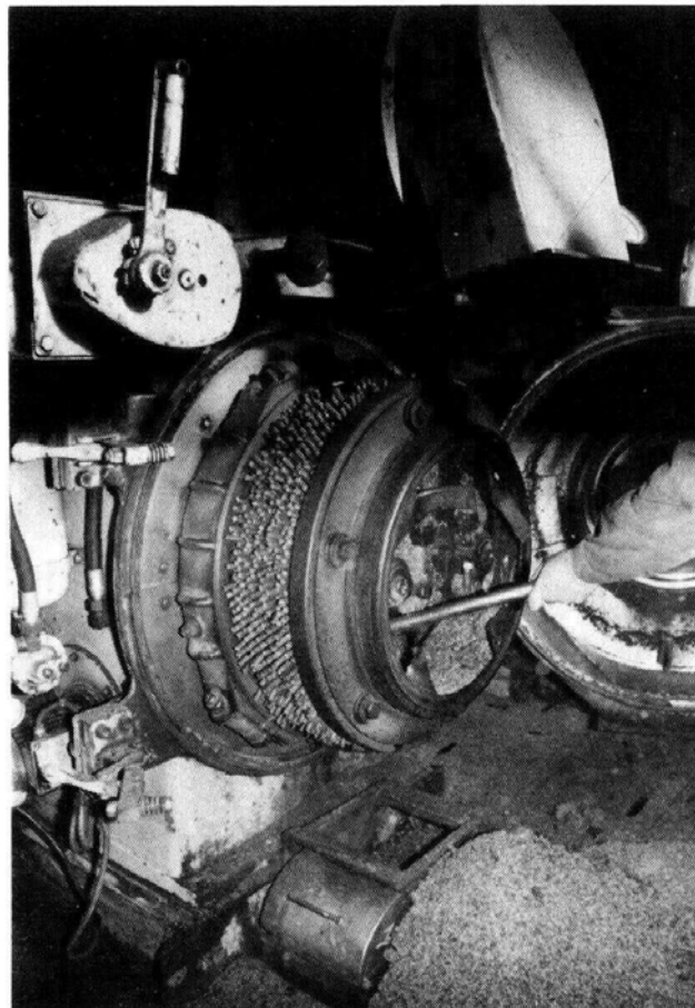
Fig. 41.39. "C.P.M." pellet mill open for cleaning.
