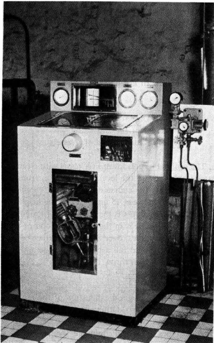
Fig. 32.25. Cabinet for brix and evaporator control (Babcock Atlantique).
