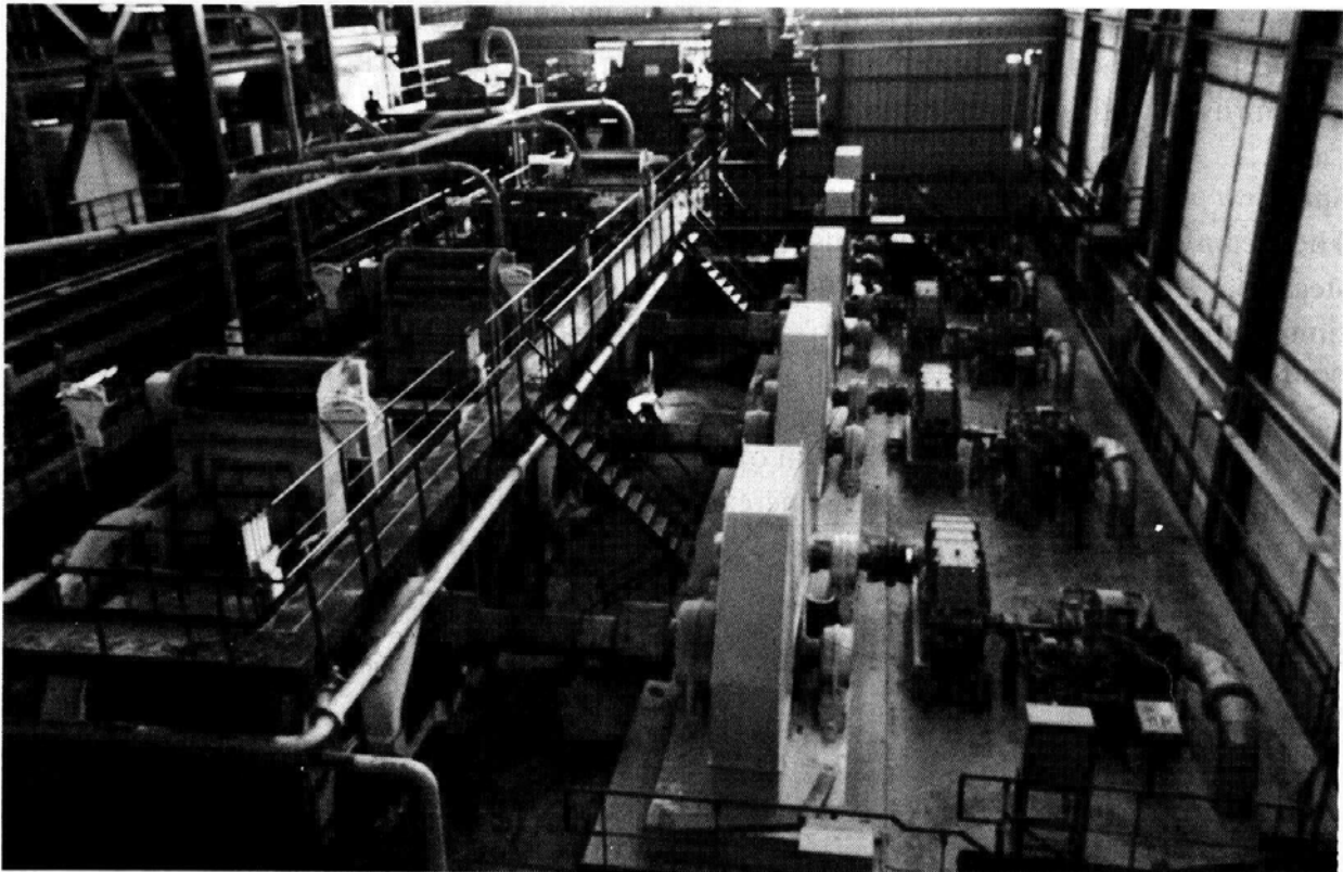
Fig. 16.3. Mill tandem driven by steam turbines.
