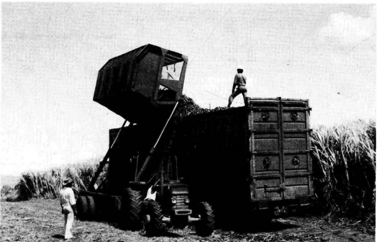
Fig. 1.14. Loading canes in billets Legras trailer.
