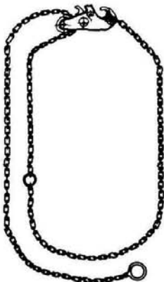
Fig. 1.1. Sling with automatic hook.
