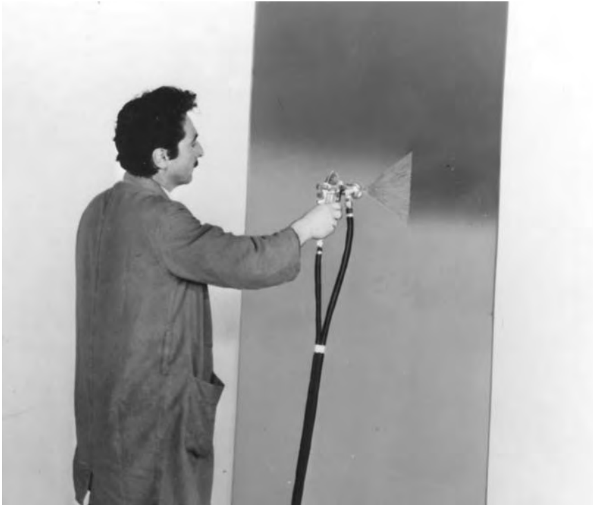
Figure 20: Manual air spray (source Kremlin).
