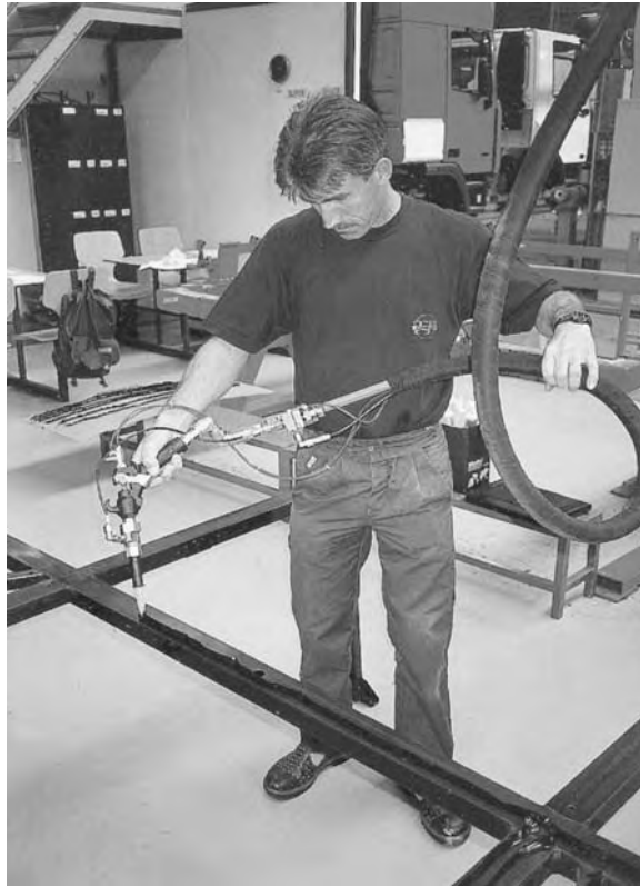
Figure 78: Application of adhesive (see colour plate section).
