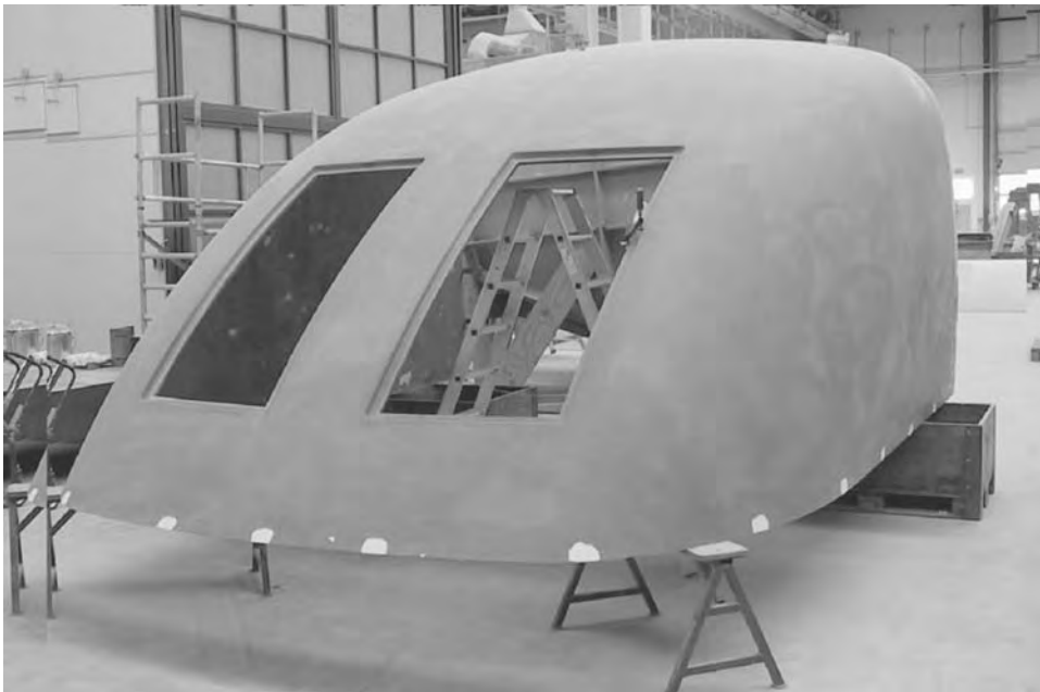
Figure 5: GRP front module of 'Transrapid'.
