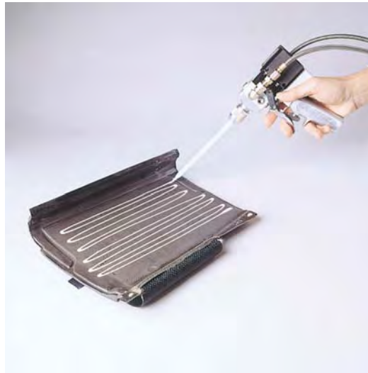
Plate 16: Application of adhesive in bead form on a plastic part with hand held gun equipped with a static mixer (source Graco, Belgium/USA).
