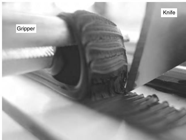
Figure 22: Peeling test of a bead.
