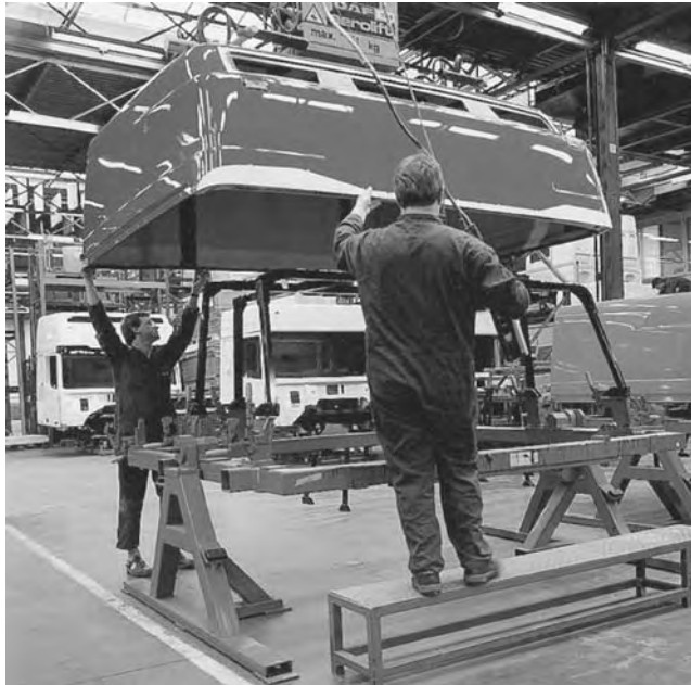
Figure 79: Lowering the GRP roof shell onto the steel frame.
