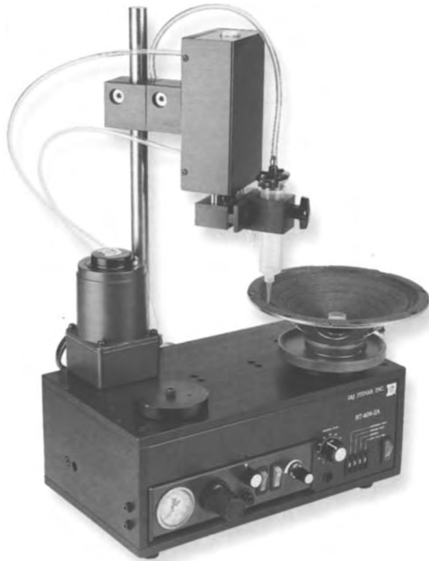
Figure 89: Bonding loudspeaker with rotation table RT404 from IJ, Fisnar, USA.
