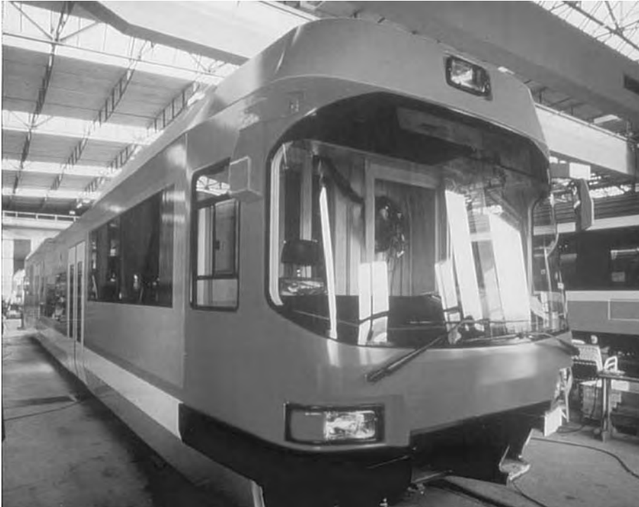
Figure 4: (continued) (b) Direct glazed front cabin bonded to the train.
