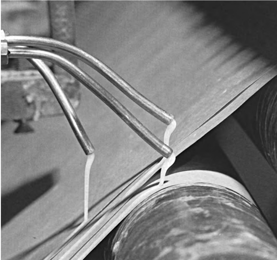
Figure 4: Viscosity of the adhesive must be adapted to the dispensing equipment. Here we show a very simple although automatic way for applying beads of starch glue on each side of a paper roll for bag manufacturing.
