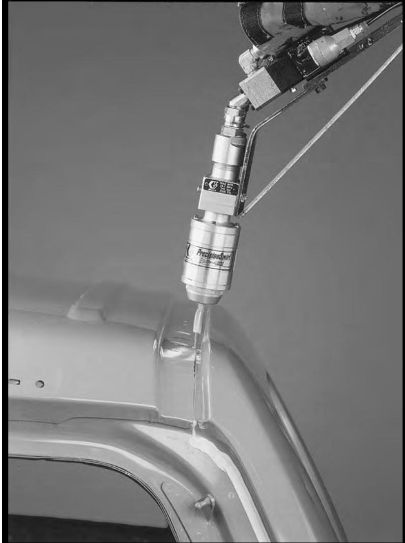
Figure 32: Graco Swirl spraying with 'Precision Swirl' gun on the roof of an automotive (source Graco Belgium).
