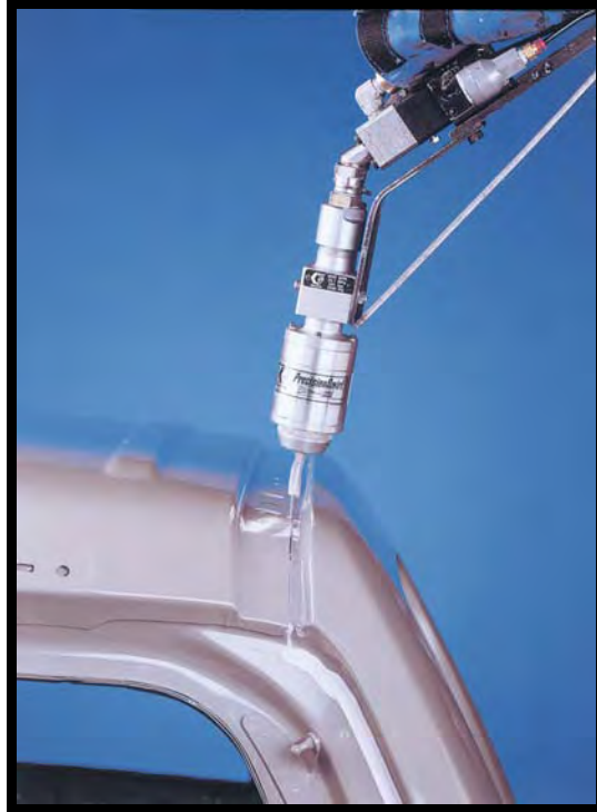
Plate 9: Graco Swirl spraying with 'Precision Swirl' gun on the roof of an automotive (source Graco Belgium).
