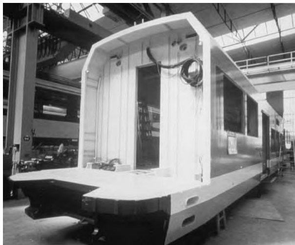
Figure 4: Modern trains owe their stylish looks to a combination of glass, plastics and lightweight metals bonded together with adhesives. (a) Train before cabin bonding.
