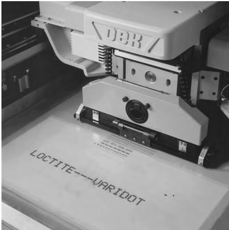
Figure 66: Varidot applicator for rotary screen printing (by courtesy of Loctite).
