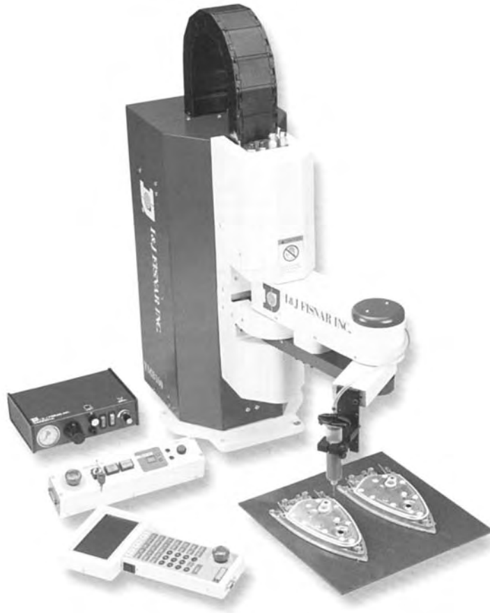
Figure 10: Robotic application with syringes.
