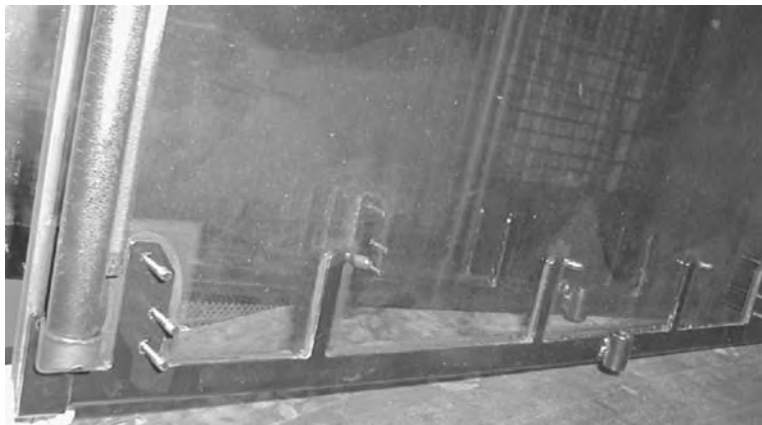
Figure 57: Lifting bar for side window bonded to glass with Sikaflex®-360 HC within 20 min at 120°C.
