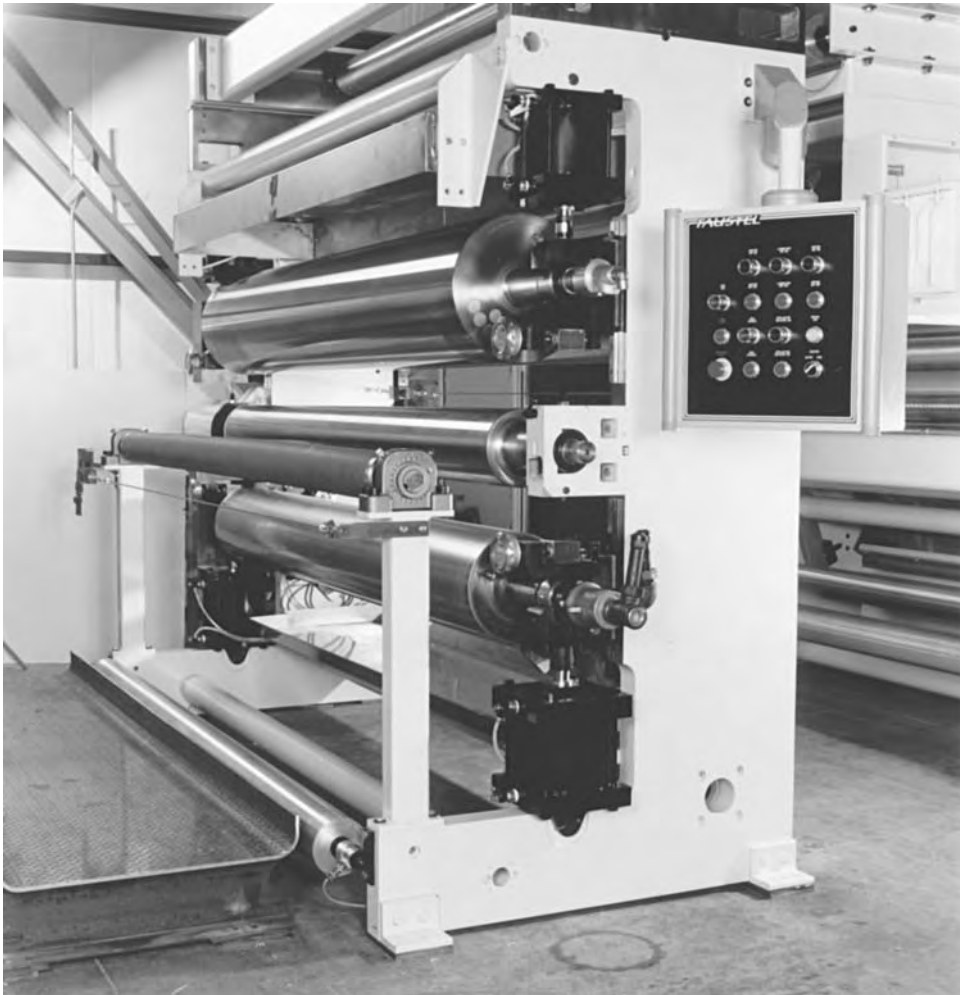
Figure 3: Roll coater for laminating unit (by courtesy of Faustel USA).
