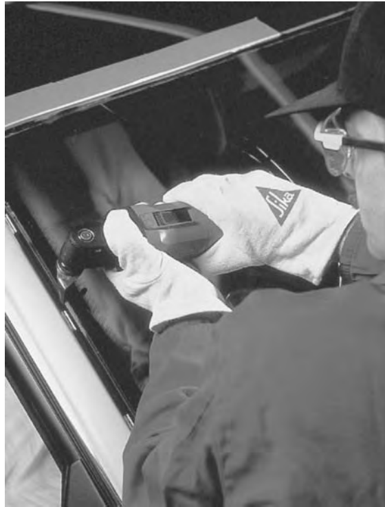
Figure 100: Removing an adhesive-bonded windshield.
