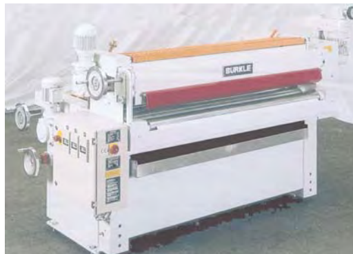
Plate 10: Roller Coater (by courtesy of Bürkle Germany).
