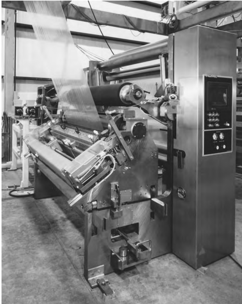
Figure 55: Cartridge style coater showing a slot die coating cartridge – mainly used for water based PSA adhesive (source FAUSTEL Inc. USA).
