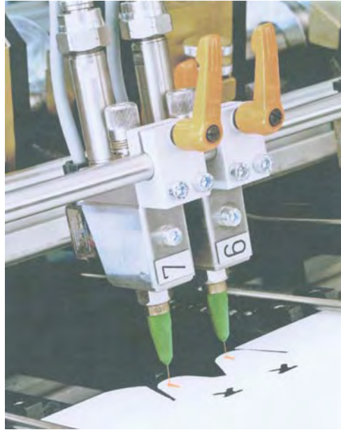
Plate 15: Needle applicator for cold glue (source Robatech Switzerland).
