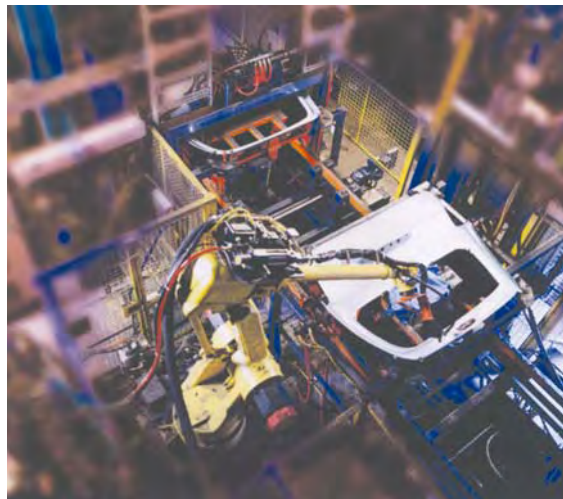
Plate 18: Robotic application of a structural adhesive on an automotive production line (source Graco).
