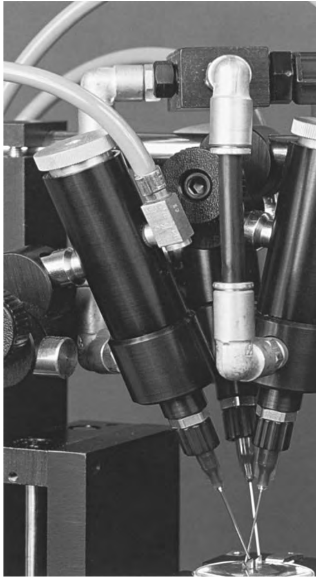
Figure 7: Syringe application. Three 740V-SS valves from EFD (USA) dispense microdots of UV curing adhesive on the lens of a barcod scanner (source EFD/USA).
