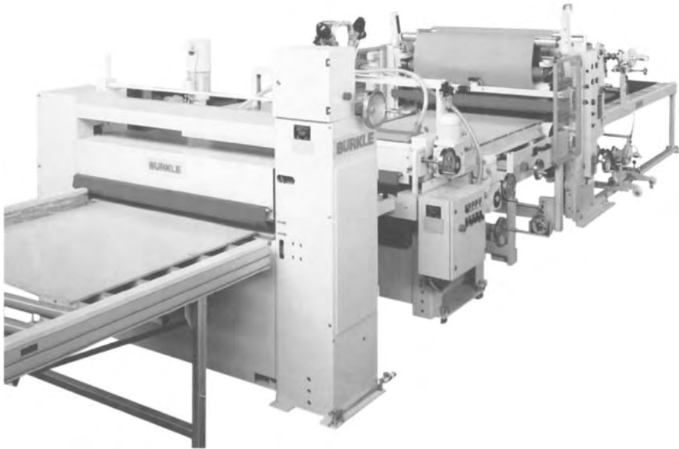
Figure 52b: Bürkle EFA 12 laminating machine (by courtesy of Bürkle Germany).
