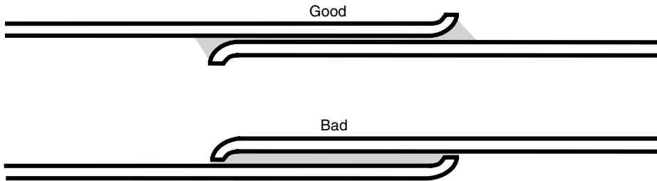
Figure 38: The joint ends have improved design if the glue line thickness increases in this high stress area.
