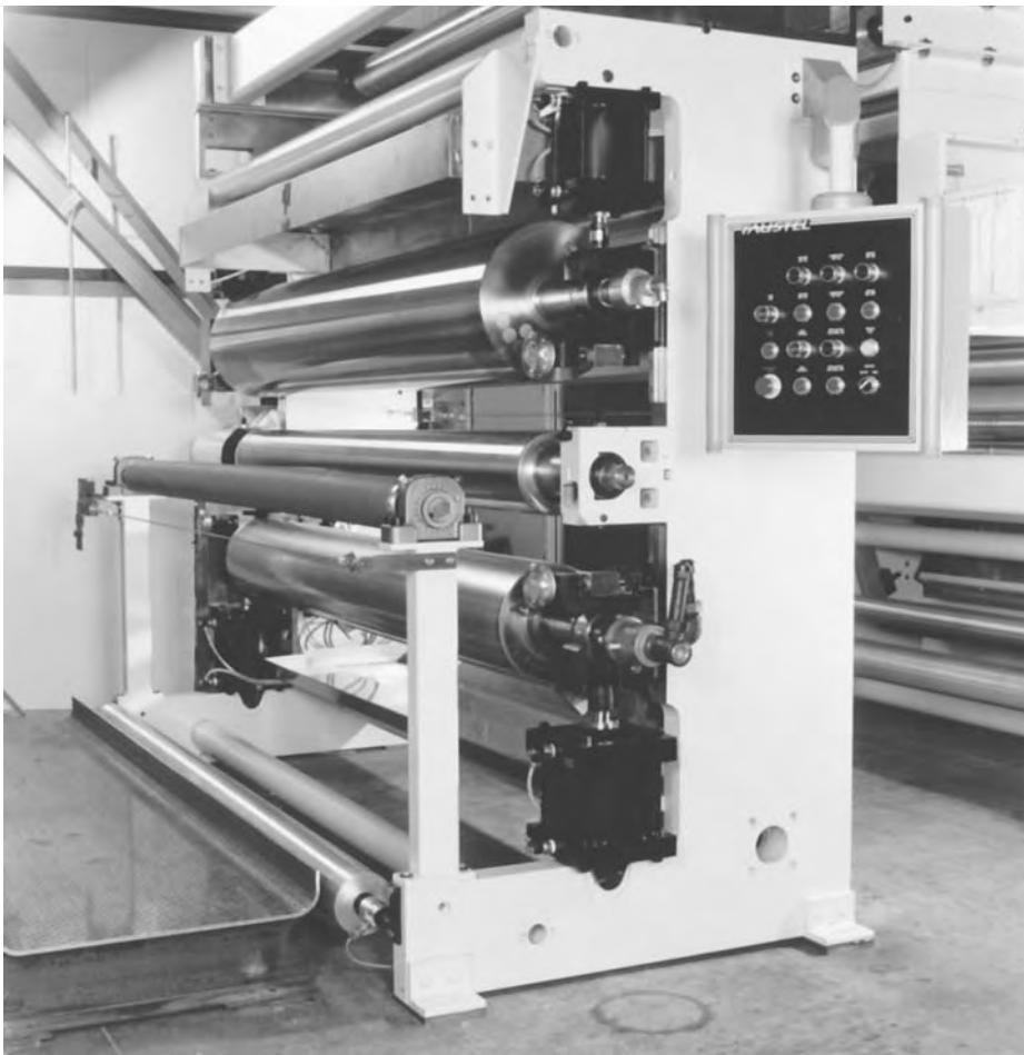
Figure 51: Faustel Roll Coater (source Faustel USA).
