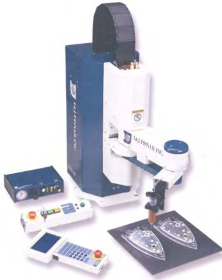
Plate 17: Robotic application of silicone adhesive/sealant on Fisnar robot equipped with syringes of adhesive/sealant (robot Scara TMB 100).
