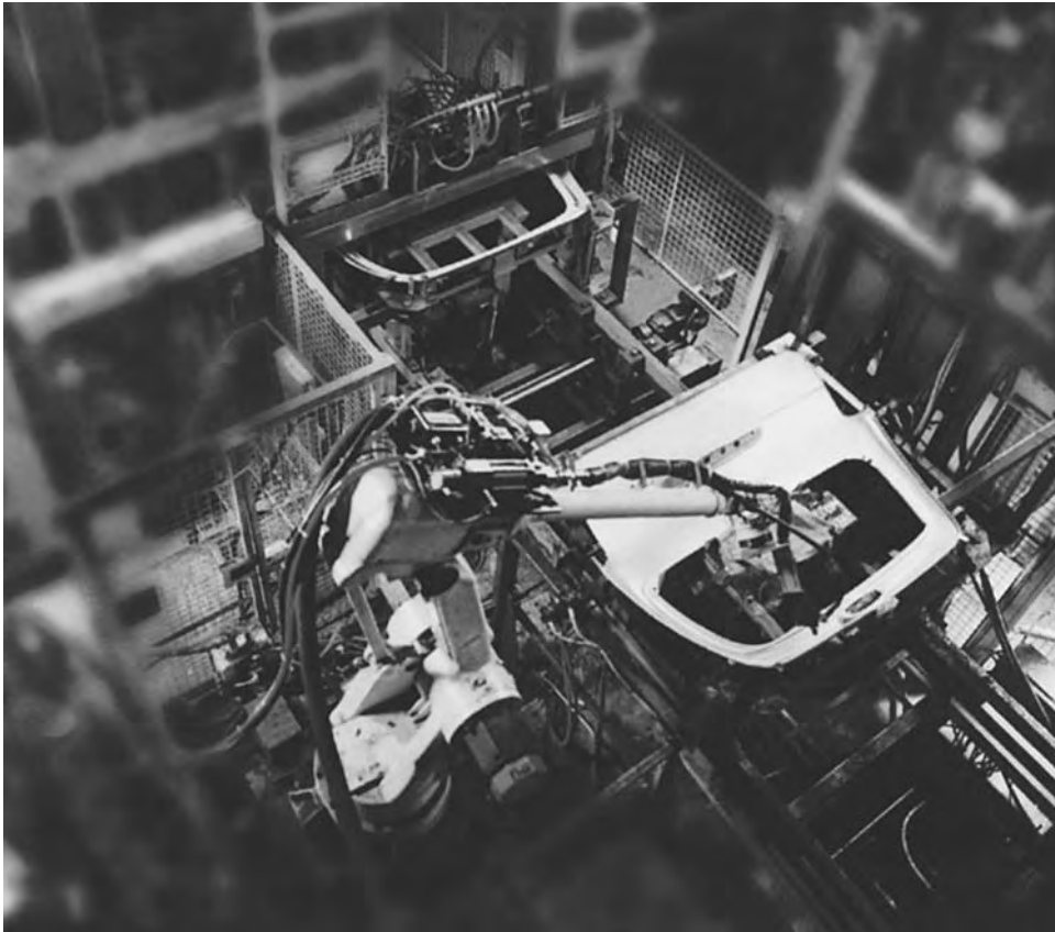
Figure 91: Robotic application of a structural adhesive on an automotive production line (source Graco).
