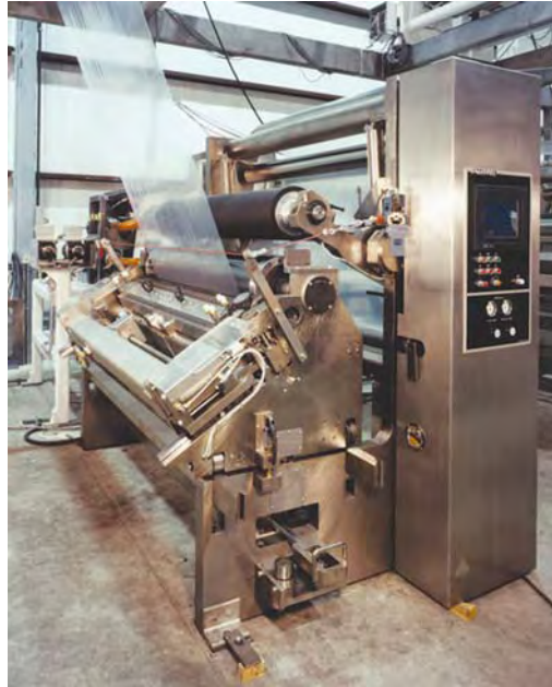
Plate 13: Cartridge style coater showing a slot die coating cartridge – mainly used for water based PSA adhesive.
