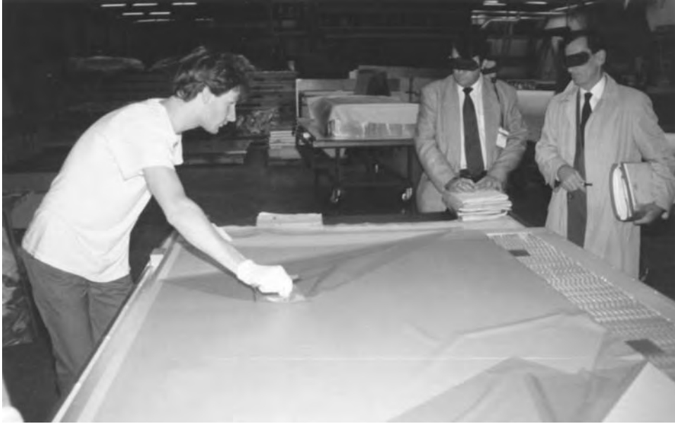
Figure 92: Hand lay down of a structural thermosetting epoxy adhesive film.
