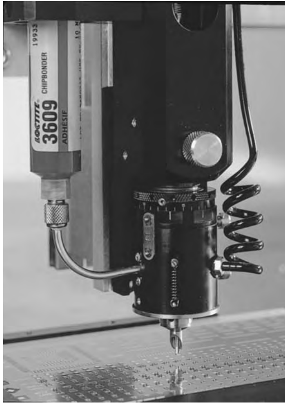
Figure 90: High speed adhesive application with small cartridges (by courtesy of LOCTITE, USA).
