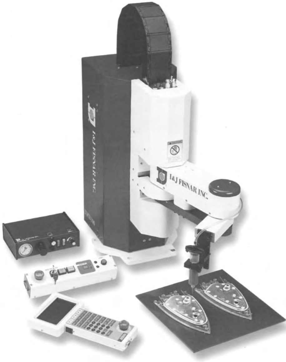
Figure 88: Robotic application of silicone adhesive/sealant on Fisnar robot equipped with syringes of adhesive/sealant (robot Scara TMB 100) (by courtesy of FISNAR, USA).
