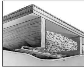
Wood-frame—with resilient attachment and THERMAFIBER SAFB.
