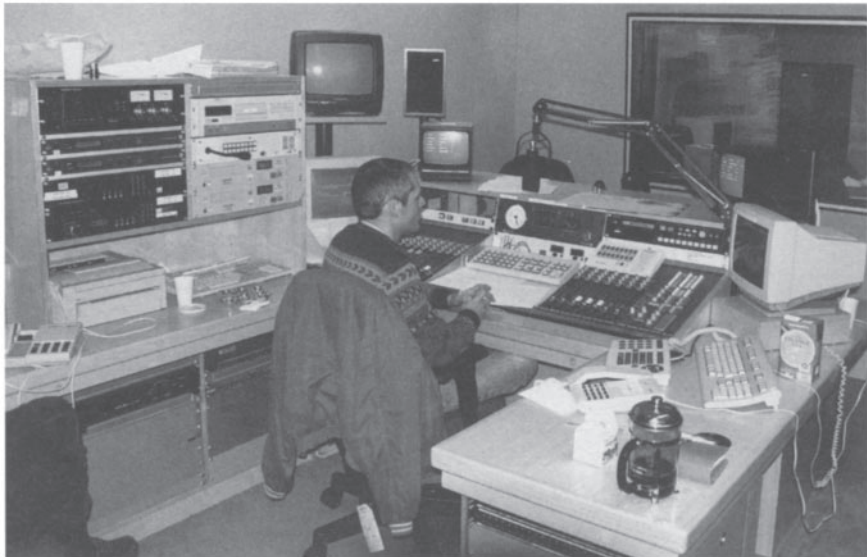
9: The control room of London's most popular talk station, LBC, which was Britain's first independent radio station. This photograph was taken when the weekend breakfast programme was being produced, with the producer Steve Campen in the studio. The control room reverts to a self-drive studio for most of the day's programming. LBC use D-Cart for news reports and features, DCS (Digital Commercial System) for adverts and jingles, mini-disc for longer pre-recorded programmes and compact disc for music. The tape recorder is redundant.
