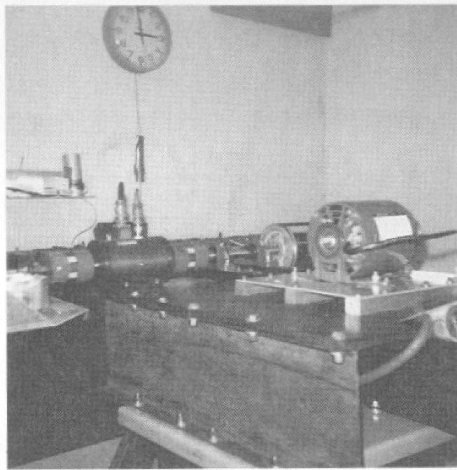
FIGURE 18.14 Torquemeter placed between the electric motor and the test fan, with bearings and flexible couplings on each side. (Courtesy of FloAire, Inc., Bensalem, Pa.)
