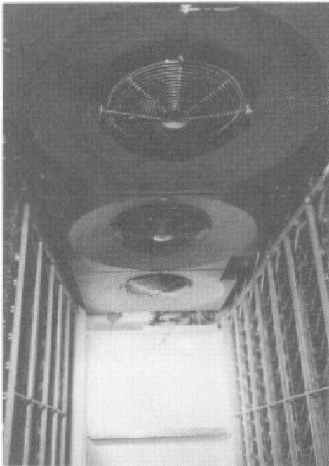
FIGURE 12.4 Inside view of an incubator showing the egg carriers on each side of the center aisle and some fans at the top. (Courtesy of Chick Master Incubator Company, Medina, Ohio.)
