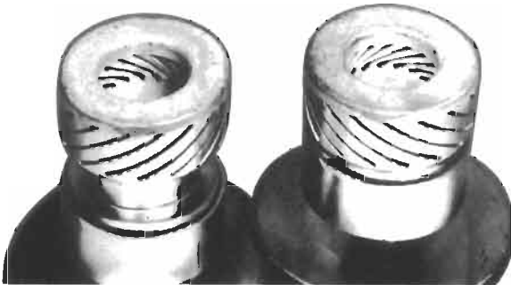
(a) Slotted cup type contacts of a 7.2 kV, 25 kA vacuum interrupter (Axial magnetic field type) (Courtesy: Siemens)
