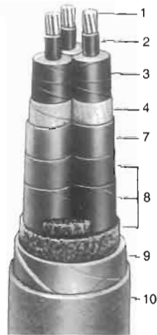
Screened SL construction (HSL type) which, in addition to possessing its own insulation and screen also has a separate lead sheath for each core as against a common lead sheath in the other two types
