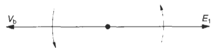
(c) When E'_1 = V_b , E_c = 0 and I_c = 0 , G_1 floats on the bus
