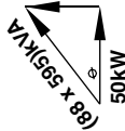
Figure 1-30 Solve for power factor in a one-phase circuit when voltage, current, and true power are known.
