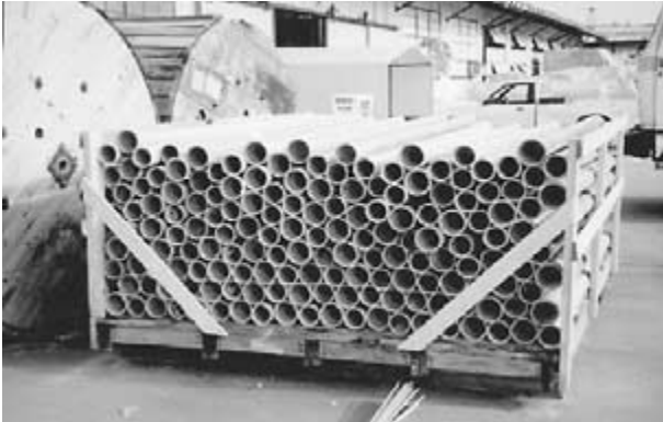
PVC conduit stored for future installation to take advantage of volume discounts that exceed the time value of money costs.
