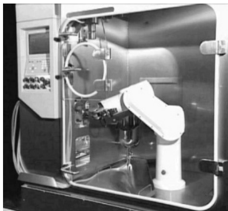
Figure 13.12 Automated infrastructure for bulk production of cellular reagents for HTS. The Cellmate (The Technology Partnership, Cambridge, UK). The Cellmate can reform bulk production of up to 500+ flasks, 1–2 cell lines/day and cell harvest by scraping. Unattended operation of the Cellmate is made possible with the addition of the Flaskmaster (BMS) to feed flasks into and out of the instrument.
