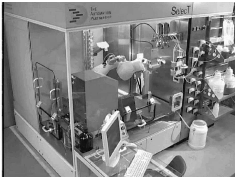
Figure 13.13 The SelectT (The Technology Partnership, Cambridge, U.K.). A fully automated cell culture system performs routine maintenance of up to 50 cell lines per day. It manages growth, incubation, and routine passaging of multiple cell lines with unattended operation. The SelectT performs cell counting, viability measurements, and cell plating into microtiter plates.
