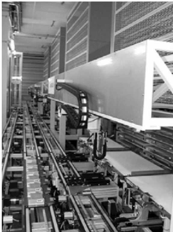
Figure 13.6 Photo of Haystack (The Technology Partnership, Cambridge, UK). The haystack compound storage system at Bristol-Myers Squibb showing the “wet” tube store.
