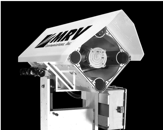
Figure 3. Photo of 0.785- \mu\text{m} -wavelength diode laser FSO system from Optical Access that uses Four laser beams to reduce speckle fading and atmospheric turbulence effects.
