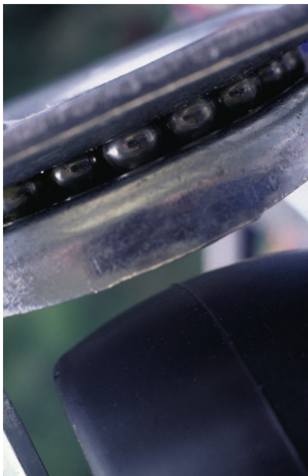
Chair castor showing ball bearings made of palladium alloys. Photograph by Robert J. Huffman. FieldMark Publications . Reproduced by permission.
