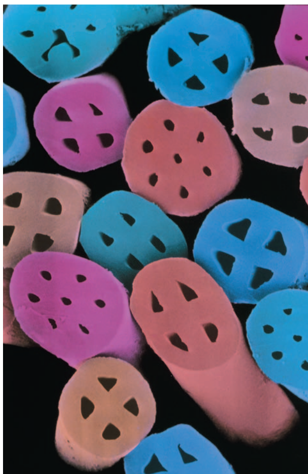
A scanning electron micrograph (SEM) of fibers of a dacron polyester material used in sleeping bags. The core of each fiber has up to seven air cavities that increase its insulating ability. Photograph. Science Photo Library/National Audubon Society Collection/Photo Researchers, Inc. Reproduced by permission.
