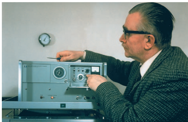
Repairs completed to an atomic clock. This clock is timed to the resonance frequency of cesium. Royal Greenwich Observatory, National Audubon Society Collection/Photo Researchers, Inc. Reproduced by permission.
