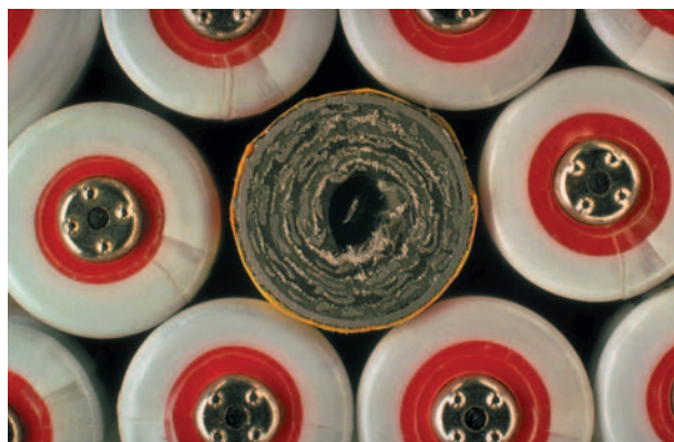
A collection of batteries seen from above, with the top of the center battery cut away to show the interior. This type of battery, a dry version of the LeClanche cell, is called a carbon-zinc primary cell. A carbon rod sits upright in the center and acts as a cathode (negative electrode). The outer vessel is made of zinc, which allows it to serve as both a container and as an anode (positive electrode). The electrodes are in contact with a moist electrolytic paste (the grey material that fills the battery) consisting of ammonium and zinc chlorides, manganese dioxide and carbon particles. © Dr. Jeremy Burgess/Science Photo Library, National Audubon Society Collection/Photo Researchers, Inc. Reproduced with permission.
