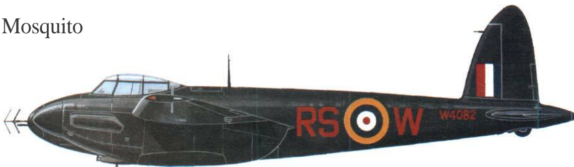
W4082 was the fifth production Mosquito MkII, delivered in January 1942. Note the exhaust flame dampers, which reduced flight performance.
