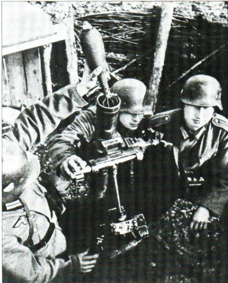
The shape of the 8-cm sGrW34 bomb can be clearly seen here as it is held ready for loading into the muzzle. The bomb weighed 3.5 kg (7.72 lb) and used multiple tailfins to provide stability in flight. The layer is making fine traverse adjustments using the simple sight mounted on the bipod.
