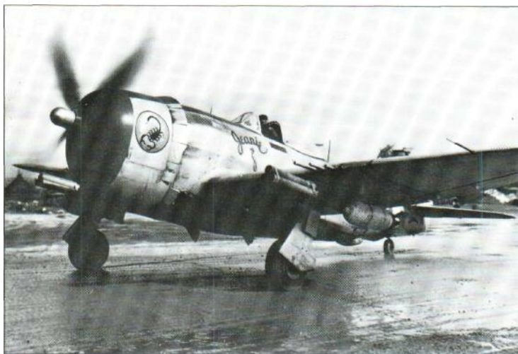
This 12th Air Force P-47 in Italy demonstrates the three main weapons of the wartime fighter-bomber, namely machine-guns, bombs and rockets. Such aircraft were the workhorses of the Allied drive up the Italian mainland.
