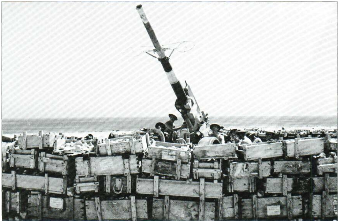
Below: A 3.7-in (94-mm) gun sited in a desert sangar formed by filling old Italian ammunition boxes with stones. The barrel is fitted with makeshift sights as the gun was no doubt operating away from its normal position.
