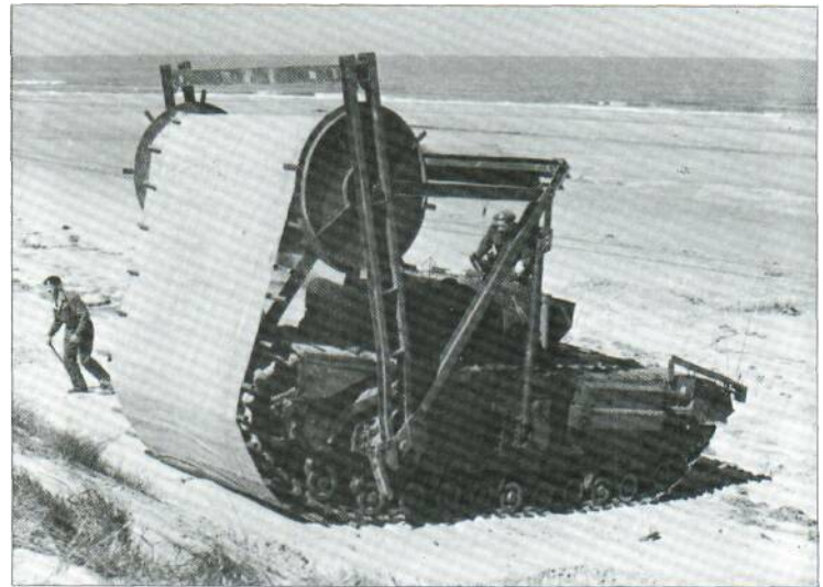
A Churchill AVRE operates a Carpet-Layer Type C, used to lay a continuous hessian mat over rough or soft ground to enable other wheeled or tracked vehicles to follow. These devices were used to cross the sand on some of the Normandy beaches on 6 June 1944.
