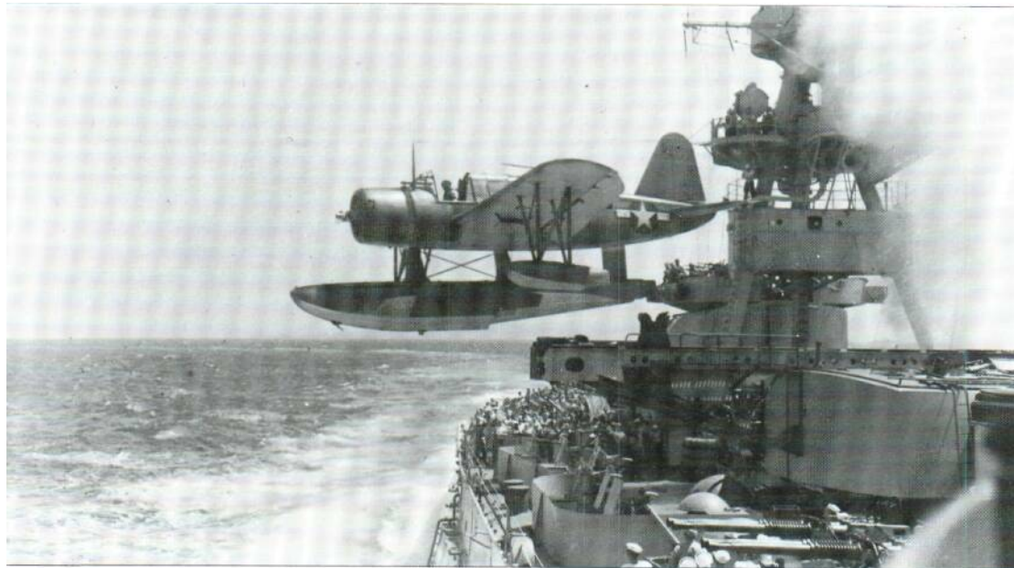
A Kingfisher catapults from USS Texas in the Mediterranean, 1944. Texas was the first US battleship to launch aircraft after being fitted with a flying-off platform while serving with the British Grand Fleet in 1918.
