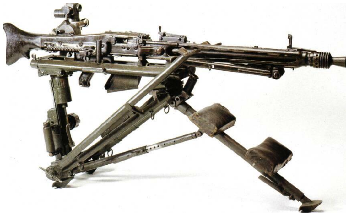
Above: An MG 42 mounted on the Lafette 42 for the heavy machine-gun role; this heavy tripod could be quickly adapted for the anti-aircraft fire role.
