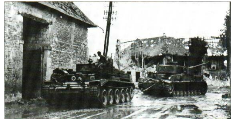
A Cromwell ARV (Armoured Recovery Vehicle) is used to tow a captured German PzKpfw IV tank out of the way of other vehicles. The Cromwell ARV was a turretless conversion of an early mark of Cromwell tank that could be fitted with a jib crane and other gear.
