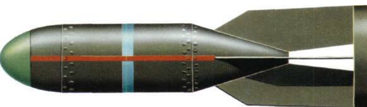
The Type 97 no. 6 59-kg bomb was a general-purpose weapon carried by a variety of Japanese aircraft, from heavy bombers to fighters.
