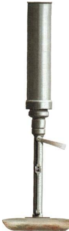
The Japanese 50-mm (1.97-in) Grenade Discharger Type 10 was first produced in 1921 and later replaced by the improved Type 89. With a limited range (160 mil 75 yards), it remained a light and handy weapon that could fire a range of HE, smoke and flare grenades.
