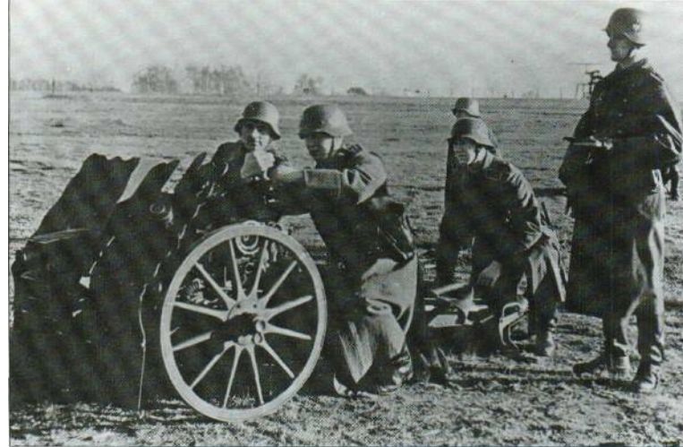
A 7.5-cm leIG 18 is loaded, an unusual procedure where operation of the breech lever raised the rear end of the barrel upwards in a slipper to expose the chamber; the breech block remained fixed. This gun has spoked wheels for horse traction, while later models had metal wheels with rubber tyres.
