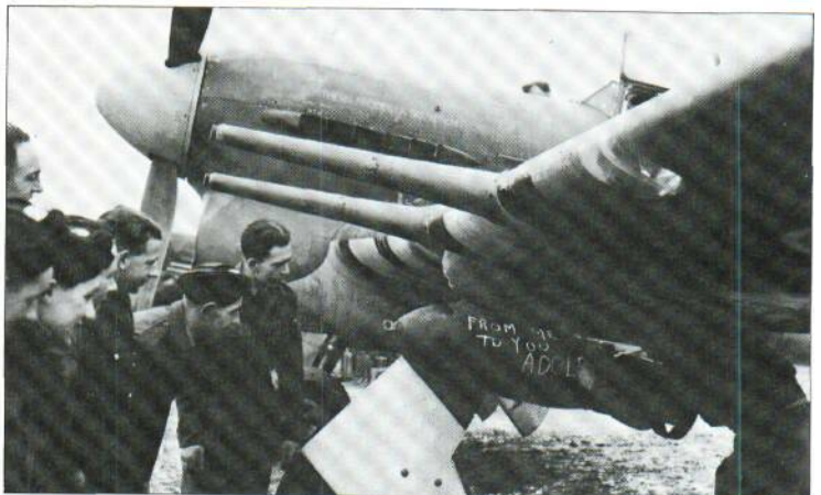
A 227-kg (500-lb) Mk III MC bomb is loaded on the wing rack of a Hawker Typhoon. The pistol and detonator has not yet been installed in the nose of the bomb; the armed bomb had pistols and detonators in both nose and tail.
