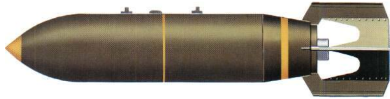
The 454-kg (1,000-lb) armour-piercing bomb used by the USAAF was a thick-cased weapon with an explosive filling to weight ratio of only 14 per cent.
