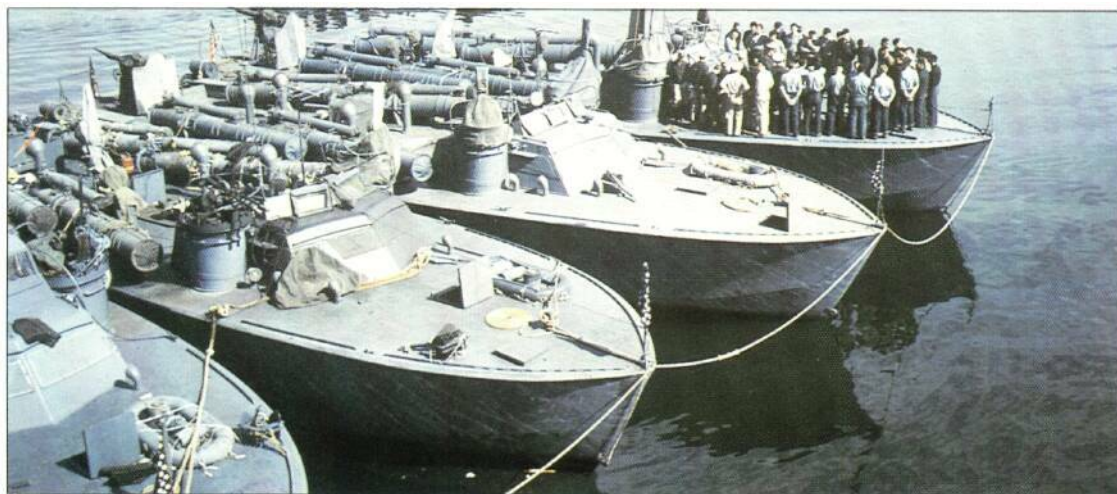
Initially the secondary armament on PTBs was limited to 12.7-mm (0.5-in) MGs, but before long heavier weapons, such as stern-mounted 20-mm cannon, began to be fitted.
