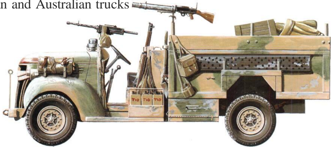
Above: A 1940 Chevrolet WA is seen in the configuration developed by the LRDC for their operations in North Africa. The vehicle illustrated carries a Lewis gun behind the cab and a Browning .30 cal M1919 with AA barrel above the dashboard.
