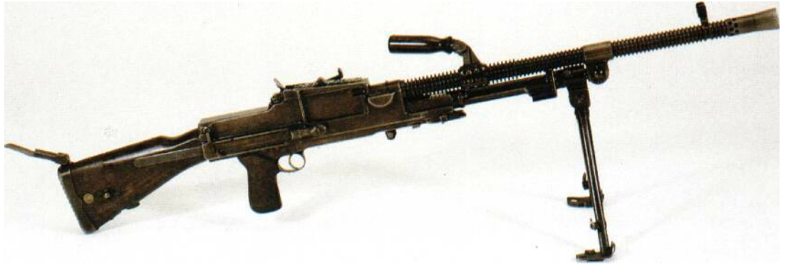
Above: The Czech ZB vz.26, one of the most influential designs of its day and the forerunner of the British Bren gun; this example has its straight 120- or 30-round box magazine missing.
