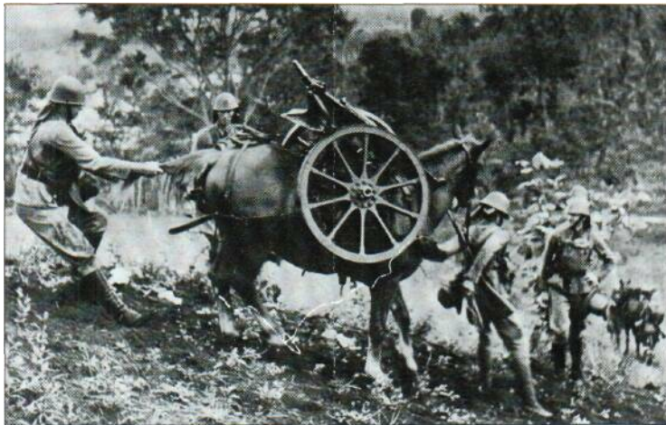
The Netherlands army used their Bofors 75-mm Model 1934 howitzers in the Dutch East Indies, where they were carried into action in pack loads carried by mules. Note how brakes were applied to this carrier mule as it moved down a steep slope carrying the wheels and part of the carriage trails.
