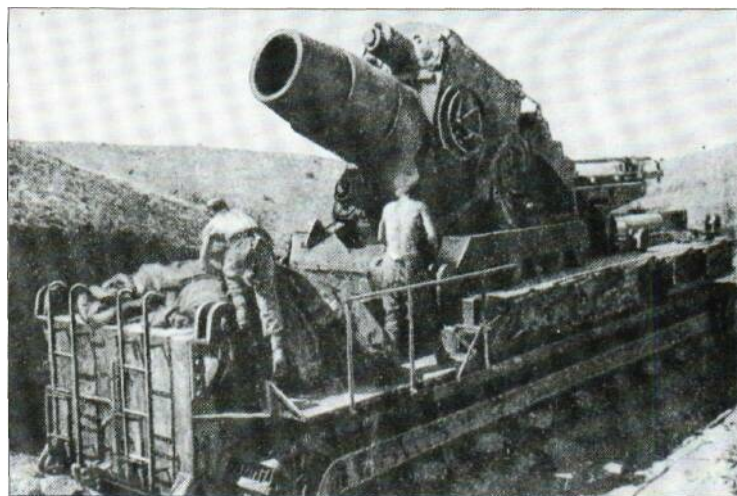
The massive 60-cm and 54-cm Karl howitzers were really fortification-smashing equipments, and they had only limited tactical mobility. They
