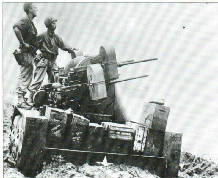
A Multiple Caliber .50 Machine-Gun Carriage M51 is seen in action at Hollandia on New Guinea against low-flying aircraft. This trailer-borne
