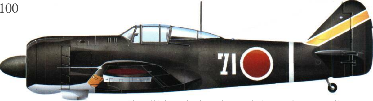
The Ki-100-1b introduced a cut-down rear fuselage over the original Ki-61 shape, which improved pilot vision. This aircraft is from the 3rd Chutai, 59th Sentai.
