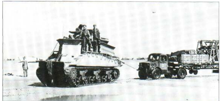
The Sherman BARV (Beach Armoured Recovery Vehicle) was developed during 1943 to tow bogged-down vehicles from deep water during amphibious operations. It was a tractor device only, and the crew usually included a trained diver to secure towing cables to stranded vehicles for towing.
