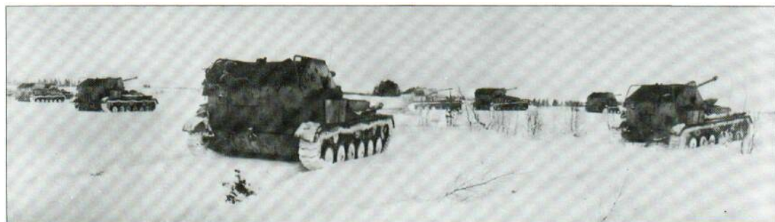
The Soviet SU-76 was a wartime and rather rushed conversion of the T-70 light tank to carry a 76-mm field gun, and although it was produced in large numbers it was little liked by its crews, who called it the 'Bitch'.
