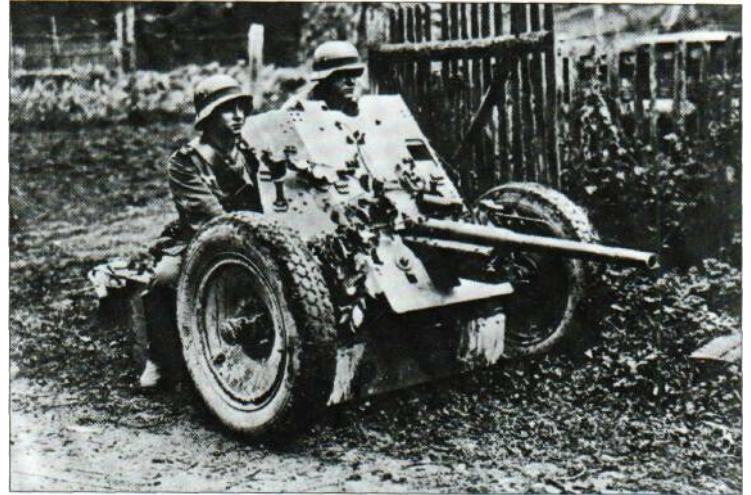
Above: The original 3.7-cm Pak 35/36 produced during the late 1920s had spoked wheels for horse traction, but by the mid-1930s these had been replaced by steel disc wheels for motor traction. It was a light and low gun that was at first issued to all arms of the Wehrmacht.
