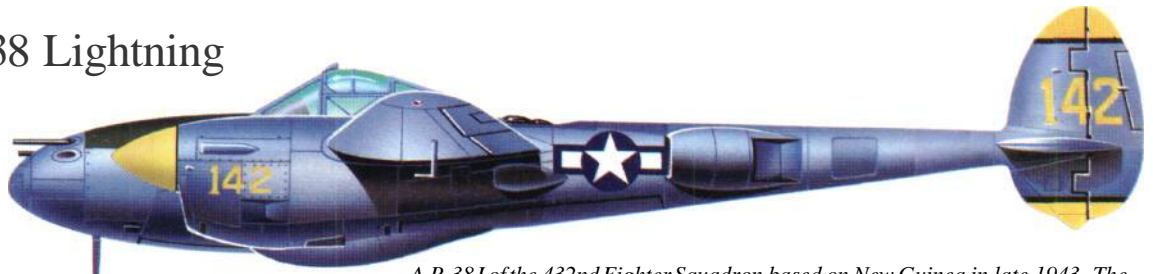
A P-38J of the 432nd Fighter Squadron based on New Guinea in late 1943. The 'J' models were the first to have relocated radiators and leading-edge tankage.
