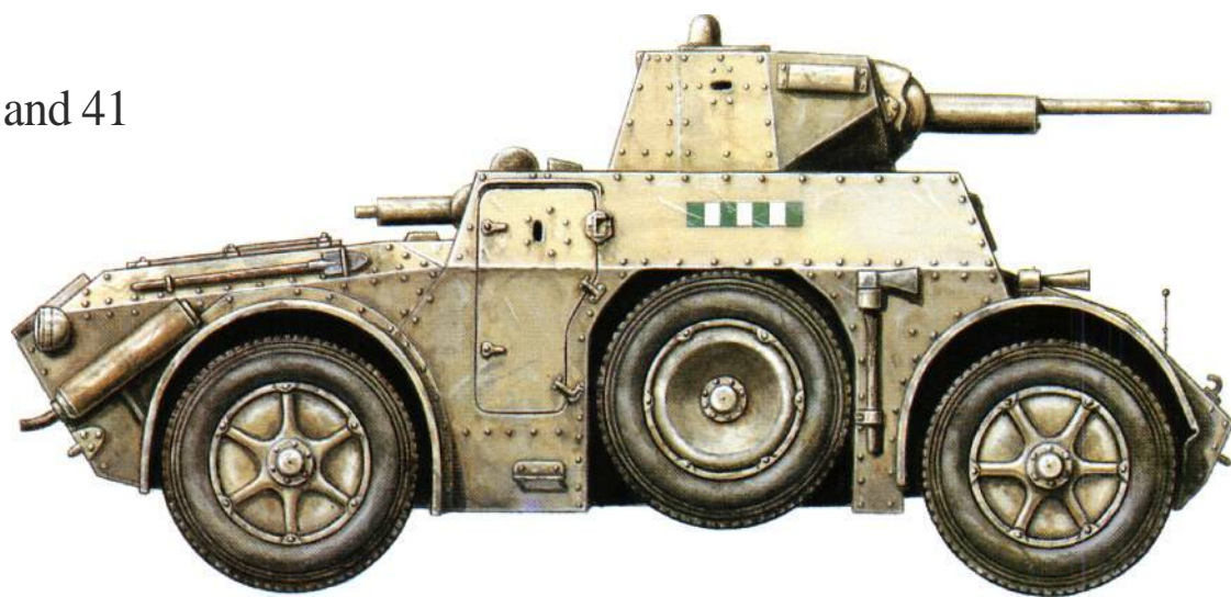
The Autoblinda 41, one of the most numerous of Italian armoured cars, is shown armed with a turret-mounted 20-mm cannon and a machine-gun at the hull rear.
