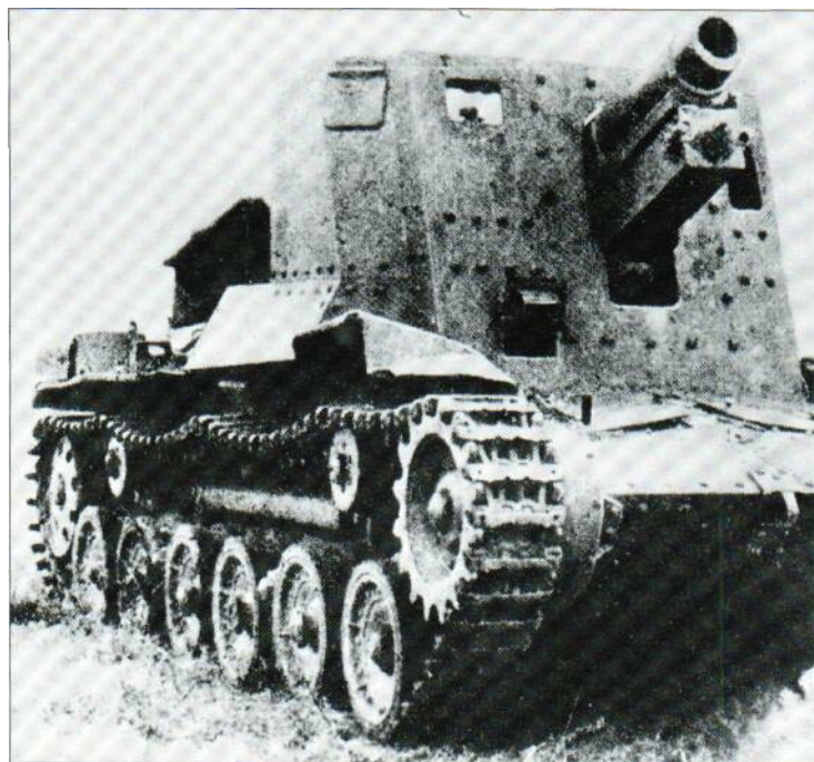
The Type 97 had its 150-mm howitzer mounted in place of the turret normally carried. The howitzer was
