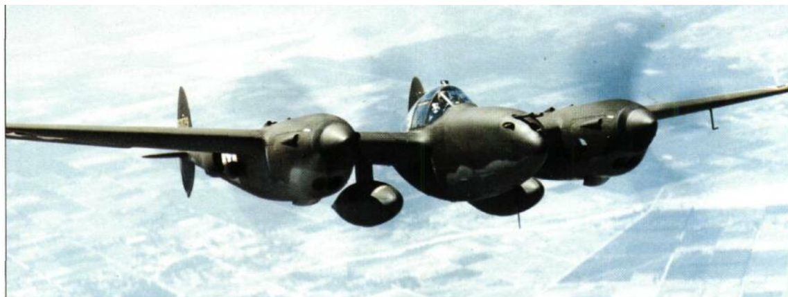
The Lightning had exceptional performance for a twin-engined aircraft and the secret of this lay in the small frontal area made possible by the twin boom layout. The position of the racks for either bombs or, as here, fuel tanks is clearly visible.
