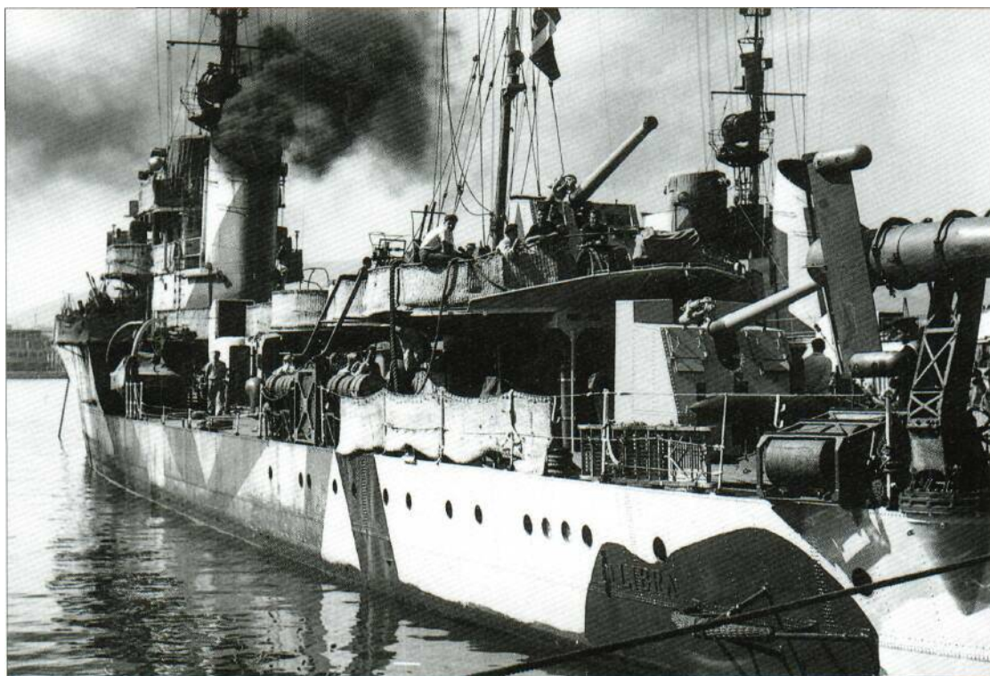
Italian torpedo boat, or light destroyer, Libra of the Alcione class of vessels, which were brought into service in 1938 and lasted until the 1960s.
