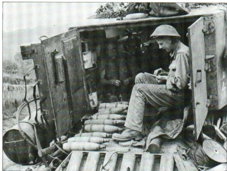
Above: Ammunition stocktaking takes place on a Bishop with the projectiles laid out on the engine covers for counting. The Bishop could carry only 32 rounds in ternally,
