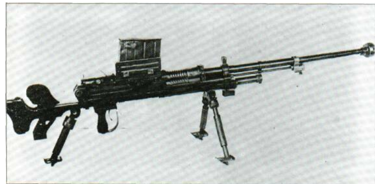
The 20-mm (0.787-in) Type 97 anti-tank rifle used a gas-operated mechanism, but the heavy recoil involved meant that a fully-automatic mode could be little used. Four men were needed to carry this rifle using special frames, and a shield was an optional extra. The box magazine held seven rounds.
