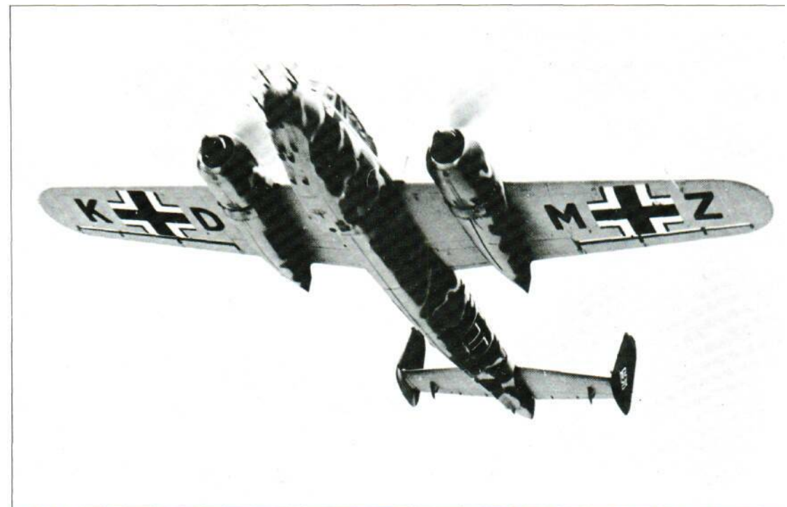
KD+MZ were the Dornier factory codes of the Do 217 development aircraft, seen here with the bomb bay of the Do 217J-1 but the Lichtenstein BC (FuC 202) radar of the Do 217J-2. Operational Do 217J-2s were all-black.
