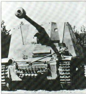
A Marder II with the 7.5-cm (2.95-in) Pak 40/2 gun barrel clamps lowered. Although this vehicle was one of the more important (numerically) of the Panzerjäger, it was rather high and generally lacked protection.
