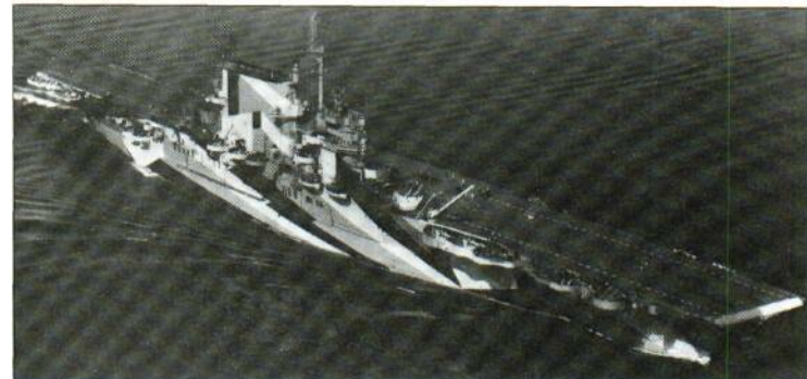
'Sara' in September 1944, painted in Camouflage Measure 32/11A. Twin 5-inch and light AA guns have
