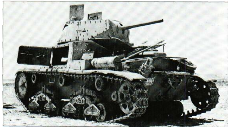
Another M14/41, abandoned after the first battle of Alamein. The M15142 looked similar but had no side hatch. Only 82 were built.
