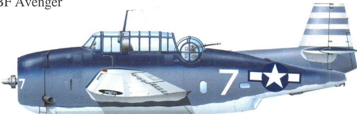
Grumman TBF Avenger of the US Navy. Armament of the dorsal turret was one 0.5-calibre machine-gun.
