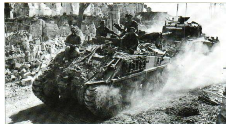
A Sherman ARV Mk I tows a Sherman gun tank during the campaign in Normandy, June/July 1944. This ARV was a British conversion of a Sherman tank that involved removing the turret and fitting a front-mounted jib crane and other equipment.
