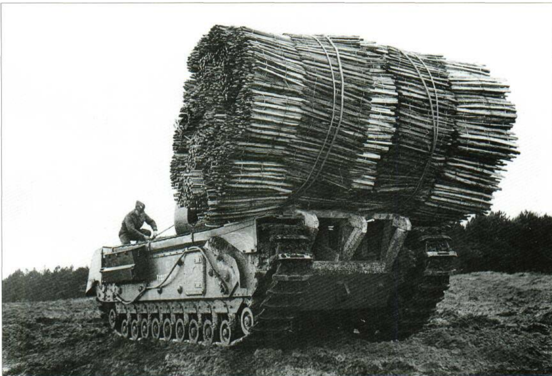
A Churchill tank with a fascine attached to the front which could be used to lay a mat over soft ground - such as sand on the Normandy beaches - for other tracked vehicles to cross.
