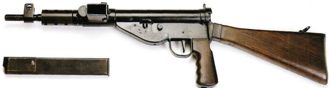
Below: By the time the Sten Mk V was produced there was time for some finesse to be added to the basic design. While the original outline was retained a wooden butt and pistol grip and No. 4 rifle foresight had been added.
