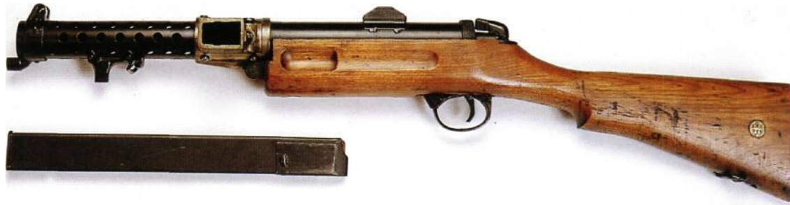
Above; Obviously based on the German MP 28, the Lanchester was ideally suited to the rough-and-tumble of shipboard life. It had a one-piece wooden stock based on the outline of the Lee-Enfield No. 1 Mk 3 rifle and there was a bayonet lug under the muzzle. The brass magazine housing can be seen.
