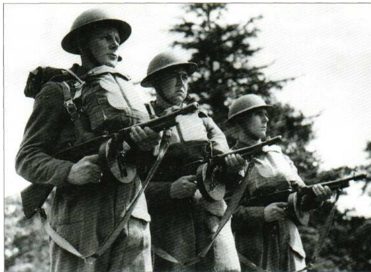
British troops wielding the American-designed .45in Thompson M1928 machine-gun, popularly known as the Tommy Gun'. These drum magazines carried 50 or 100 rounds but proved too troublesome in use so various box types replaced them.
