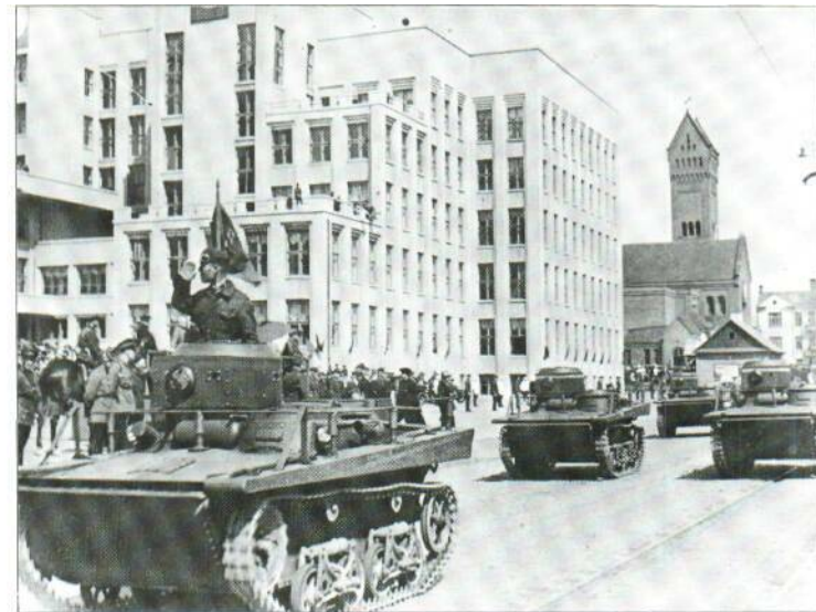
T-37 light amphibious tanks on parade in the Soviet Union. The three leading tanks are T-37(TU) command tanks fitted with frame aerials and radios; most T-37s had to communicate with flag signals as the general issue of tank radios was not standard practice until after 1945.
