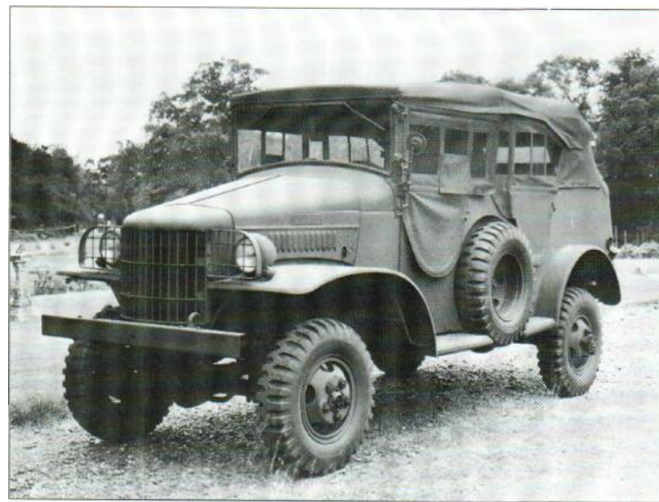
The Dodge T215 WC23 was a 1/2-ton command and reconnaissance vehicle of the same family as the T207. The 1941 pattern vehicles are identifiable from the heavier 1942 models by their sloping bonnet.
