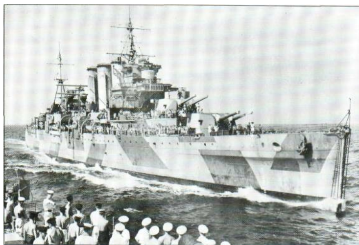
Below: HMS Norfolk as she appeared in 1943. The 'County' class heavy cruisers were a compromise designed to operate effectively in the protection of long trade routes. They had excellent endurance and were popular with their crews.
