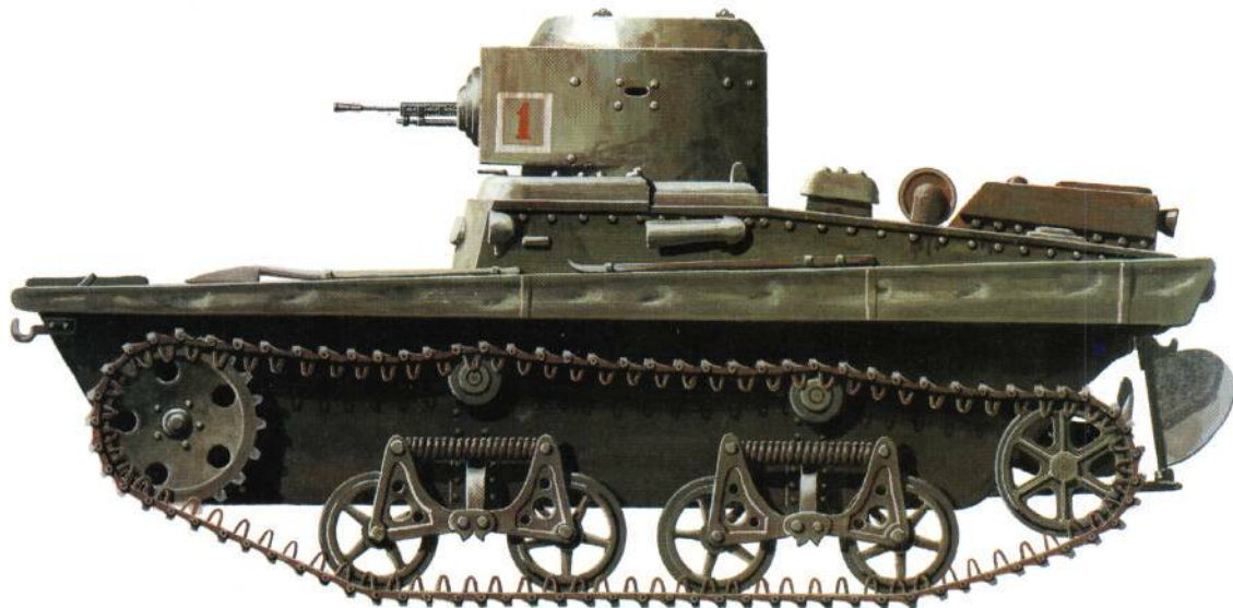
Above: The tiny T-37 light amphibious tank was produced in several versions, but all were lightly armoured and had only two-man crews. They were in production from 1935 onwards, but few survived after the end of 1941 as they were too frail to stand up to prolonged combat.
