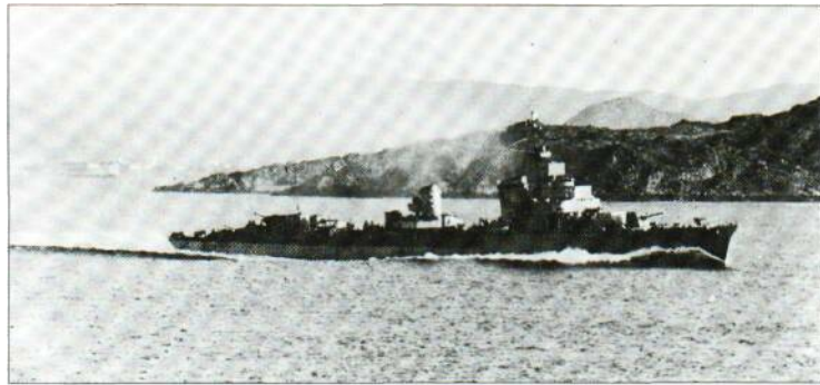
Z25 cruises purposefully off the Norwegian coast before her conversion to 'Barbara' standard, which gave her an impressive AA capacity of 12 37-mm (1.45-in) and 18 20-mm (0.78-in) automatic weapons. Transferred to the French navy, she served as the Hoche until 1956.
