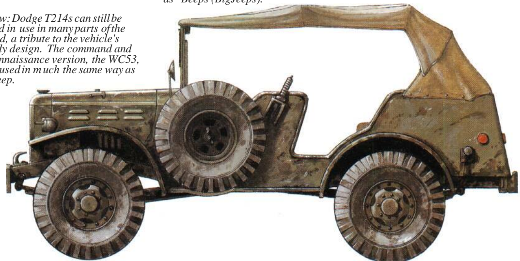
Above: Superseding the T207-WC3, the T214 range of trucks were 3/4-ton vehicles. Introduced early in 1942, they were in full production by June. Used to transport personnel, weapons, tools and equipment, the T214 range were sometimes known as 'Beeps' (Big Jeeps).
