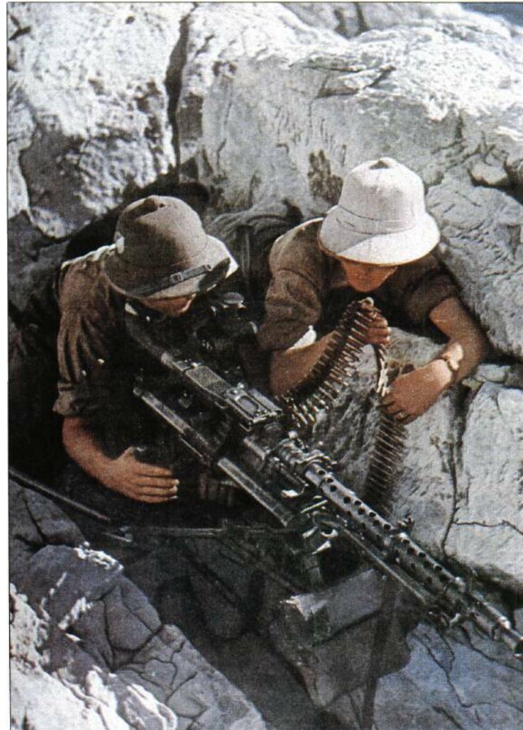
Two Afrika Korps soldiers with an MG 34 in the heavy machine-gun role on a Lafette 34. By removing the indirect fire sights and trigger, the MG 34 quickly converts to an LMG.
