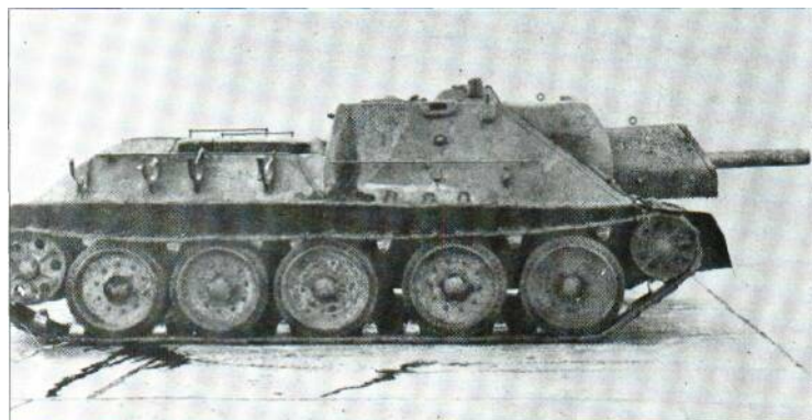
The SU-122 was a conversion of the T-34 tank to accommodate a front-mounted 122-mm howitzer in a well-armoured and well-sloped superstructure. It was produced in large numbers for the close-support role, but could be used for 'stand-off' artillery fire.
