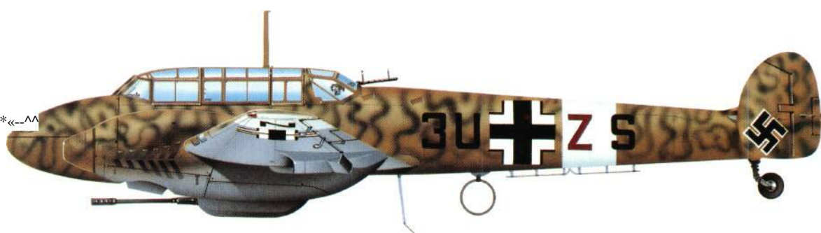
A Messerschmitt Bf 110E of 8./ZG 26 based at Berca, North Africa, in September 1942. It is armed with the powerful MK 101 30-mm cannon, for use in the tank-busting role.
