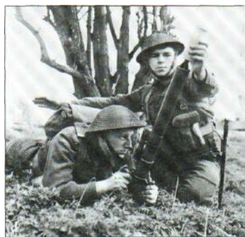
A drill book demonstration of the loading of a 2-inch Mortar. As the loader drops the bomb into the muzzle, he taps the firer on the back to order him to pull the trigger lever via a cord lanyard. The model is the Carrier version with the large baseplate.
