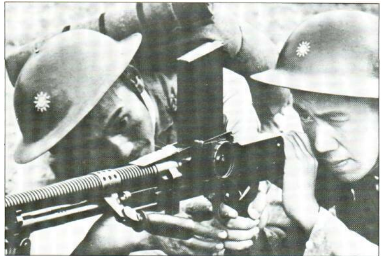
Above: The Czech ZB vz.26, one of the most influential designs of its day and the forerunner of the British Bren gun; this example has its straight 120- or 30-round box magazine missing.
