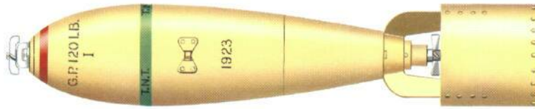
Left: The 54-kg (120-lb) GP HE bomb was one of a series of new, improved bombs of better aerodynamic shape than those used since World War I. This weapon replaced the old 50-kg (112-lb) GP bomb.
