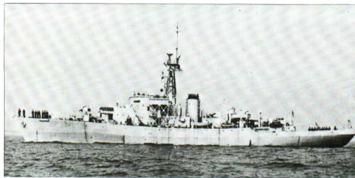
Armament: one 101.6-mm (4-in) DP, and two twin and six single 20-mm AA guns, one Squid, and depth charges Complement: 120
