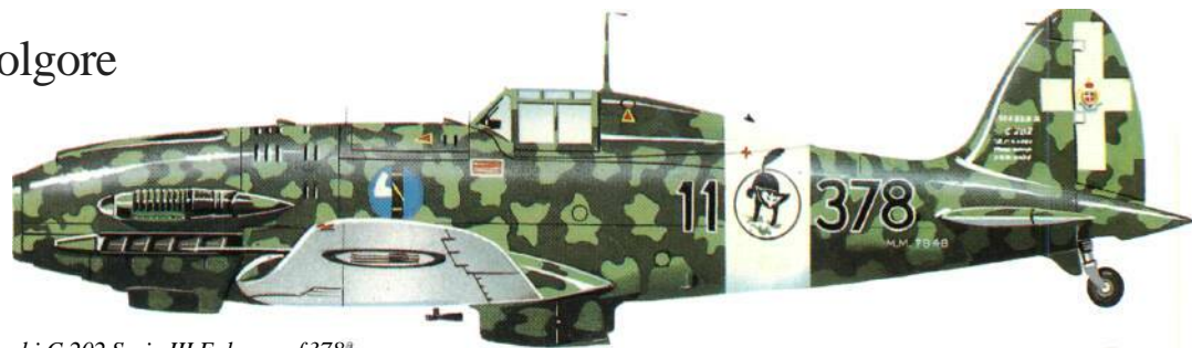
Macchi C.202 Serie III Folgore of 378 a Squadriglia, 155° Gruppo, 51° Stormo. The C.202 was the most effective of Italian fighters but suffered from lack of armament.
