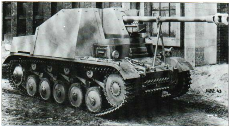
The SdKfz 131 Marder II mounted a 7.5-cm (2.95-in) Pak 40/2 and was one of the more important of the Panzerjäger conversions. Based on
