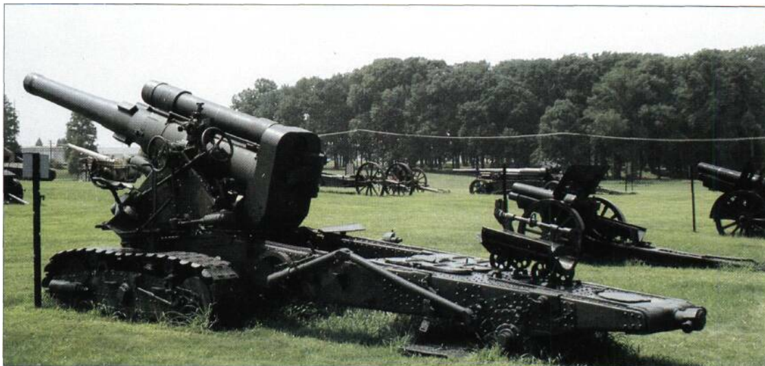
Above: The heaviest Soviet gun in field use during the war, the 203-mm Howitzer Model 1931 was mounted on converted agricultural tractor tracks widely available in the Soviet Union as a result of Stalin's lopsided industrialization programme. It fired a 100-kg (220-lb) shell to a maximum range of 18 km (11 miles).
