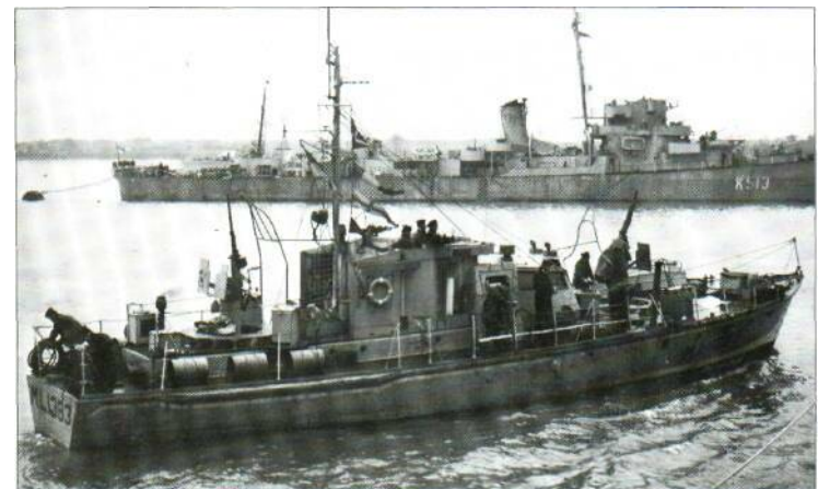
HDML 1383 leaves Harwich harbour past HMS Curzon (formerly the US destroyer escort DE-84). This example is armed with a 20-mm Oerlikon fore and aft and twin Lewis guns on each side of the bridge.
