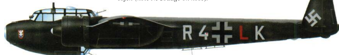
The Do 17Z-10 Kauz II was the first sensor-equipped Luftwaffe night fighter, with the Spanner sight projecting through the windscreen. R4+LK served with I/NJG 2 at Citzel-Rijen (note NJC badge on nose).
