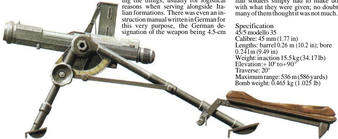
The Italian 45/5 modello 35 'Brixia' mortar was one of the most complicated mortar designs ever produced. It used a lever-operated breech mechanism and fired tiny 0.465-kg (1.025-lb) bombs.
