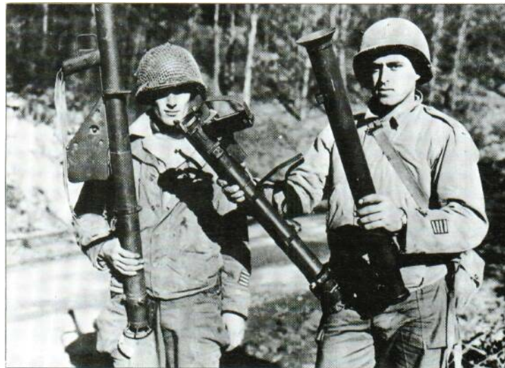
The original M1 bazooka is shown on the left and the M9 on the right. The M9 could be broken down into two halves, which greatly assisted carrying and stowage inside vehicles. By the time the war ended a version of the M9 was being produced in aluminium for lightness; this was the M18.
