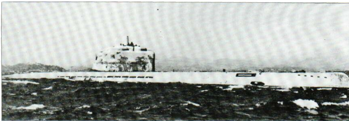
Above: Lack of paint on both tower and stemhead are clues to the high speeds attained by this Type XXI. The hull is faired into an almost elliptical cross-section, leaving little deck, and the forward hydroplanes fold back into slots to reduce drag.
