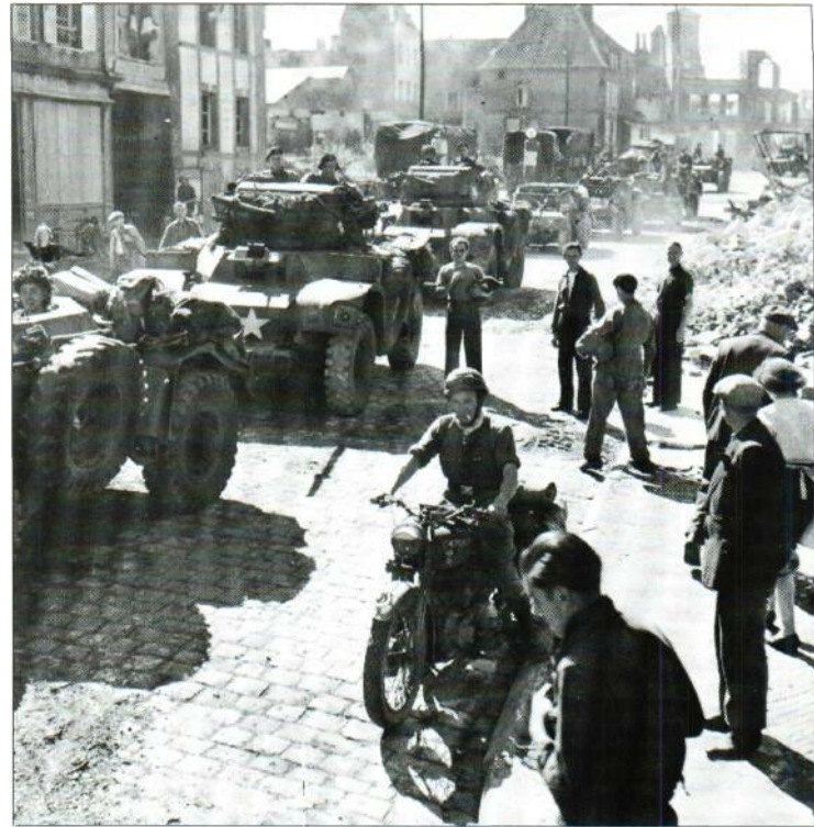
A British reconnaissance unit moves through the village of Gacein Northern France during August 1944. The turreted armoured cars are Daimlers and also visible are Daimler Scout Cars; the vehicle just visible on the left is a Humber Scout Car. The white star was the Allied recognition symbol of the period.
