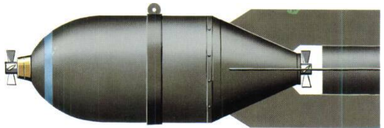
The 100-kg (220-lb) high-explosive bomb was a standard weapon used by Ilyushin Il-2s for ground attack work. The famous heavily-armoured attack aircraft could carry six of these bombs.
