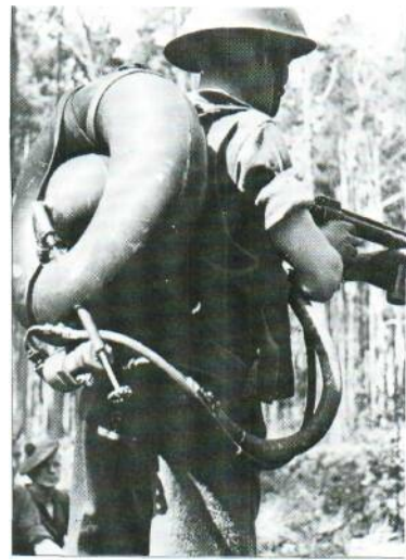
Above: The Mk I version of the Flame-Thrower, Portable, No. 2 was usually known as the Lifebuoy from its shape, but it was not a great success and saw only limited operational use before being replaced in late 1943 by the Mk II.
