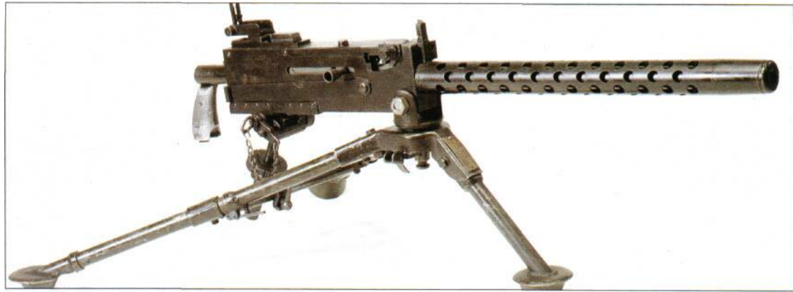
Above: A Browning M1919A4 machine-gun on its normal tripod and clearly showing the perforated barrel cooling jacket and the square receiver; it was produced in huge numbers and the type is still in use all over the world.
