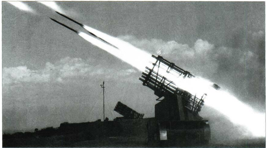
Mobile multiple-barrelled rocket launchers, such as this British 76.2mm (3in) anti-aircraft version, laid down huge blankets of fire; the most famous example of this weapon was the Soviet Katyusha.
