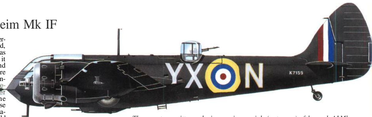
The nose transmitter and wing receiver aerials (antennas) of the early AI Mk III radar can be seen on this Blenheim Mk IF, which in 1941 was training crews at No. 54 Operational Training Unit, RAF.
