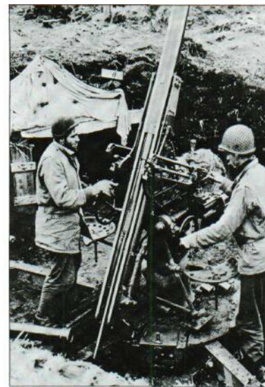
Above: The mount of a captured Type 88 75-mm gun is examined in the Pacific. Notice the five legs of the firing platform and the detached barrel at the bottom left of the photograph.
