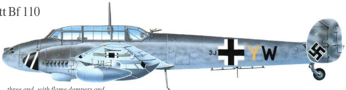
Above: Though fitted with enlarged fins and DB G05A engines, the early Bf 110G models lacked flame-damped exhausts, and this Bf 110G-2 of 12/NJG 3 had no radar. It was based at Stavanger until the final collapse in May 1945.
