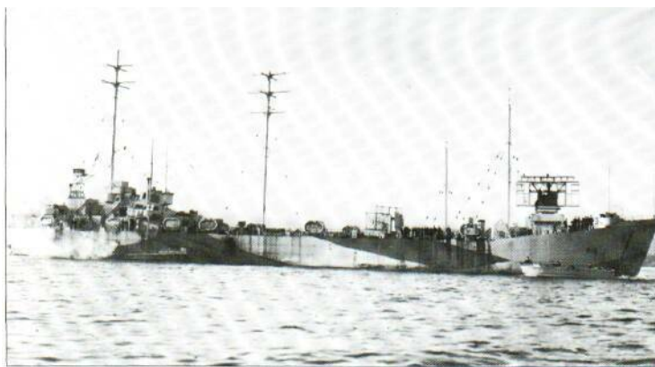
Above: LST216 after conversion to fighter-director. Offices built into the tank deck included those for communications, fighter control and radar plotting, as well as workshops and stores.
