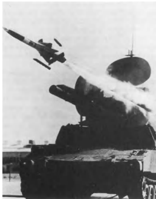
Fig. 3. Launching of a field-mobile, short-range, all-weather surface-to-air Roland missile. The German-French Roland has been licensed for production in the United States for use as a U.S. Army air defense weapon. (U.S. Army)
