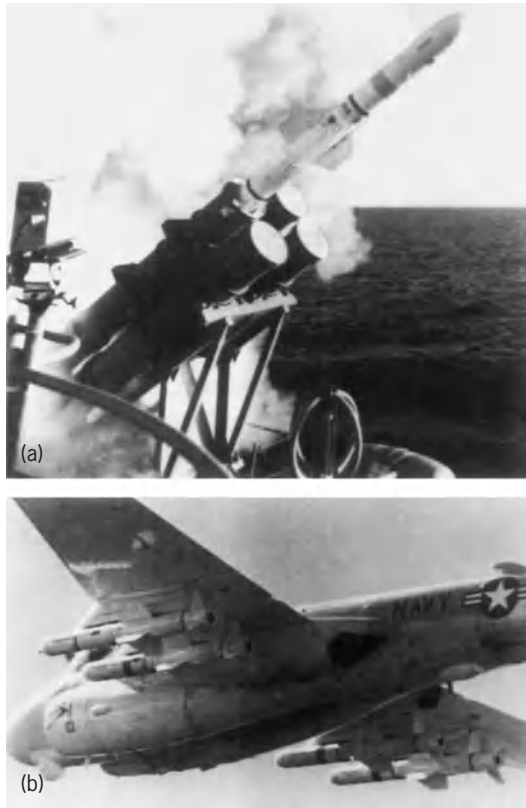
Fig. 8. Harpoon antiship cruise missile. (a) Ship-launched. (b) Air launch version on A-6 intruder attack aircraft. (McDonnell-Douglas)
