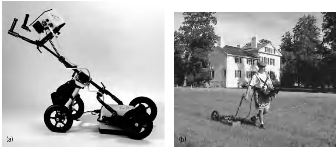
Fig. 1. Ground-penetrating radar equipment. (a) Portable equipment with 500-MHz antenna and controller that displays scrolling vertical slices of the soil in real time (USRADAR). (b) Portable equipment with 400-MHz antenna being used in archeological survey at Franklin D. Roosevelt's Hyde Park Estate in New York (Geological Survey Systems, Inc.).
