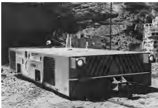
Fig. 20. A 16-ton (14.5-metric-ton) diesel locomotive with exhaust water scrubber for use in coal mines. (Brookville Locomotive Division of Pennbro)
