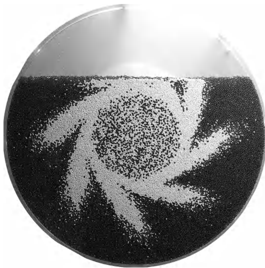
Fig. 10. Unmixing of particles of two different sizes in a rotating tumbler operating in a time periodic mode.
