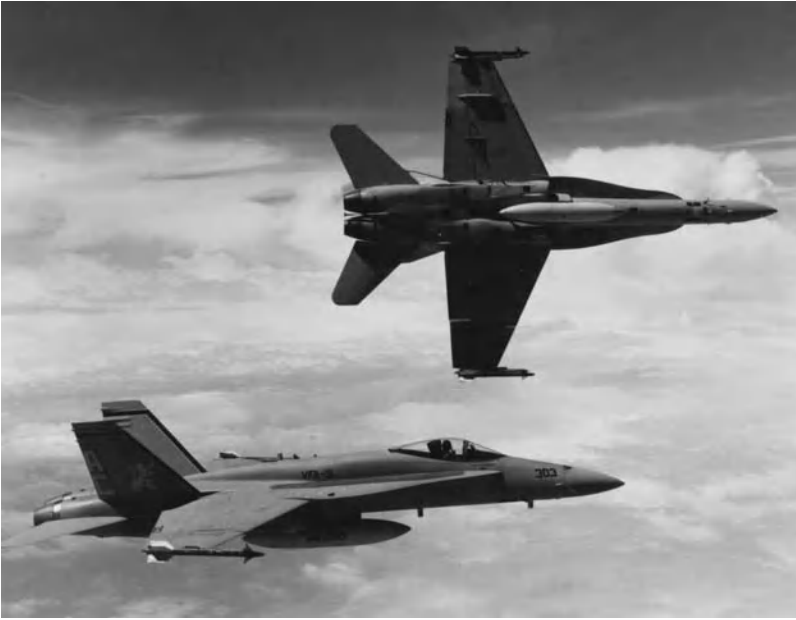
Fig. 7. Two McDonnell Douglas F/A-18 (Hornet) strike fighter aircraft, each carrying two heat-seeking Sidewinder missiles and an external fuel tank. (McDonnell Aircraft Co., McDonnell Douglas Corp.)
