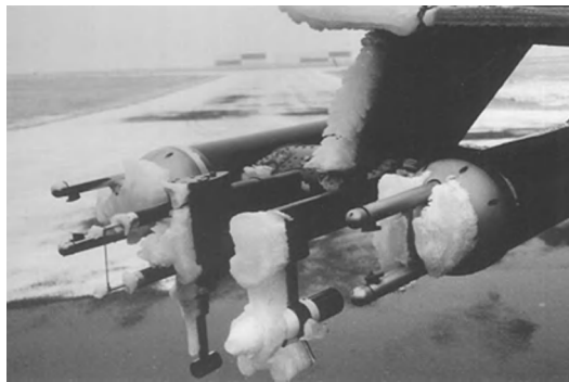
Fig. 2. Hydrometeor optical spectrometers and temperature sensors on a research aircraft. Optical spectrometers use lasers to create particle shadow images in two dimensions. Particles are imaged as they flow between the blunt arms ahead of the electronics pod beneath the wing. ( University of Wyoming )
