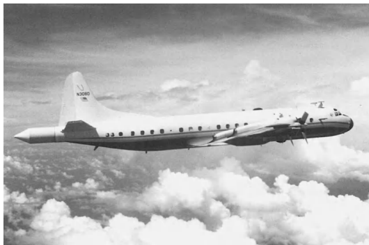
Fig. 2. Electra aircraft; the antenna radome. (R. Carbone, National Center for Atmospheric Research)
