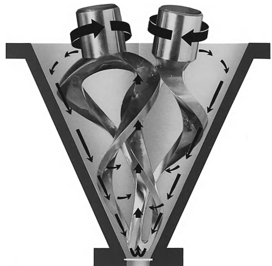
Fig. 8. Ribbon turbine with double spiral, for high-viscosity liquids.
