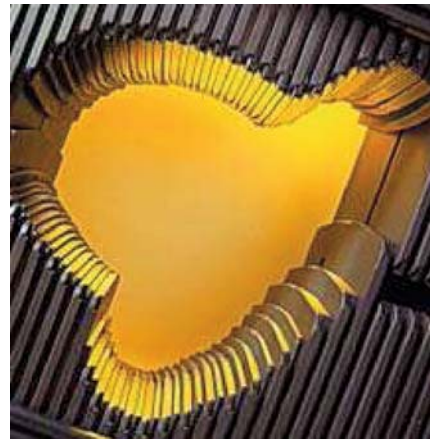
Beam Selection in Radiotherapy Treatment Design, Figure 2 A multileaf collimator
