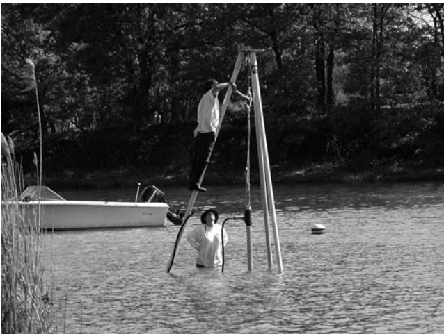
Figure V4 Retrieval of vibracore using a portable aluminum A-frame. The lightweight A-frame has pads on the feet so the unit does not sink into the sediment when load is applied. One leg of the A-frame has steps so the driller can extract the core barrel with a hand-operated come along. The A-frame must be placed vertically over the core barrel to ensure easy extraction without flexure or bending of the core. The A-frame collapses into a compact unit for transporting (Photo courtesy of Steve Krupa, South Florida Water Management District, West Palm Beach, Florida).
