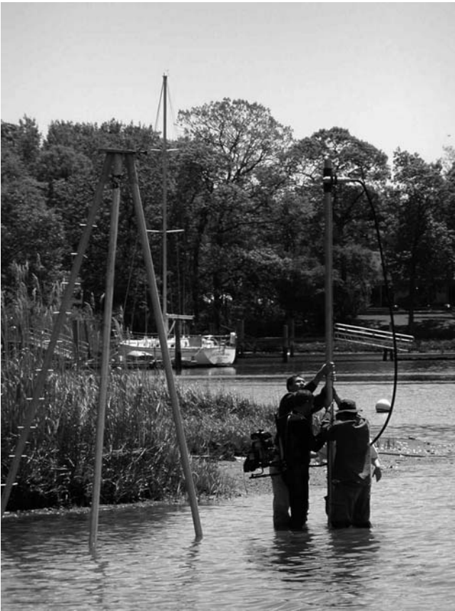
Figure V3 Small, portable vibracore. A backpack power unit operates this pneumatic vibracore; the core barrel is stabilized by hand as the unit penetrates the marsh sediments. The lightweight aluminum A-frame is carried to the site and waits for use in retrieval of the core (photo courtesy of Steve Krupa, South Florida Water Management District, West Palm Beach, Florida).
