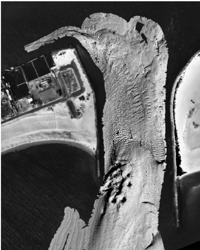
Figure M28 Multi-beam acoustic data from Shinnecock Inlet, Long Island, New York, December 1998. Sand waves are evident in the inlet, and the highly irregular bottom near the west jetty indicates scour holes. North is to the top of the image. (Data collected and processed by State University of New York, Stony Brook.)
