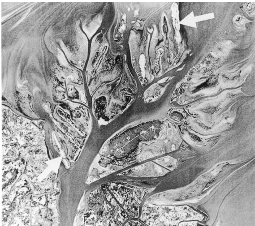
Figure W33 Arrows point to recently created dredged material wetlands built to mimic the natural geomorphology of the Atchafalaya Delta, Louisiana, USA.
