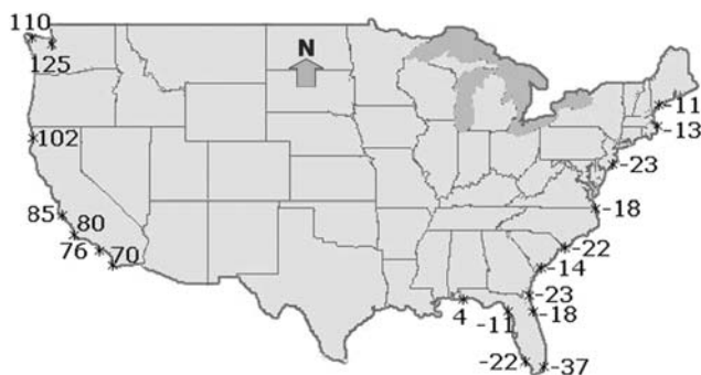
Figure T13 Height in centimeters of MSL datum above NAVD88 (redrawn from USACE, 2002).
