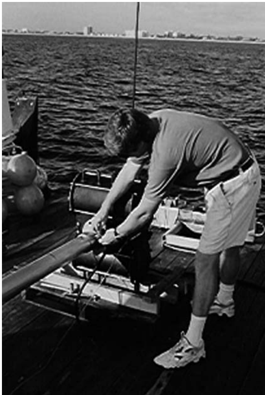
Figure V8 The 7.5-cm-diameter core barrel is attached to the electric vibrahead assembly prior to being lowered overboard into the Atlantic Ocean as part of an offshore sand search near Miami, Florida. Although the unit is of medium size, the weight of the vibracore assembly requires crane winching from the deck (photo courtesy of Coastal Planning & Engineering, Boca Raton, Florida).
