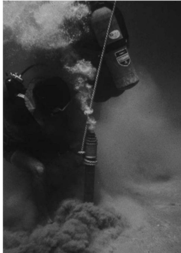
Figure V10 A "wash boring" that is operated by jetting down a pipe within a pipe at intervals of 1–2 m and "washing" up a sample with a blast of compressed air between the pipes. This exploratory technique was previously used to provide preliminary information on the quality of sand in a potential borrow area before engaging more expensive vibracoring operations. Although surface sand samples can be easily obtained, it is necessary to know what type of material lies at depth. This method of sampling provided an inexpensive way to sample sediment at depth, which would be "washed up" the pipe and trapped in cloth bags that were used to catch the samples. The heavier materials (gravel, etc.) could not be lifted in the pipe, but divers could "hear" gravel and rocks banging against the casing to establish the presence of unusable coarse materials. Fines could not be trapped because the material would pass through the cloth bags used to trap sediment samples; the "cloudiness" of the water, however, provided experienced divers with a rough indication of how much silt plus clay was present in the sediment. The penetration of the pipe was similar to jet probes that are now used in order to test the depth of unconsolidated sediment. Although crude, this method provided useful information for refining sand searches. The limitations of disintegrated wash borings compared to undisturbed vibracores emphasize the value of cores that can be subsampled, analyzed, and archived. Wash borings today find specialized applications by most researchers (photo courtesy of Coastal Planning & Engineering, Boca Raton, Florida).
