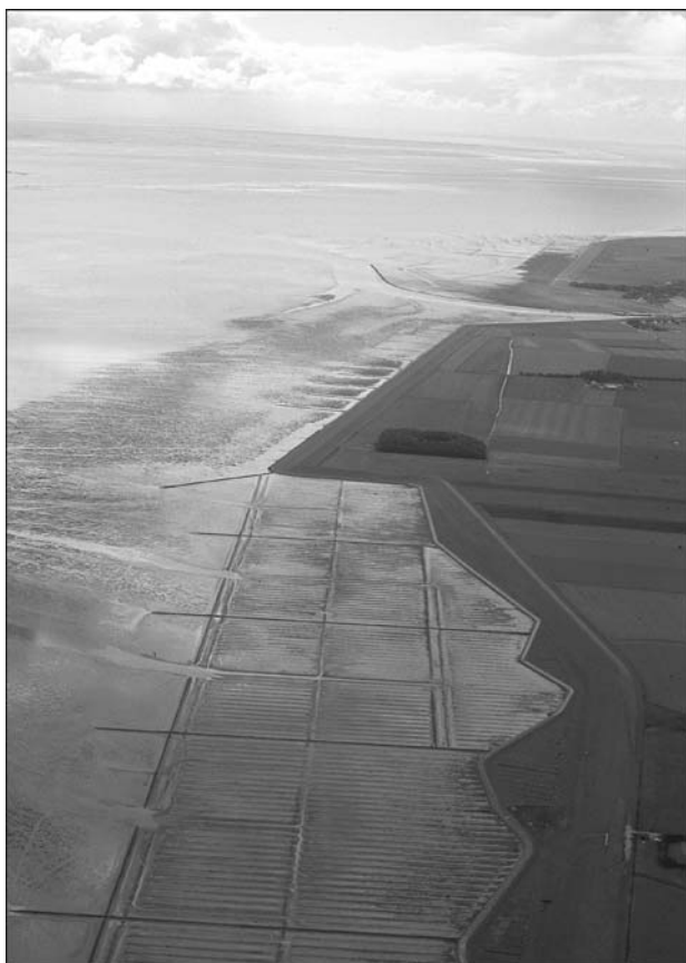
Figure E36 Land reclamation outside the marshes at the northern German North Sea coast, mostly as a tool for protection of dikes and farmland.
