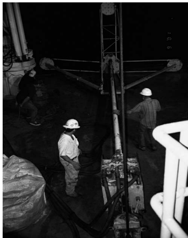
Figure V2 Same vibracore assembly unit shown in Figure V1 being laid down on the deck. The long core inside the 10-cm-diameter core barrel will provide valuable undisturbed sediment data from the seabed on the continental shelf off Louisiana. Operations such as this one require experienced crew to handle these large vibracoring units (photo courtesy of Coastal Planning & Engineering, Boca Raton, Florida).
