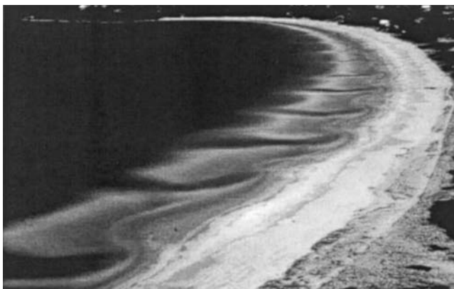
Figure R18 Enhanced time-exposure image of topographically arrested accretion rips at Palm Beach, NSW, Australia. Rip channels appear as dark areas between bars (white regions) and are approximately 150–200 m apart. Note the absence of pronounced longshore feeder channels (image courtesy of G. Symonds, R. Holman, and R. Ranasinghe).
