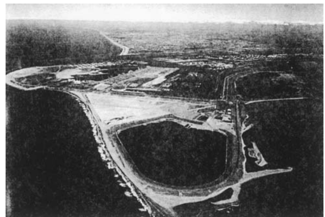
Figure D47 The "Slufter" offshore diked disposal are used by EURO-PORT (Rotterdam) for polluted materials (adapted from Brunn, 1990b).
