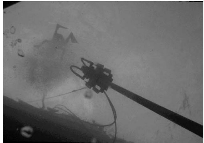
Figure V9 Diver's view of vibracore being lowered over the side of the research vessel. The dark area in the upper left of the photo is the bottom of the vessel's hull. Cables to power the vibrahead and a lifting cable are visible to the left of the diver near the water surface (photo courtesy of Coastal Planning & Engineering, Boca Raton, Florida).
