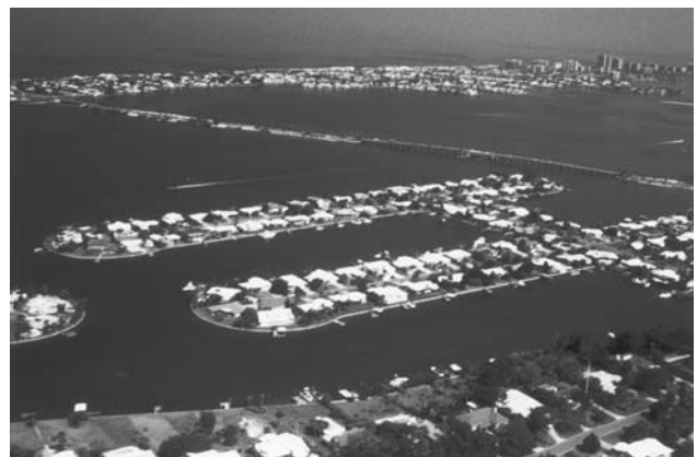
Figure H20 A fill-type causeway constructed between the mainland and a barrier island.
