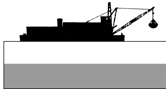
Figure D37 The clamshell or grapple dredge (adapted from Bruun, 1990b).
