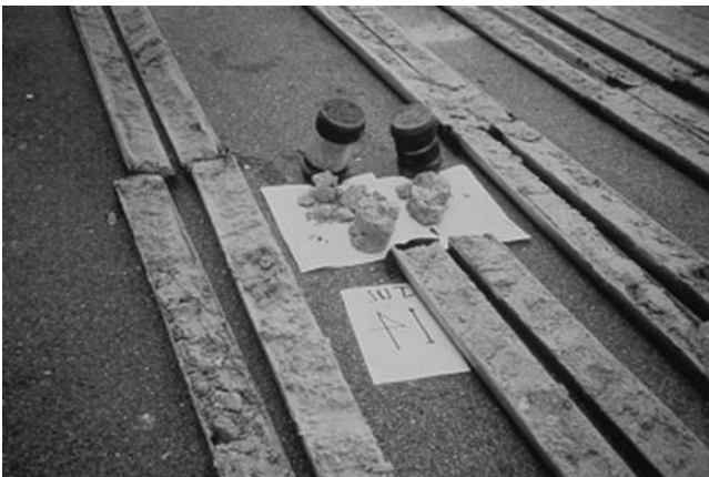
Figure V11 Split core liners from vibracore that penetrated sandy bottom sediments in an inter-reefal area offshore from Miami, Florida. The vibracores are split longitudinally, one half is retained for archival purposes and the other is logged and analyzed in the laboratory for grain-size parameters, organic content, coarse fragments (e.g., loose shell hash, pieces of coral, chunks of coquina), mineral composition (e.g., silicates versus carbonates), etc. Note: Core barrels are generally cut into sections that are about 2 m in length. Depending on the length of core obtained, there may be a small section left over that would be difficult to split lengthwise. These small leftover sections also tend to be disturbed because they are at the end of the core. The two PVC ends shown here are used to store "bit samples" because the core-cutting bit does not have a liner. Typically, when a core is being recovered, the material in the bit falls out because it is below the core catcher. Sometimes the sample stays in the bit and it is saved as shown in the photo. The two piled samples sitting on paper in the center of the photograph are plugs of rock, cut from the subsurface, that were lodged in the bit (photo courtesy of Coastal Planning & Engineering, Boca Raton, Florida).
