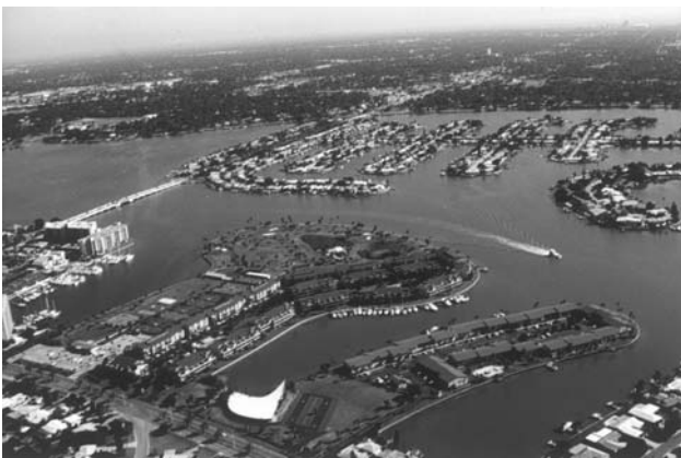
Figure H22 Finger canal development on the back-barrier area as the result of dredge and fill construction.
