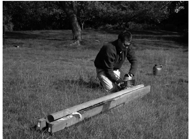
Figure V5 Splitting a vibracore. As shown here, the core barrel is laid in a wooden frame and an electric circular saw uses the frame as a guide to cut the flight lengthwise. The upper half is then rotated away from the frame and placed on the ground for observation and sampling (Photo courtesy of Steve Krupa, South Florida Water Management District, West Palm Beach, Florida).
