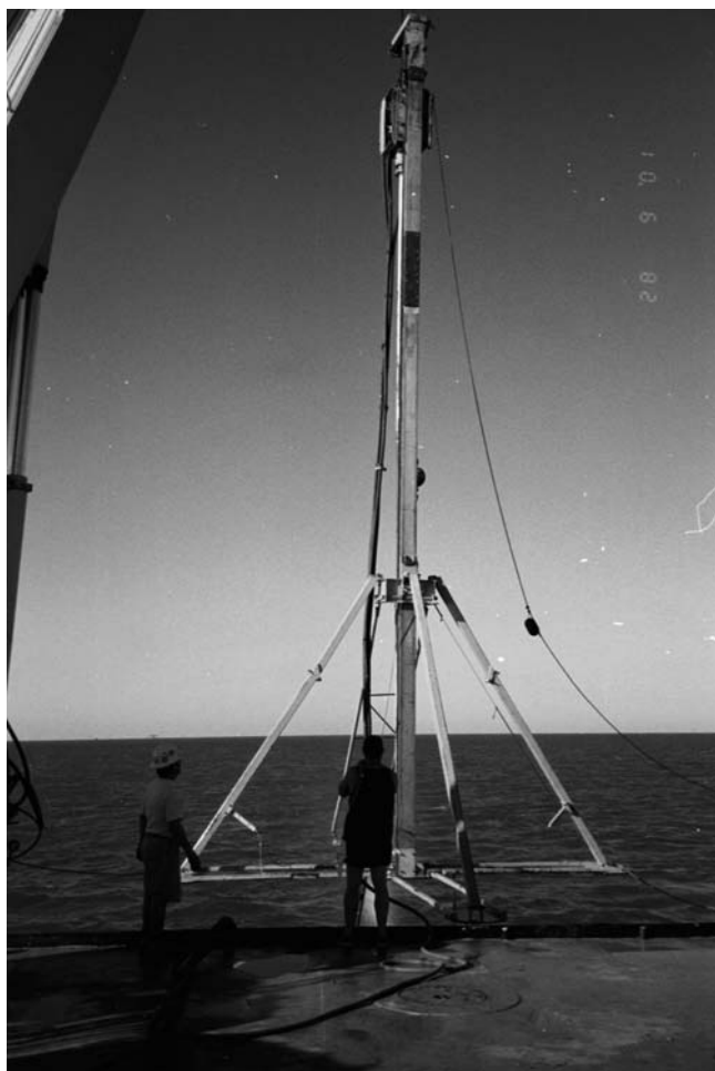
Figure V1 A 10-m vibracore (Alpine rig) being raised from the Gulf of Mexico seafloor offshore from Louisiana. The quadrapod stand stabilizes the vibracore frame, which sits on the seabed and allows the pneumatic vibrahead to slide downwards with core penetration. The entire apparatus is lifted aboard the research vessel using a hydraulic crane that reaches over the stern (photo courtesy of Coastal Planning & Engineering, Boca Raton, Florida).
