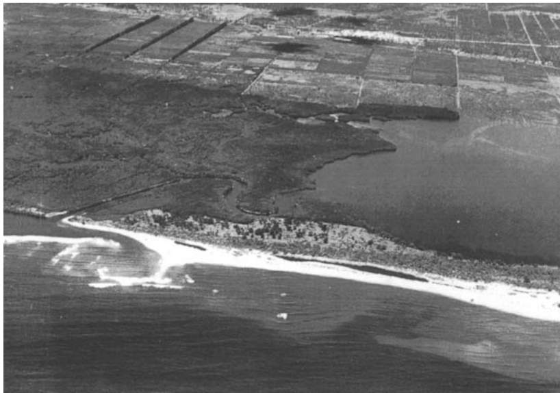
Figure N6 Bay mouth bar and barrier spit near Fort Lauderdale, Florida, ca. 1925 (looking from east to west). The shallow open freshwater body on the right side of this oblique aerial photograph is Lake Mabel, now converted into the Port Everglades Turning Basin. A 9-km long barrier spit, situated approximately 100 m offshore, continued alongshore from Fort Lauderdale to Dania passing in front of the bay mouth bar. Inlet cutting in Fort Lauderdale beheaded the updrift part of the barrier spit turning it into a barrier island that migrated shoreward over a three to five year period. During the migratory phase or barrier island rollover, approximately 6-10 \times 10^6 \text{ m}^3 of sediment was moved shoreward (Finkl, 1993). Shown here is welding of the barrier spit to the bay mouth bar. The remaining southern (left side of photo) portion of New River Sound opens to a temporary natural inlet. By 1930, the entire barrier island (formerly a barrier spit) was welded to the mainland. When the Intracoastal Waterway (ICWW) was dredged through the tidal marsh (left center of photo), the ICWW—beach tract of land was mistaken for a barrier island and is still so designated today. (Partial scanned image from an original 1925 print by Fairchild Aerial Surveys, Inc., Long Island City, New York.)
