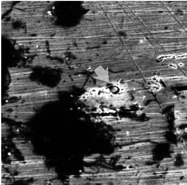
Figure 8. AISI 316 (1,000 \times ): anaerobic incipient localized pitting corrosion.
