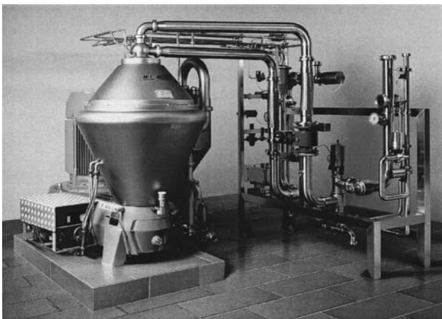
Figure 3. Solids-ejecting disk bowl centrifuge of production size. Capacity in breweries up to 75 m 3 /h. Type BREW 2000. The height of the separator is 2.2 m. Source: Courtesy of Alfa-Laval Separation AB.
