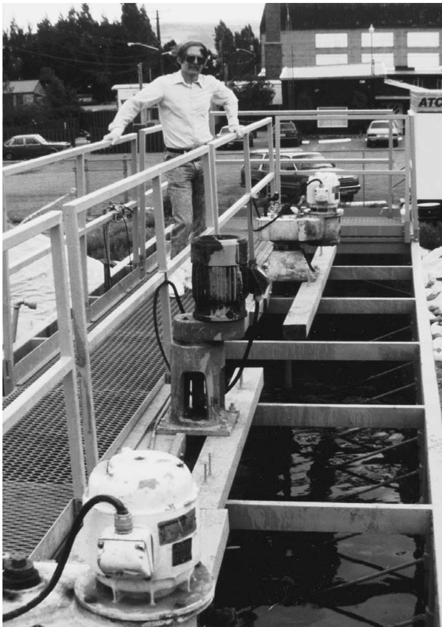
Figure 1. Pilot-scale anaerobic slurry reactor for treating TNT-contaminated soil. Source: University of Idaho, with permission.
