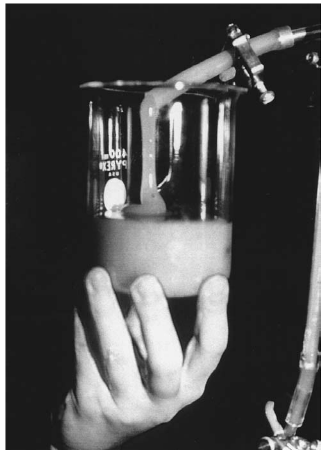
Figure 8. Highly viscous fermentation broth of A. pullulans in a sucrose medium: the broth slowly flowing out of a fully opened large-size sampling tube under the compressed air inside the fermenter.
