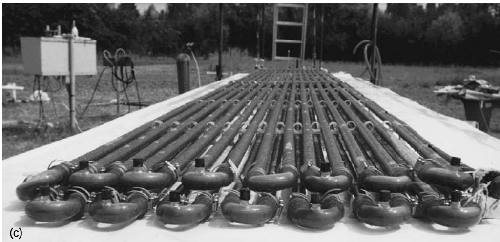
Figure 6. Horizontal serpentine photobioreactors set up at the University of Almeria, Spain (a) (photograph courtesy of E. Molina Grima) and at the Centro di Studio dei Microrganismi Autotrofi of Florence, Italy (b, c) (photographs courtesy of G. Torzillo).
