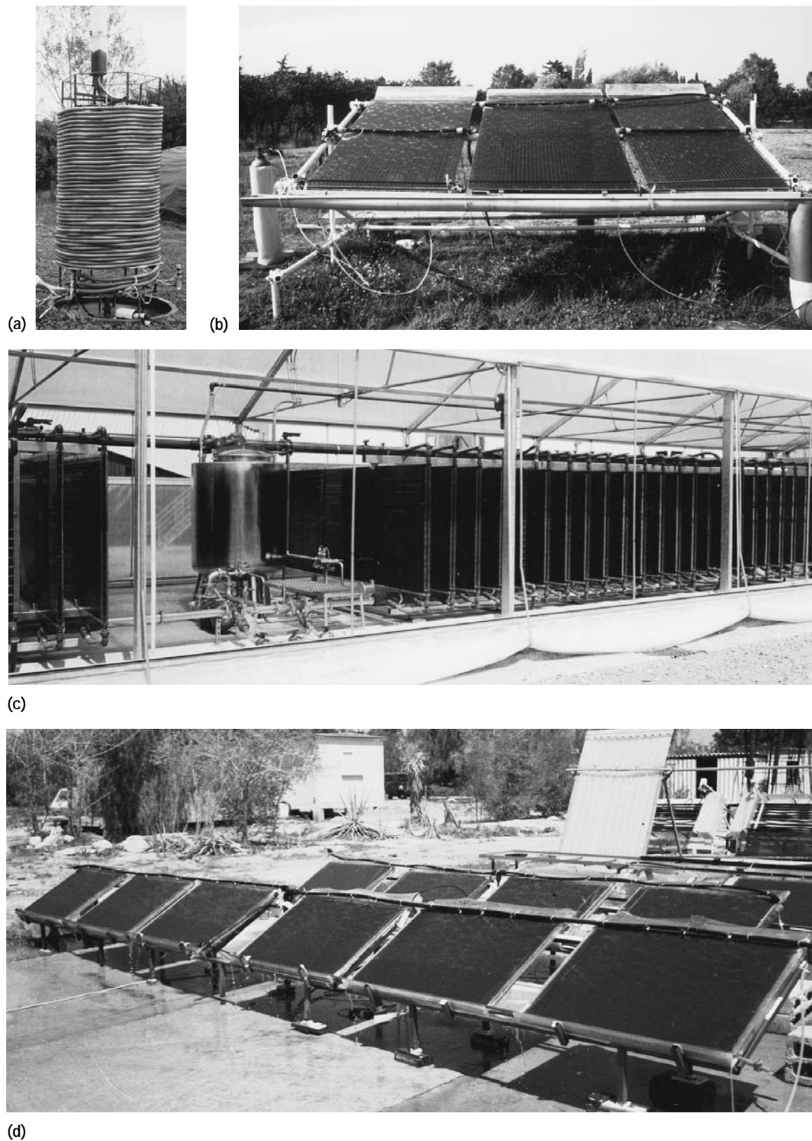
Figure 9. Biocoils and flat photobioreactors: (a) helical bubble-column reactor designed at the University of Florence, Italy (photograph by S. Pintus); (b) flat alveolar panels experimented with at the University of Florence, Italy (photograph by G. Chini Zittelli); (c) PBR system built by B. Braun Biotech Int., Germany (photograph courtesy of O. Pulz); (d) glass flat reactors experimented with at the Ben Gurion University of the Negev, Israel (photograph courtesy of A. Richmond).
