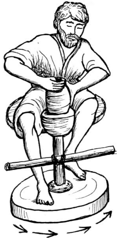
Potter’s wheel driven by foot power, allowing the potter to use both hands to shape the vessel.
