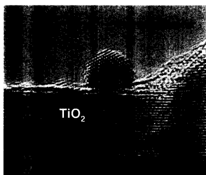
Fig. 2 The HR-TEM image of the eight-shell Pd nanocluster immobilized on the \text{TiO}_2 surface.
