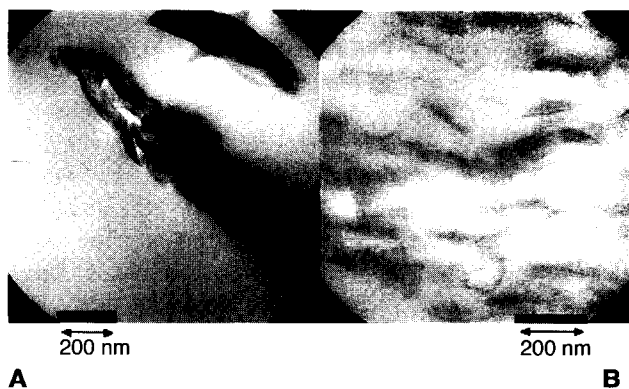
Fig. 3 Transmission electron microscopic image of polypropylene compound containing 10 vol.% organophilic fluoromica (M100/ODA) without addition of PP-g-MA compatibilizer (A, left) and the corresponding ME100/DA nanocomposite obtained in the presence of 20 wt.% PP-g-MA compatibilizer. (From Ref. [13] with permission from Marcel Dekker, Inc.)
