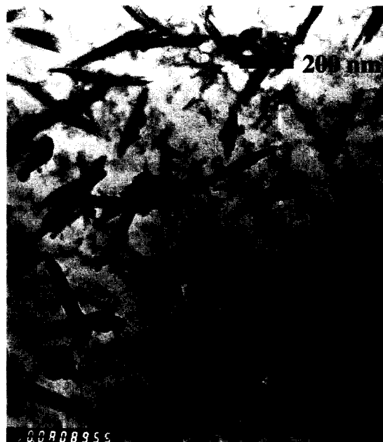
Fig. 4 TEM image of 2.5 layer-pairs with eight oxidative hydrolysis cycles using 4 mM NiCl 2 ·6H 2 O and ammonia base (50 K × magnification). The smaller particles are about 50 nm in length, while the larger particles are about 300 nm in length. The smaller nanoparticles are generated with each cycle, whereas existing particles continue to grow in size with each cycle. (From Fojas et al. [Ref. 39], with permission.)
