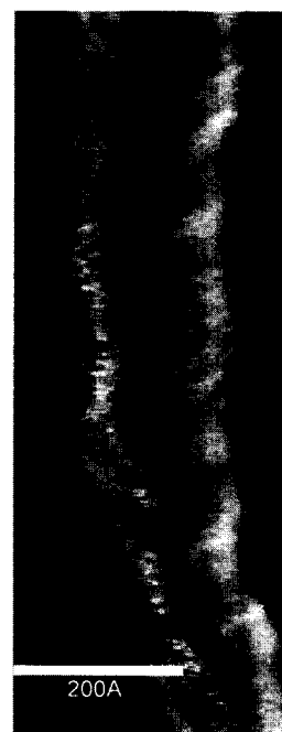
Fig. 11 STM image of two PmPV-coated SWNTs lying on HOPG substrate. The ordered coating can be seen in the tube on the right. There are two individual tubes on the left, separating at the bottom. (©ACS, 2002.)
