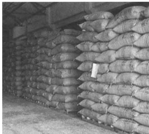
Fig.D.17: Platform of wooden planks used in godowns for storage of goods.
