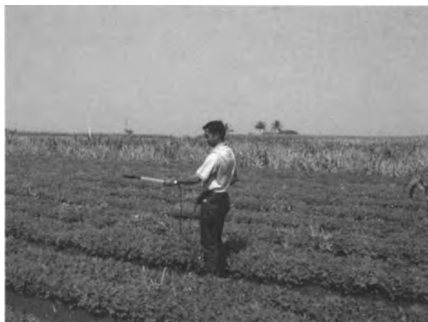
Fig.L.7: Plant canopy analyzer being used in groundnut field for estimating leaf area index.
