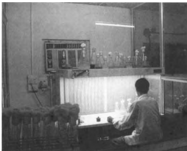
Fig.1.4: Inoculation of microbial cultures being done under aseptic conditions.
