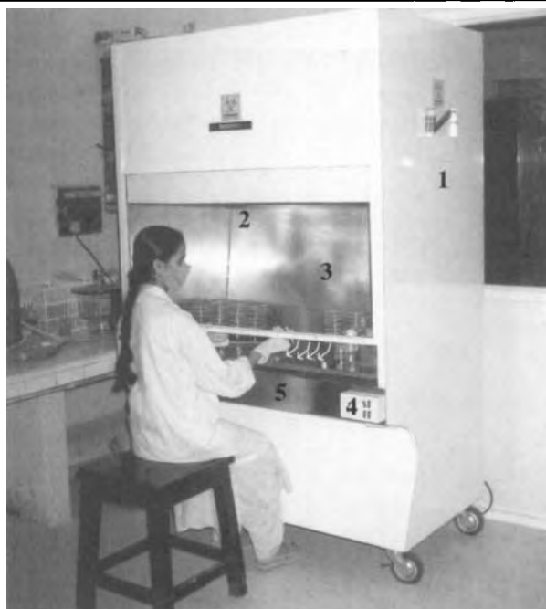
Fig.L.2: A laminar air flow cabinet. 1. Body of the equipment, 2. UV lamp, 3. Glass sliding window, 4. Switch board, and 5. Metal base (working platform). Arrows show the direction of airflow.
