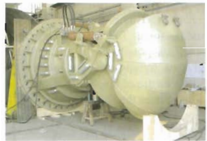
Waterjet with reversing bucket
