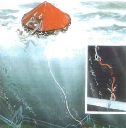
The last (weak) connecting line breaks and the survivors can climb into the inflated life raft.
