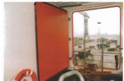
An opened side door, equipped with hydraulic cylinders for opening and closing. Also shown in the photo a lifebuoy and the pilot ladder.
