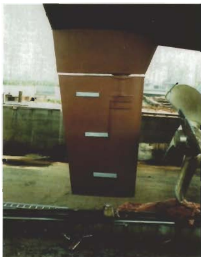
A spade rudder on a reef, freely suspended from the rudder dome
