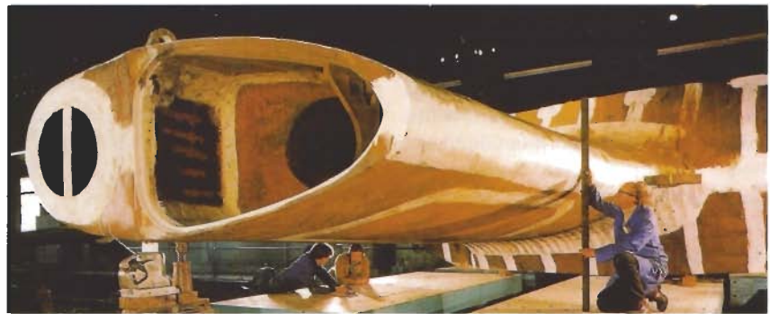
Cast steel rudderhorn
