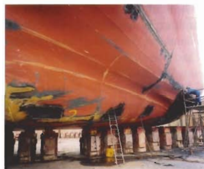
A view under the ship standing in a dock (normal dock block-arrangement)
