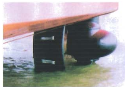
Sacrificial anodes on the propeller duct
