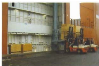
Fork lift places paper rolls on the ramp
