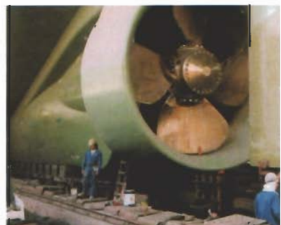
Controllable pitch propeller in a fixed nozzle.
