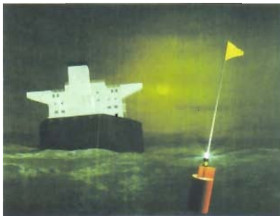
Buoy of an emergency towing system
