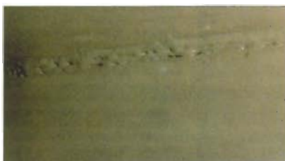
If holes or cracks are not welded properly this may cause problems with cleaning and pre-treatment. This in turn can cause small blisters, that cause de-tacking of the paint-layer.
