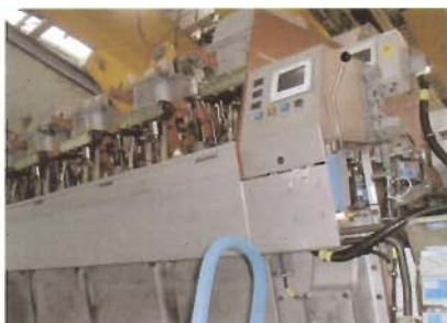
Engine control system fitted to an engine
