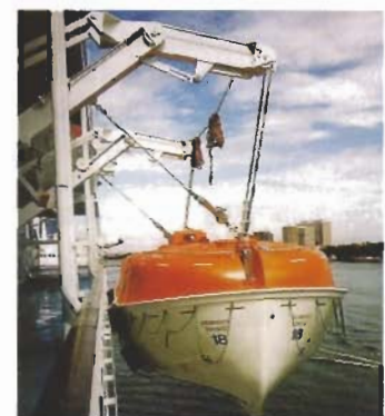
Life-boat tied with 19x7 steel wires
