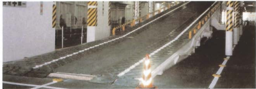
Hoistable car deck
