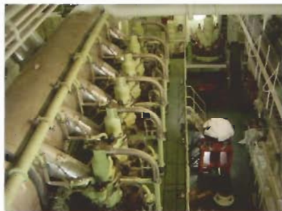
Low-speed engine (crosshead) two-stroke diesel engine, RPM range 80 to 120.
