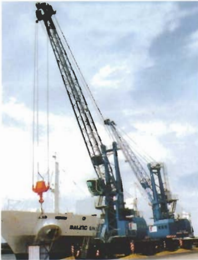
A mobile crane on pneumatic-tyres
