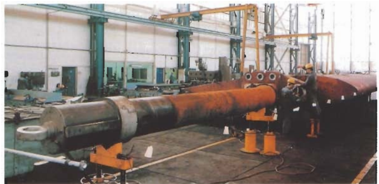
Alignment of rudder and stock in shop
