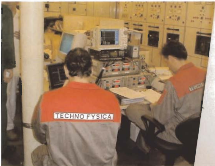
Engine-control room "Blue Star". During sea trials, specialists measure shaft RPM and torque to determine actual power, fuel consumption, etc.
