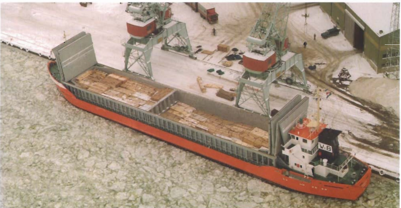
ship with opened (hydraulic) folding hatches. The ship is being loaded with timber parcels
