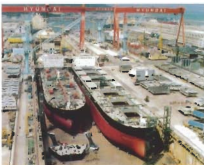
Construction in an excavated dock
