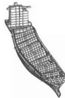
Waves coming in from portside at an angle, torsion
