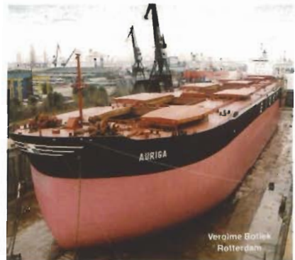
A ship with a small block-coefficient and a large midship section coefficient
