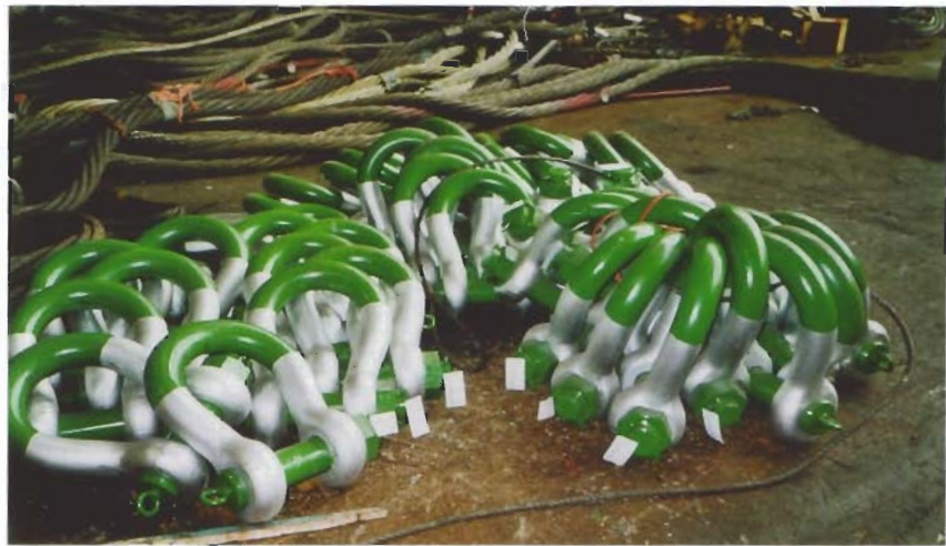
Heavy-duty bow shackles ready for testing
