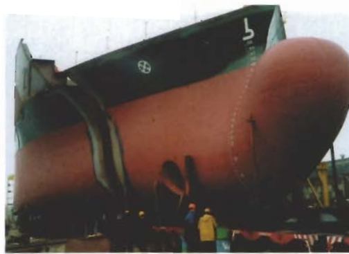
The fore part is being attached to the ship
