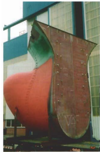
Forepeak, ready to be installed
