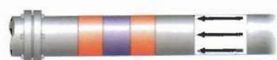
Pipe with colour code and arrows indicating the direction of the liquid flow
