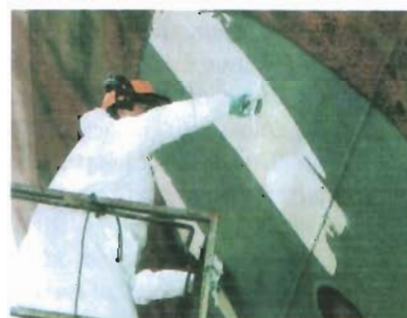
Special paint layer around the anode
