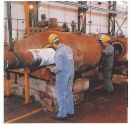
Fitting of pintles to new bushings
