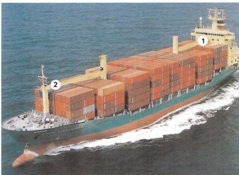
Midship deck cranes (SWL 40 tons and range 28 metres)
