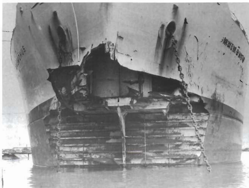
Damage caused by panting strain. Entire forepeak tank torn off. Ship size 100,000 t dead weight.
