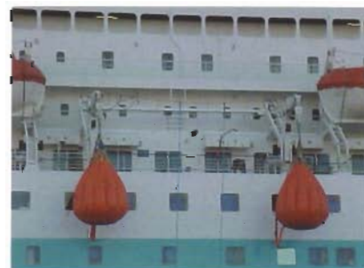
Testing lifeboat davits using water bags
