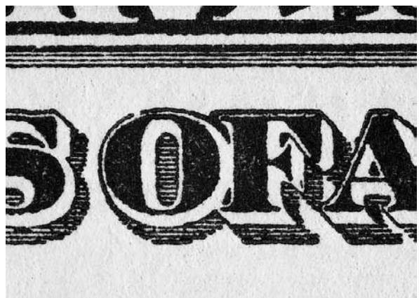
Figure 19 Counterfeit US $100 FRN: printed typographic.
