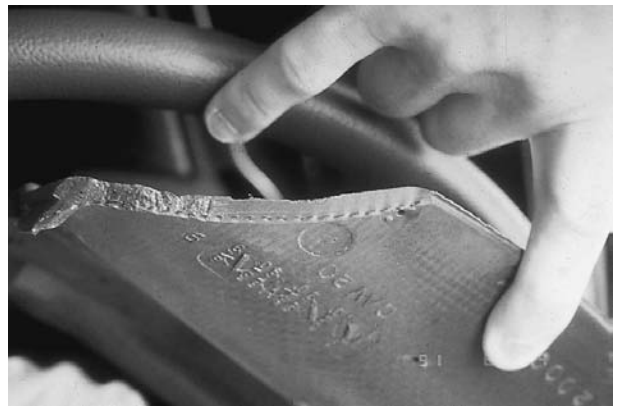
Figure 11 (A) The left lower corner of the module cover exhibited tearing from contact with the left side of the driver's face. (B) Close-up of the module cover reveals the presence of a torn area. There is also an area which indicates this piece was removed by a sharp implement.
