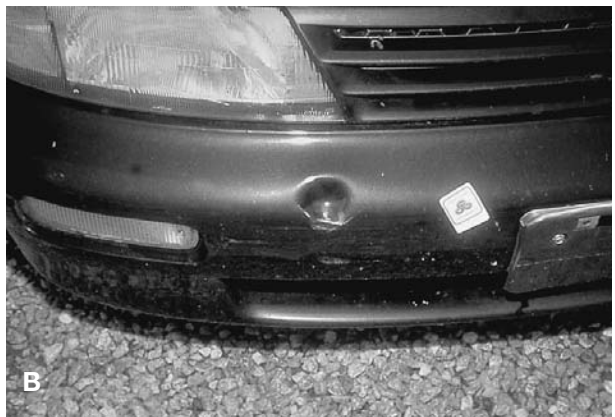
Figure 15(A) and (B) A 1995 Nissan Altima. The only damage to the vehicle is a 5 × 5 cm indentation in the front bumper from impact with the ball of a trailer hitch.
