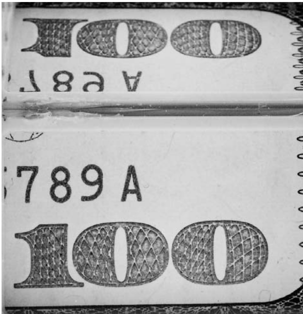
Figure 5 (see color plate 27) Green-to-black color shifting ink on genuine US banknote. Photographed using an angled mirror: green image (below) at normal; black (above) at an oblique angle.
