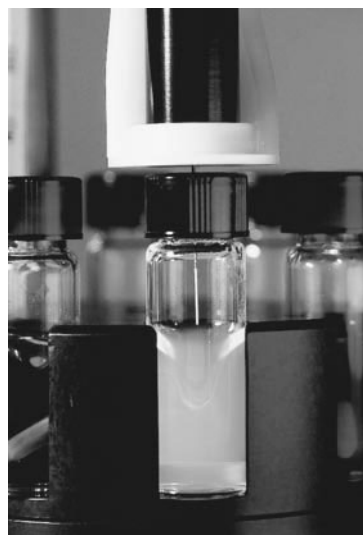
Figure 2 (see color plate 8) Photograph of a SPME fiber inserted into headspace of a sampling vial. (Courtesy R Mindrup, Supelco Inc.)
