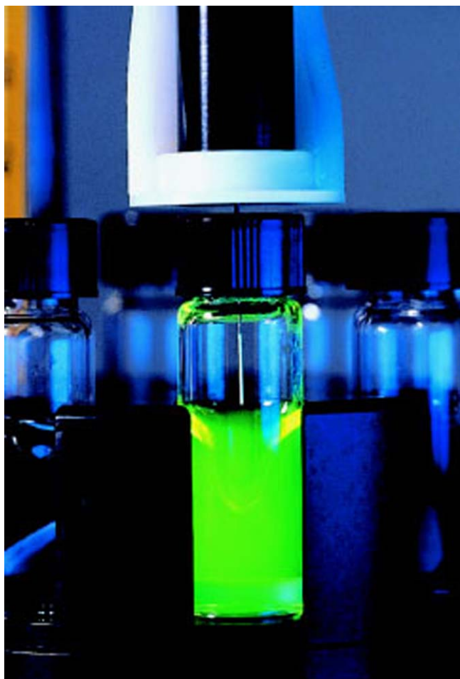
Plate 8 ANALYTICAL TECHNIQUES/Separation Techniques Photograph of a SPME fiber inserted into headspace of a sampling vial. (Courtesy R Mindrup, Supelco Inc.)
