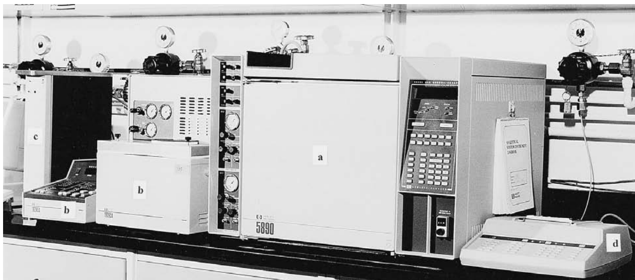
Figure 4 HS-GC instrument system with GC instrument (a), HS analyzer (b), A-D converter (c), and optional integrator with printout (d).
