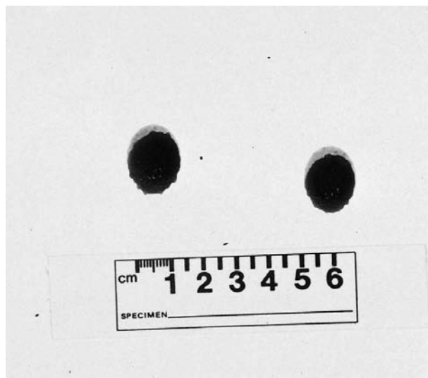
Figure 3 The shape of a drop of blood that impacted the target surface from an angle of 50°.
