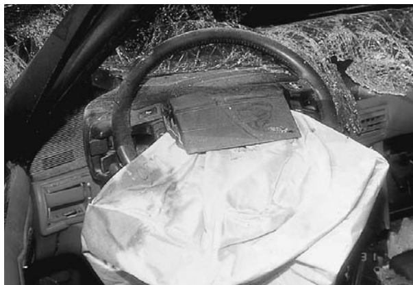
Figure 2 The injury-producing components of the air bag system are the air bag and the module cover which overlies it.
