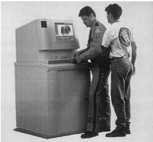
Figure 6 Livescan station for electronic recording of fingerprints. Courtesy Printrak International.
