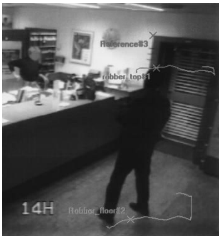
Figure 8 Measuring the height of a robber by reverse projection from a digitized surveillance video recording. The height was calculated from an image sequence and the path of the robbers movement in the bank have been tracked.
