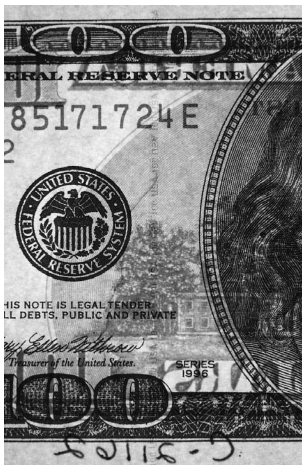
Figure 9 Counterfeit US $100 FRN security thread: simulated by offset printing.
