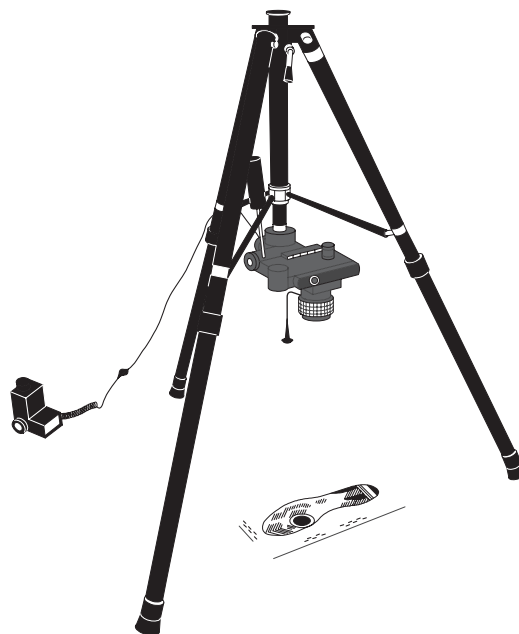
Figure 1 To take examination-quality photographs, a camera on a tripod should be positioned directly over the impression. A scale should be placed alongside the impression. A flash unit and long flash extension cord will allow the proper use of oblique light during exposure.
