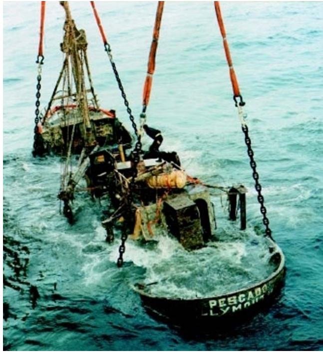
Plate 19 ENGINEERING The fishing vessel Pescado was recovered from the sea off the south west coast of England to assist the Marine Accident Investigation Branch enquiry into the loss of the vessel and crew. Marine Accident Report 1/98 (1998), London DETR. (Copyright–The Chief Constable, Devon and Cornwall Constabulary.)
