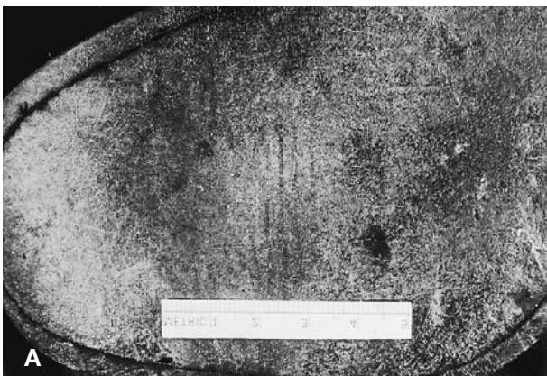
Figure 10 (A) Examination of leather-soled shoes may reveal the presence of a pedal imprint. (B) The shoe reflects an imprint from the vehicle's brake pedal and indicates that the wearer of the shoe was, in fact, the driver.
