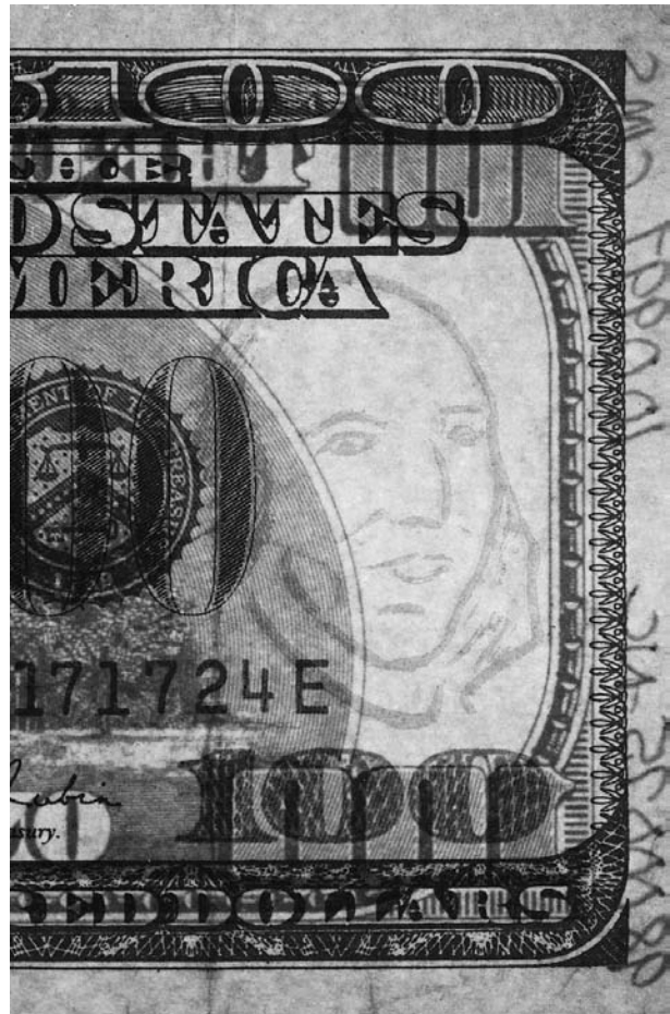
Figure 7 Counterfeit US $100 FRN watermark: simulated by offset printing.
