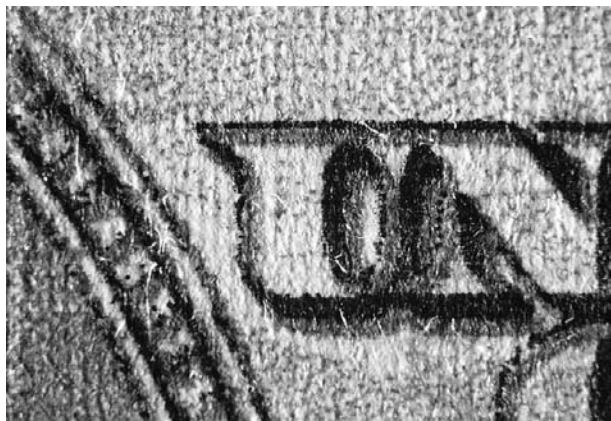
Figure 25 (see color plate 33) Counterfeit US $100 FRN: inkjet full color copier/printer.
