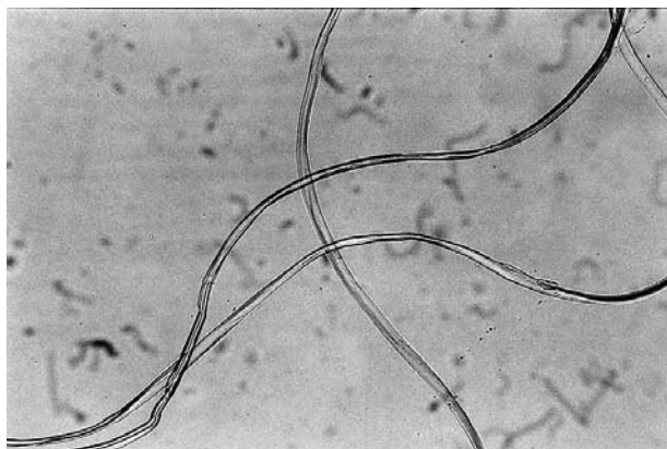
Figure 2 Silk fiber (magnification 90×).
