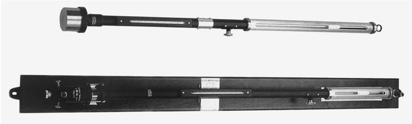
A Kew barometer, measuring the ordinary temperature range and calibrated in millibars and millimeters of mercury. (Casella CEL Ltd.)
